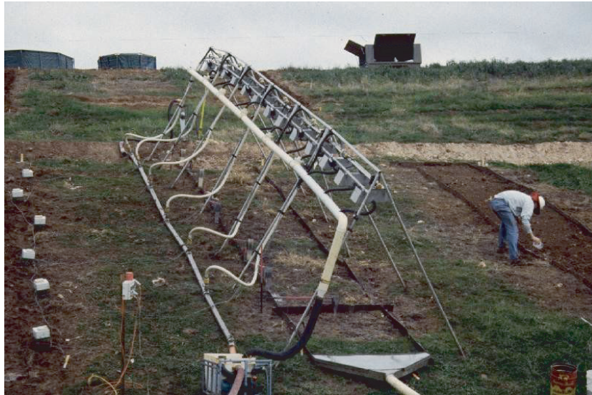
Fig. 1. 6-module RFS, showing modular design, catch troughs, pump, and water delivery and return systems, with control boxes visible at the left of the picture.
