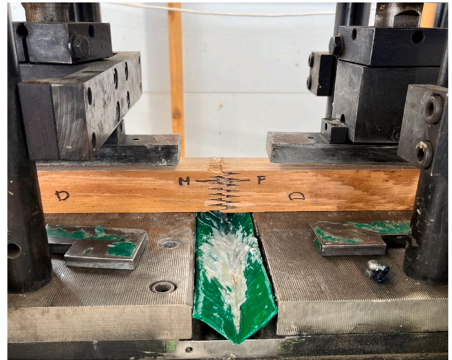
Fig. 2. Modified Festo Jointing Machine Combination FKV used in Stage 1 to press finger joints.
