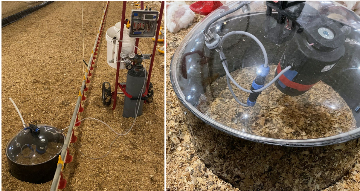
Figure 28. Flux chamber along with sweep-air cylinder, flow regulator and data logger used to measure ammonia emissions from litter.
