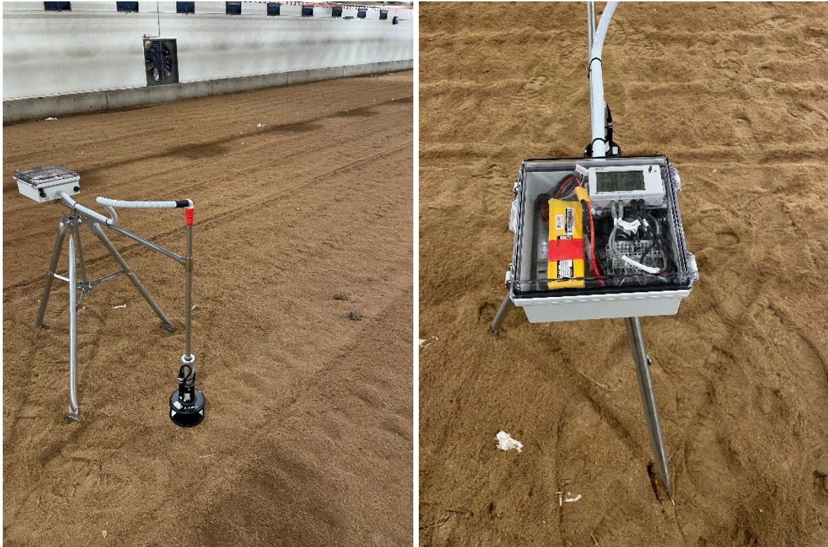
Figure 57. Ultrasonic sensor and logger used to measure airspeed close to the litter surface during side-vent ventilation.
