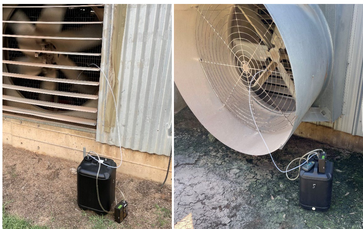
Figure 43. Odour sampling configuration and equipment used.
