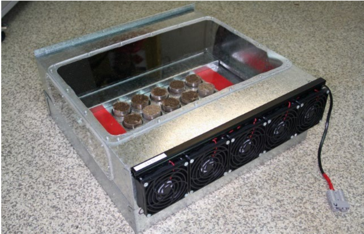
Figure 53. Wind chamber used to provide constant airspeed (0.5, 1.0, 1.5 or 2.0 m/s) at the surface of litter samples.
