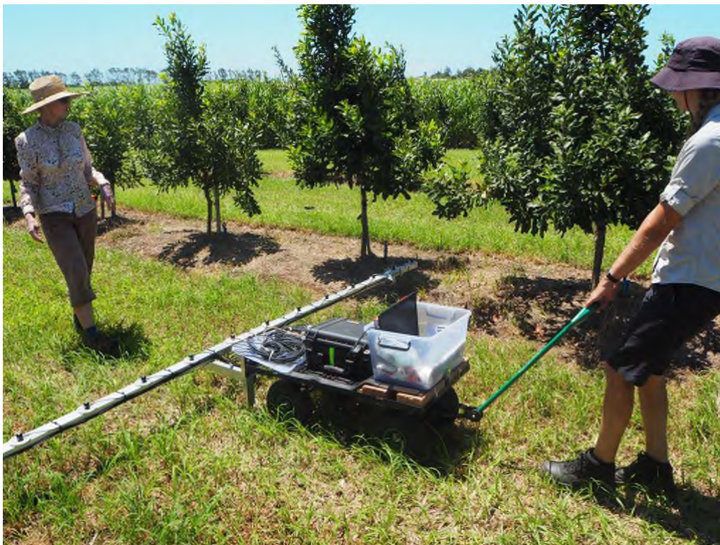
Figure 1. Purpose built light trolley measuring total light interception in the macadamia Planting Systems Trial.
