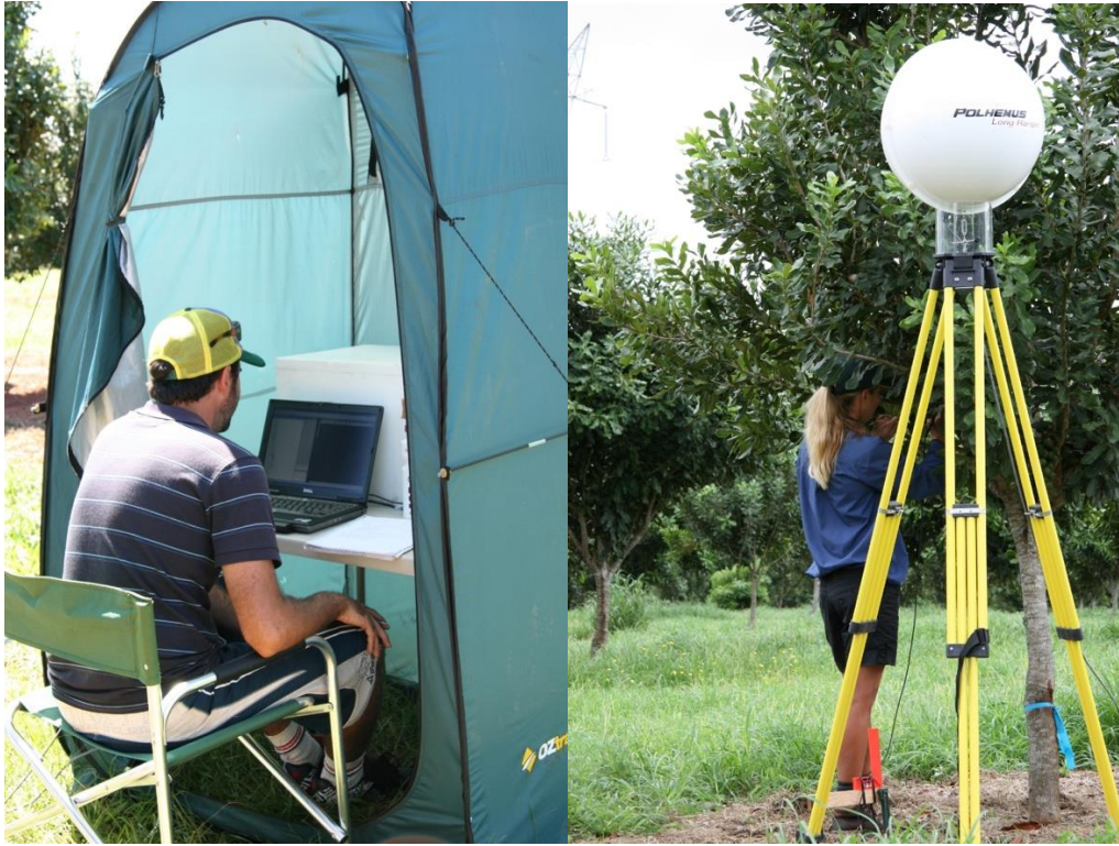
Figure 1. Digitising a macadamia using the Polhemus Fastrak
