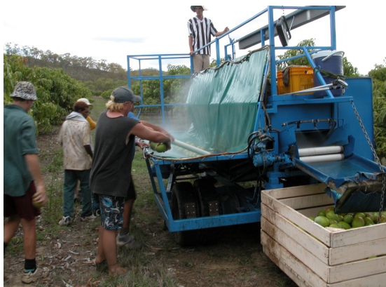
FIGURE 1 - Australian mango harvest-aid used in field uses a detergent covered tarpaulin to catch fruit and cover them in a protective layer of detergent to prevent sap-burn.
