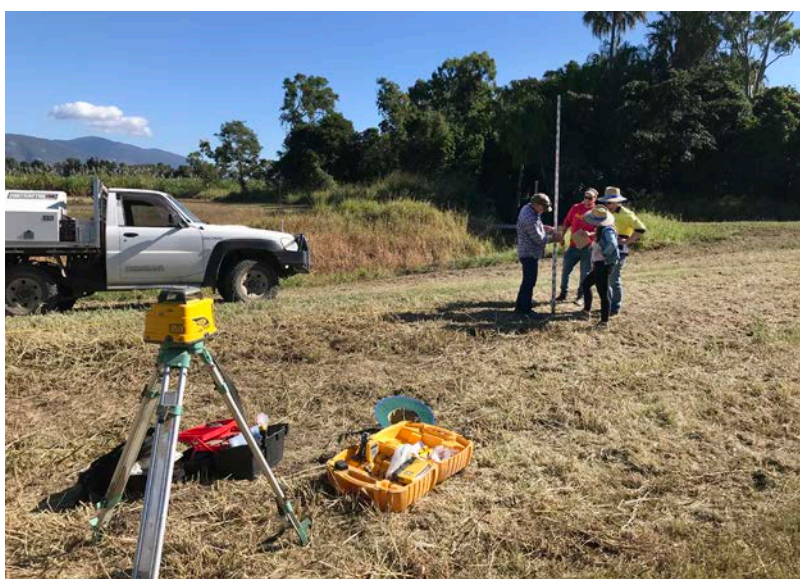
Figure 3.1 Taking levels during the site investigation to determine if slope is sufficient.
