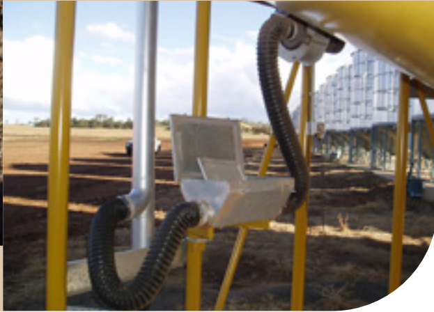
Phosphine fumigation using the tablet in trays place in the silo headspace
