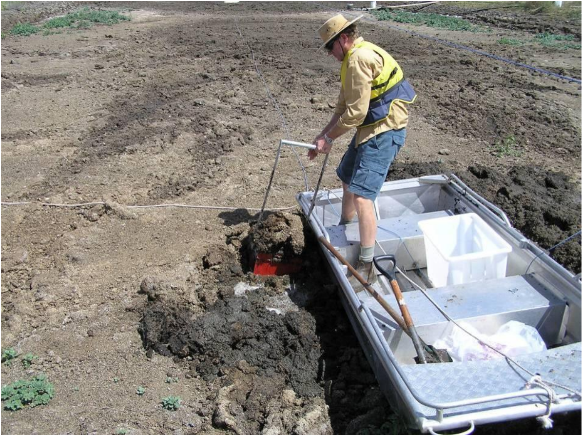
Figure 18: Crust sample collection on the highly loaded pond at the Dalby piggery.
