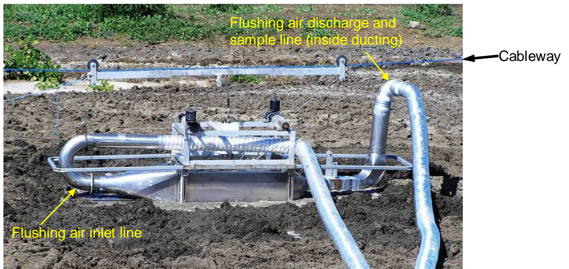
Figure 21: DPI&F wind tunnel in use on highly loaded pond
