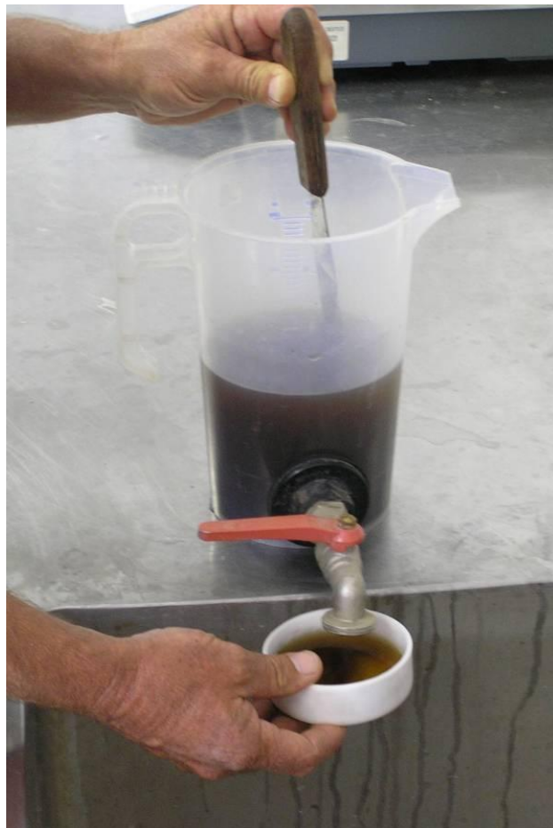
Figure 15: A 2 L capacity jug was used in the laboratory to decant effluent into the crucibles used for TS and VS analyses during stage 2.
