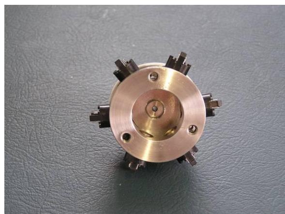
(d) Prototype 2 sensing chamber showing the six MOS sensors and minimal internal volume of 23.5 mL (internal view)
