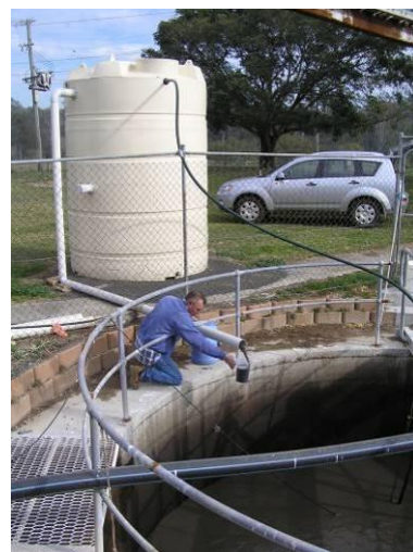
Figure 29: Collecting settling tank outlet sample from overflow pipe.
