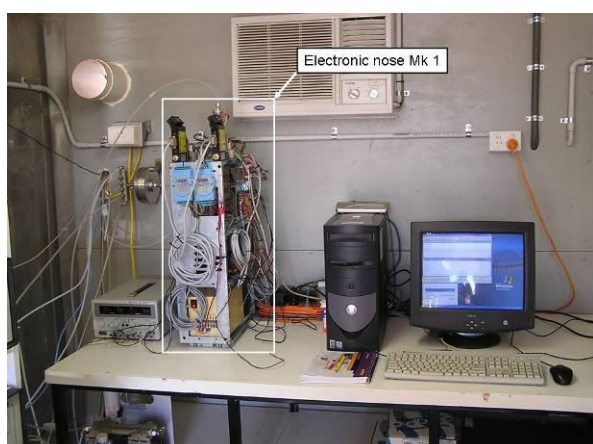
(a) Gas sensor array system comprising 24 MOS sensors
