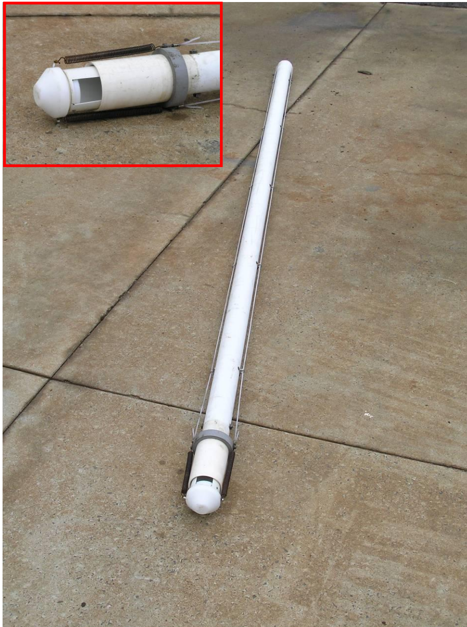
Figure 17: DPI&F pond sludge sampler with the sludge collection slot partly exposed.
