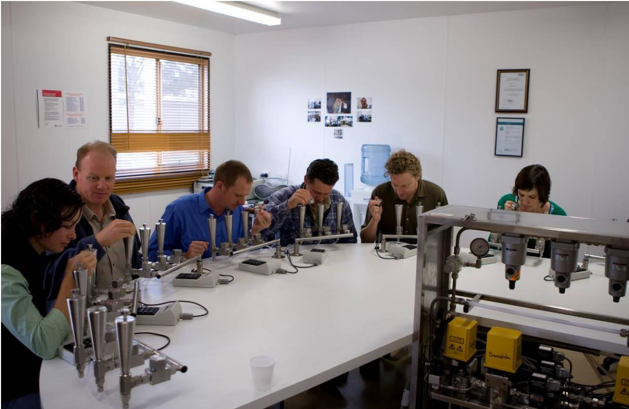
Figure 24: The DPI&F olfactometer in operation showing panellists sniffing at ports.
