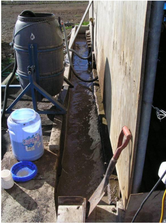
Figure 7: 200 L tipping drum during pumped sampling from the shed 5 effluent sump.
