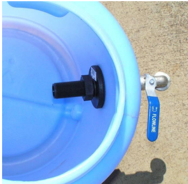
Figure 9: 25 litre sampling drum used for temporary storage, transport and sub-sampling of composite effluent samples.
