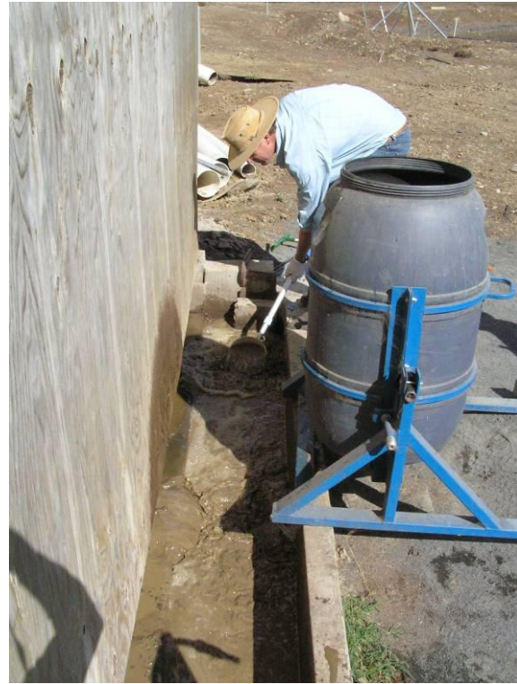
Figure 8: 200 L tipping drum during manual bucket sampling from the shed 5 effluent drain.
