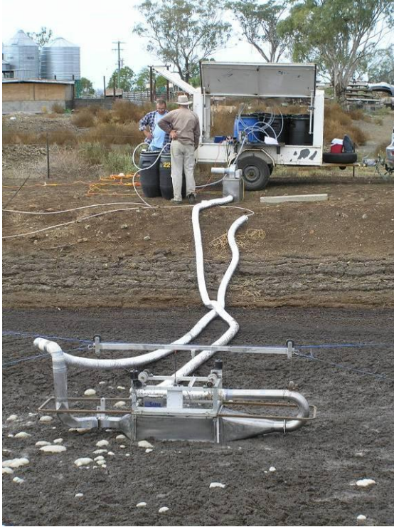
Figure 22: Odour sampling from wind tunnel suspended above primary pond crust.
