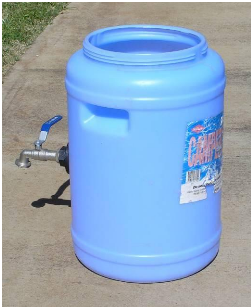
Figure 9: 25 litre sampling drum used for temporary storage, transport and sub-sampling of composite effluent samples.
