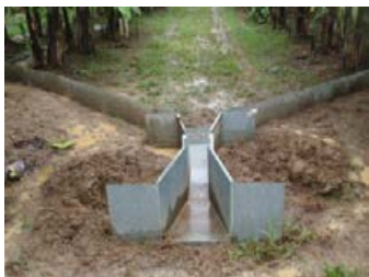
Flumes capture surface run-off and help researchers assess the level of sediment and nutrient movement after rainfall.
