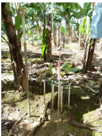
Devices such as lysimeters can be buried to measure nutrient losses through leaching.
