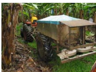
Fertilisers must be applied to the row only, when using a fertiliser spreader. This places the fertiliser where it is required and reduces the total amount applied.
