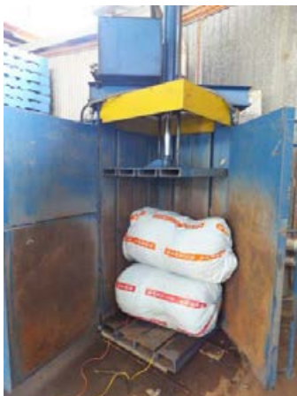
Presses compress waste bunch covers to reduce their total volume.
