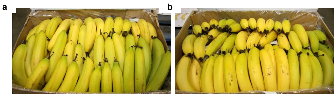
Figure 7.5 - Condition of bananas packed in a standard (a) or stronger grade (b) carton following transport and ripening.
