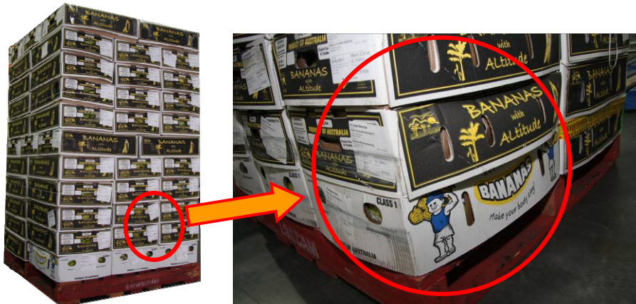
Figure 6.3 - Carton condition after ripening, showing the difference in carton integrity between standard (black) cartons and the stronger grade (white) cartons on the base of each pallet.
