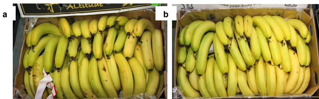
Figure 6.4 - Condition of bananas packed in a standard (a) or stronger grade (b) carton following transport and ripening. Damage incidence and severity was similar for both carton types
