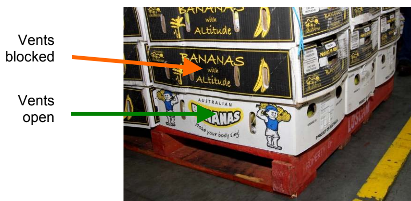
Figure 7.4 - Carton condition after ripening, showing the difference in carton integrity between standard (black) cartons and the stronger grade (white) cartons on the base of each pallet.
