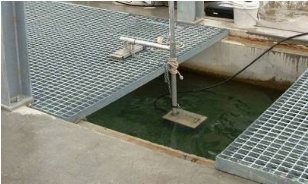
Figure 2. Location of the DIDSON system in the fishway exit channel at Lock 10.
