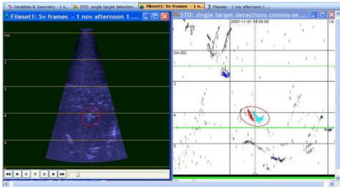
Figure 5. Echogram showing a school of fish detected swimming out of the fishway exit channel at Lock 10 fishway by the DIDSON system. The window on the left shows the acoustic system image the window on the right shows the single targets and two fish tracks (red and blue shapes around targets).
