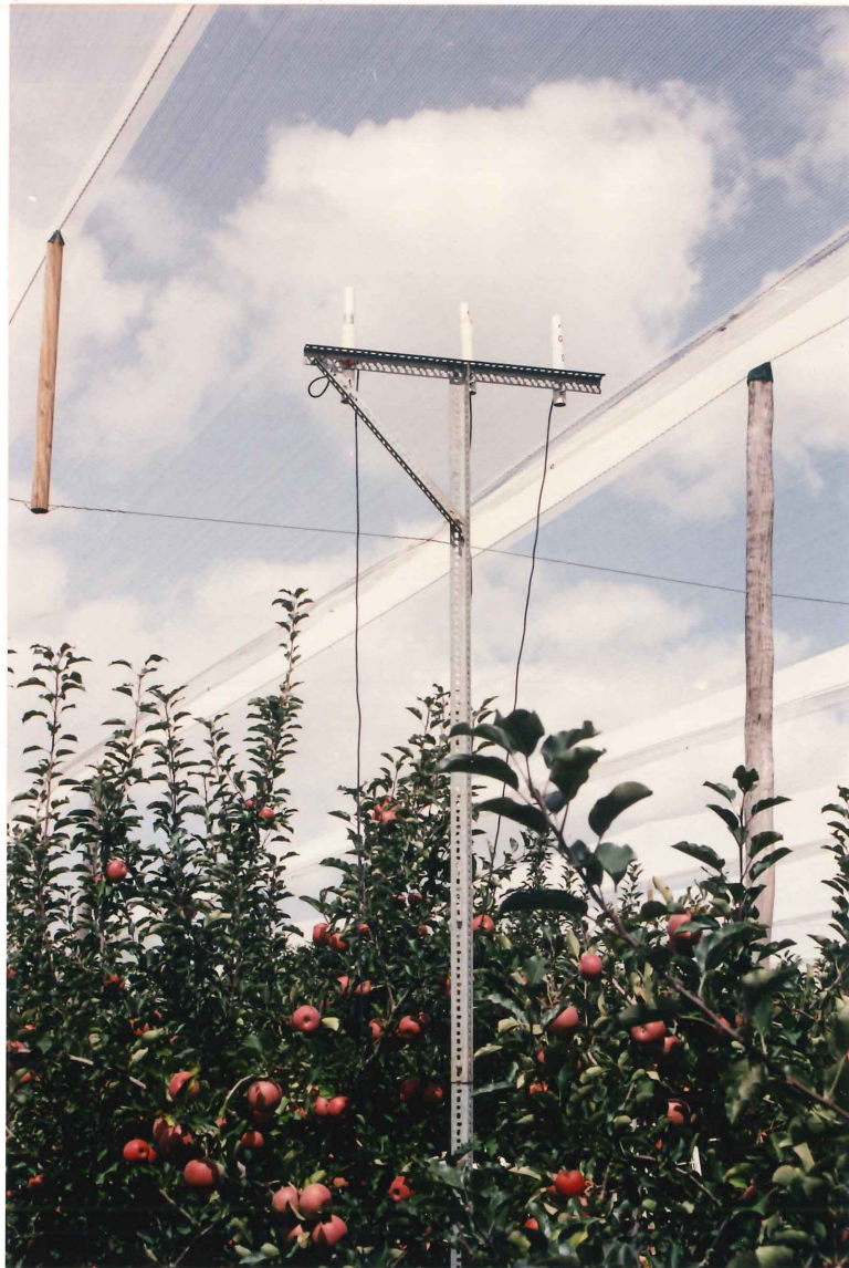
Plate 3. White Hailgard netting above Fuji trees at Site 3 (Granite Belt, Qld). This net type was also used at Site 4. Three lightmeters are visible in the centre of the photograph, and are measuring the light penetration (PAR) through the hail netting.
