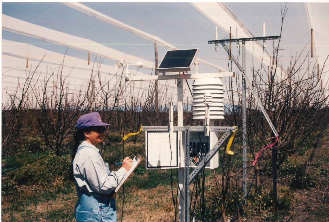
Plate 3. An automatic weather station under white hail netting on the Granite Belt, Qld. The data logger is housed in the white box; above this is a Stevenson screen that encloses a temperature sensor and a humidity sensor. Also visible are an anemometer, solar panel, two temperature sensors in the foreground (one in a small screen and one exposed), and three lightmeters above the dormant Red Fuji trees.
