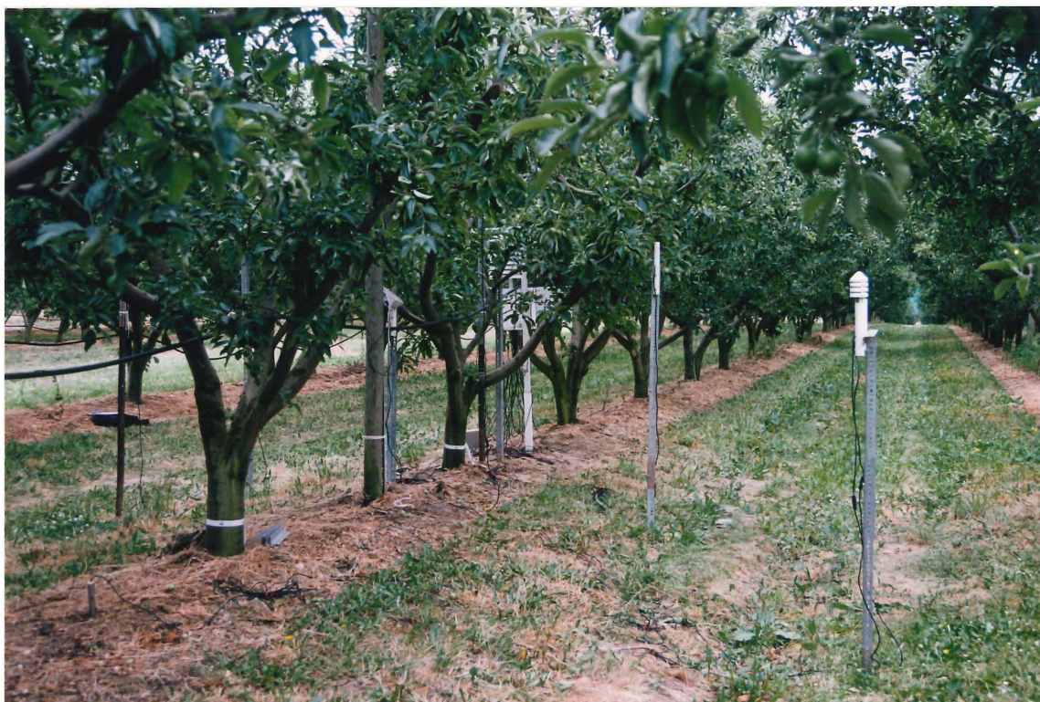
Plate 2. Trial site at Drouin, Vic. The automatic weather station is positioned within the tree row, midway between two Granny Smith trees. A temperature sensor in a miniscreen (far right) and a lightmeter are visible in the alleyway.
