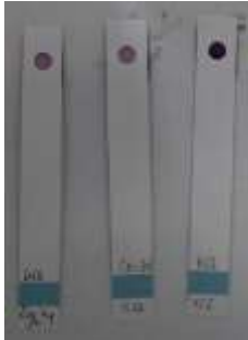
Figure 336 Accuvin strips showing development of dark purple colour in response to presence of glucose in YCS leaf sample
