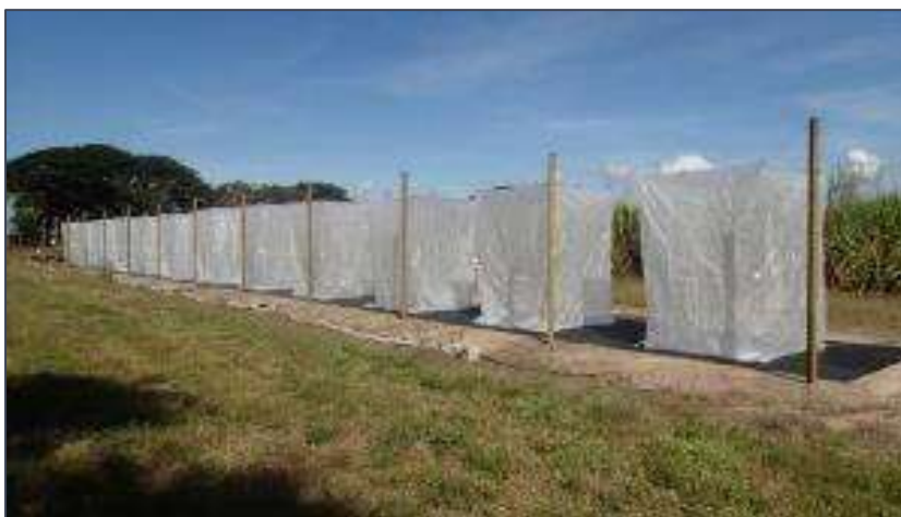
Figure 211 Insect exclusion experiment. Twelve insect tents on site at the SRA Burdekin station.
