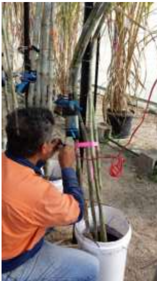
Figure 181 Sap flow meter being attached to a cane stalk in the shade house
