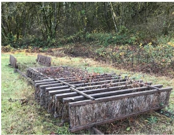
Figure 23. Weathering of wood in I-Beam durability trial in OSU field site (L) and on wooden cladding in Switzerland (R)
