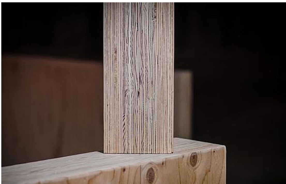
Figure 12. Section of veneer-based mass panel. (Source – Portland Business Journal, Matt Swain Photography)
