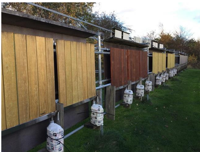
Figure 59. Weathering and leaching assessments at DTI, Denmark
