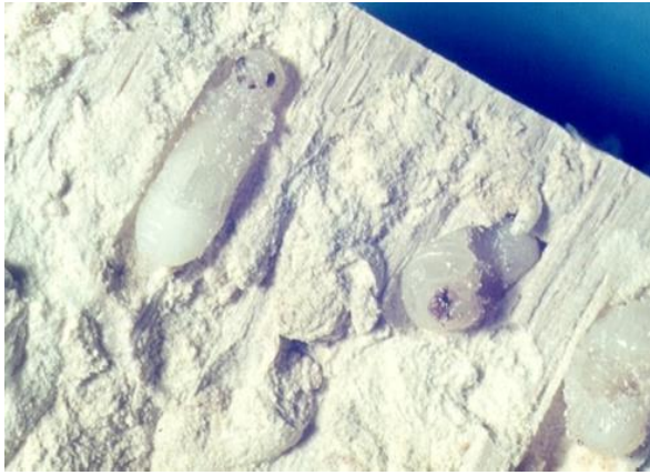
Figure 22. Lyctid beetle (borer) damage to wood including larvae and frass. (Source – Doug Howick (L) and Ted Stubbersfield (R)).
