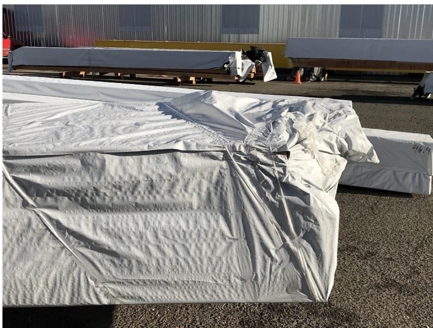
Figure 48. Plastic wrapped glulam in the USA.
