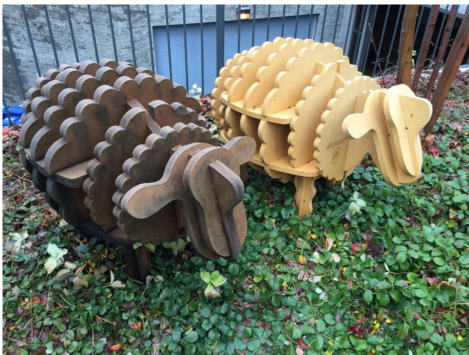
Figure 41. Tricoya treated MDF in sheep on right showing improved exterior performance after outdoor exposure at the University of British Columbia.
