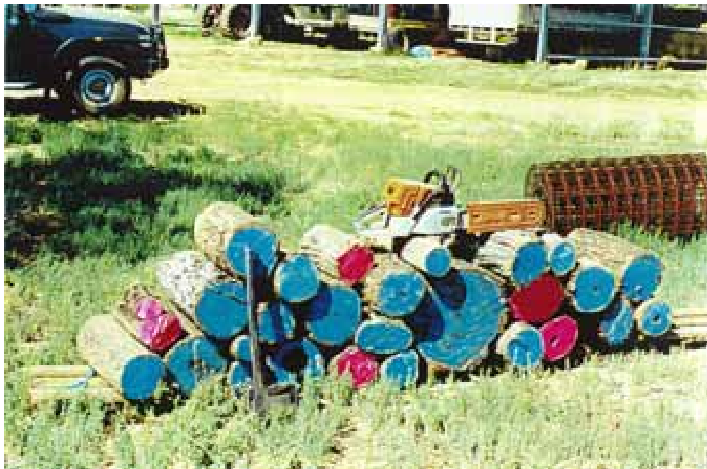
Figure 3.2 Billets were end-painted after cutting to limit drying degrade prior to testing
