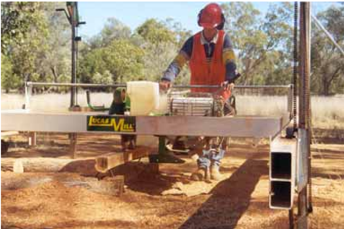
Figure 4.5 Sawing boards from a small mulga sawlog
