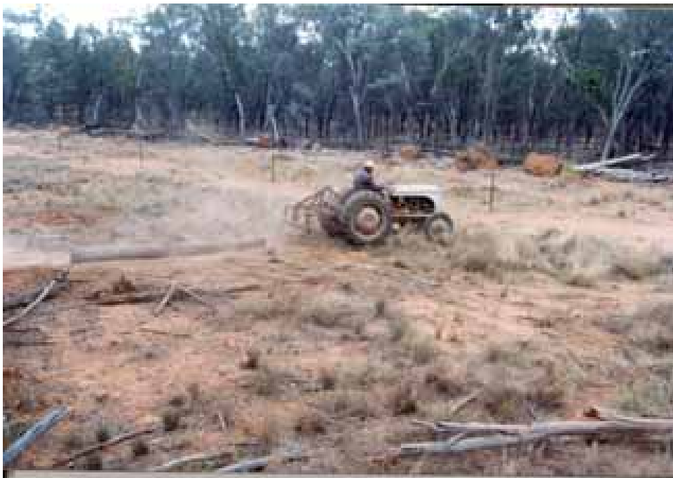
Figure 4.3 Snigging a mulga sawlog to a loading zone
