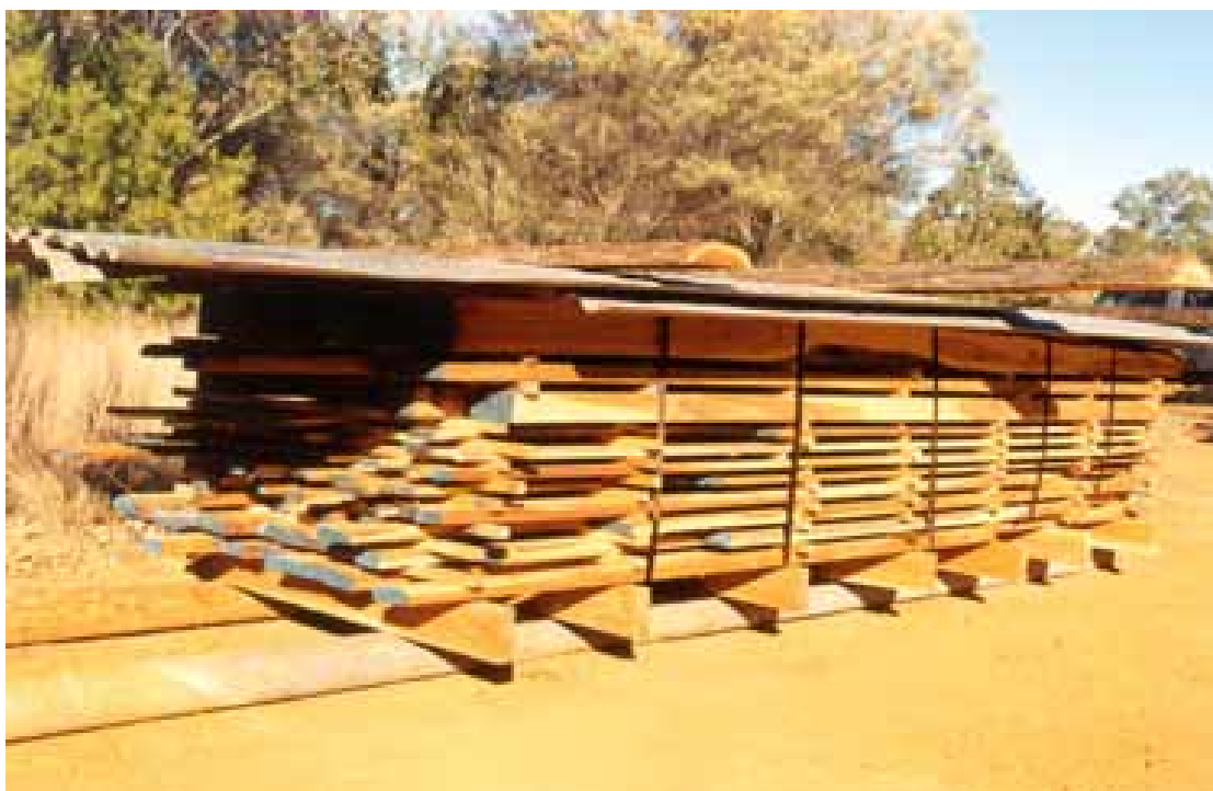
Figure 5.1 Unprotected air-drying of mulga on Maryvale Station
