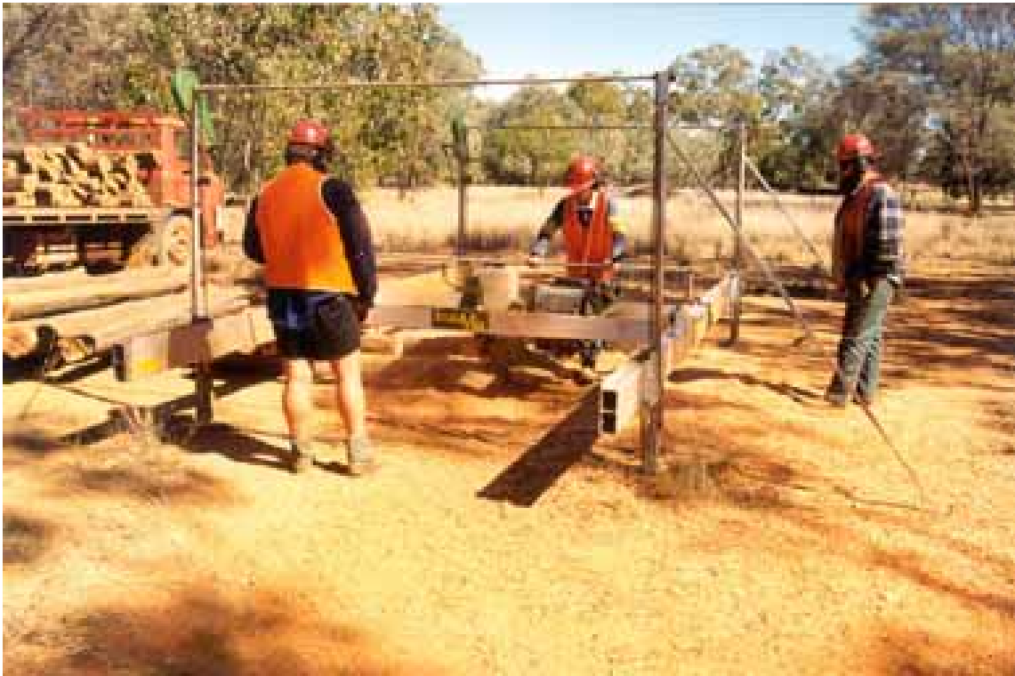
Figure 4.4 The Lucas 8" portable sawmill in action at Maryvale Station
