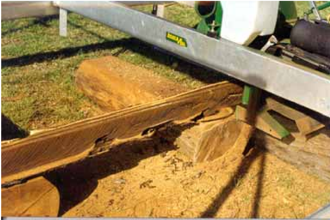
Figure 6.10 Decay and heart associated defects in a gidgee board
