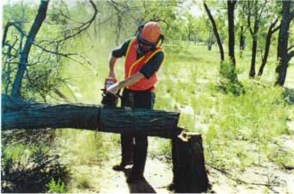
Figure 3.1 Cutting a billet from a tree for wood property testing
