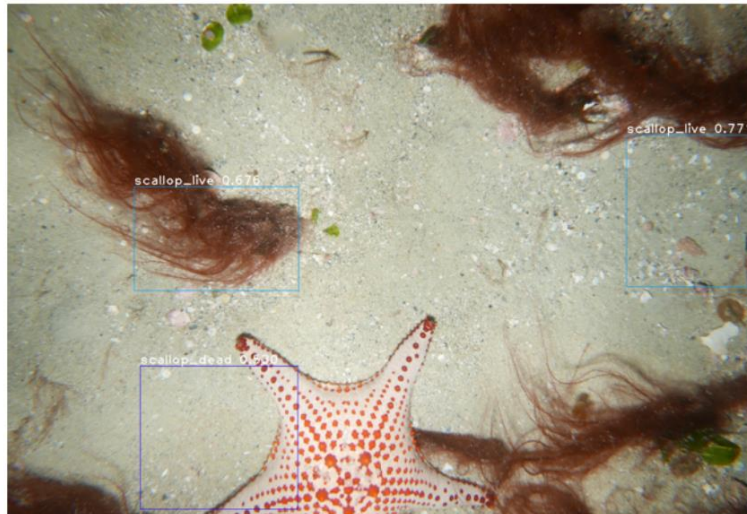
Figure 15. Example where objects were detected by autclassification, when clearly no scallop exists
