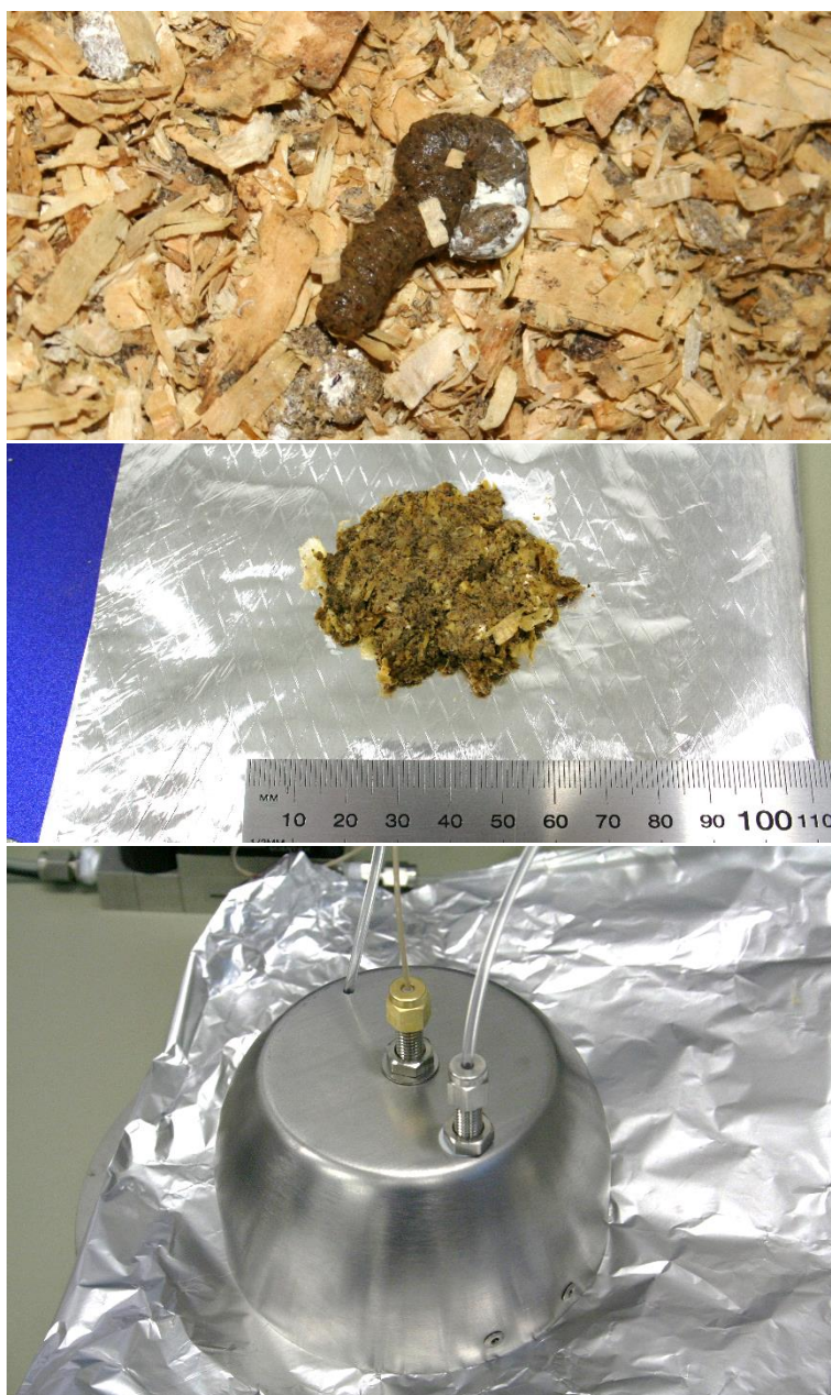
Figure 88. Odorant collection from fresh excreta: ( top ) fresh excreta as sampled from the litter surface; ( middle ) excreta levelled and measured to determine surface area; and ( bottom ) flux chamber sampling odorants for PTR-TofMS analysis
