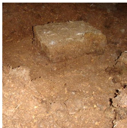
Figure A. 7. Cake collected to assess moisture holding capacity and drying rate
