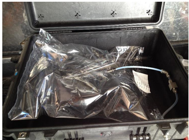
Figure 80. Collection of odorant samples: VOC samples collected into sorbent tubes (left); and VSC and odour (for olfactometry) samples collected into Nalophan bags (right)
