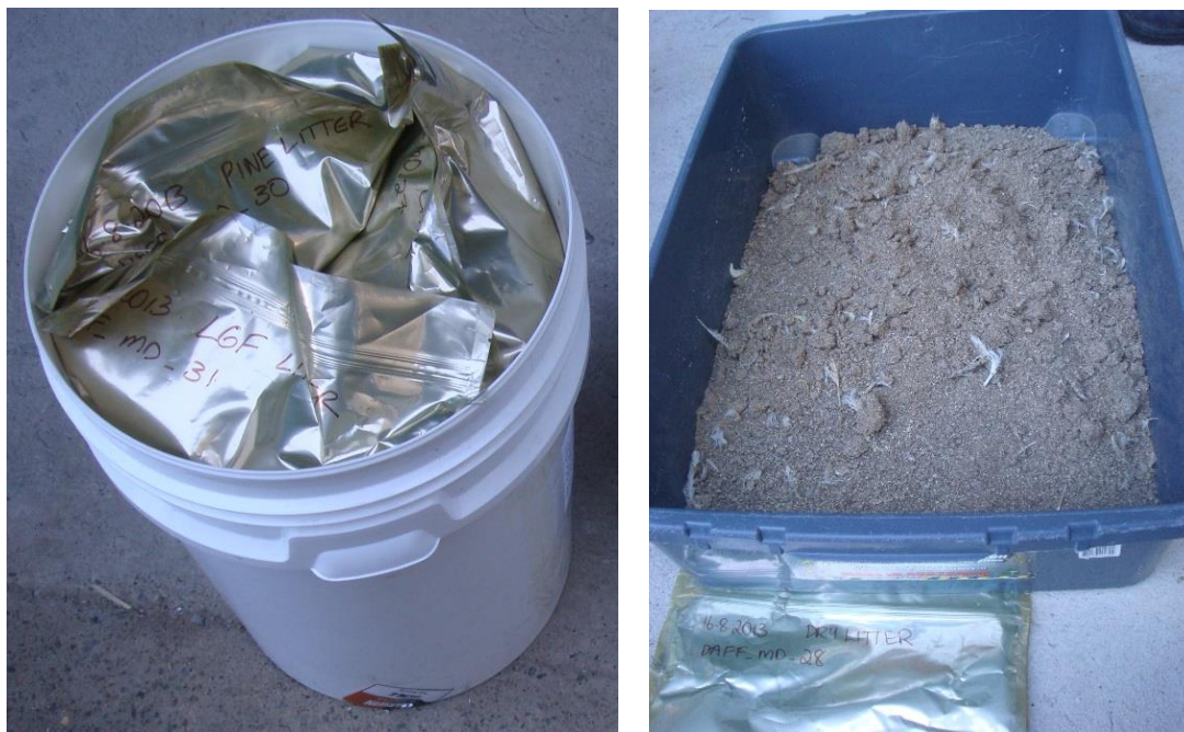
Figure 77. Litter samples were sealed in plastic bags for transport to the laboratory ( left ) and spread in a tray ready for odorant collection using a flux hood
