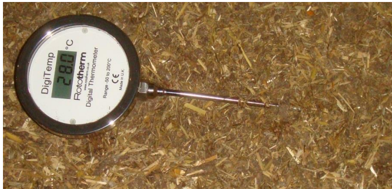
Figure 54. Using a thermometer to measure litter temperature
