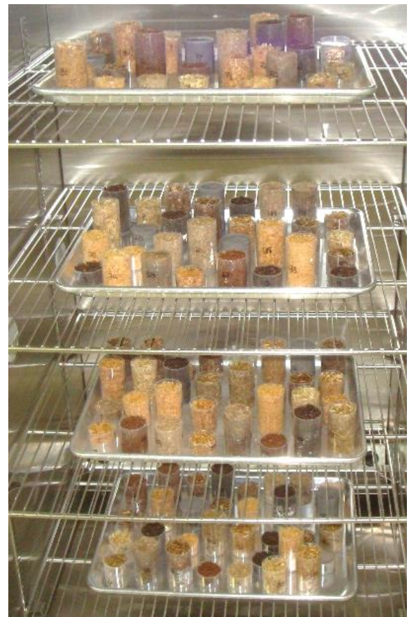
Figure A. 10. Sample trays in the temperature and humidity controlled cabinet
