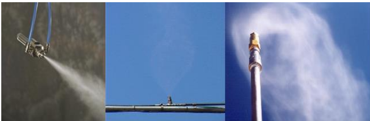
Figure 22 Types of spray nozzles typically used in odour control applications
