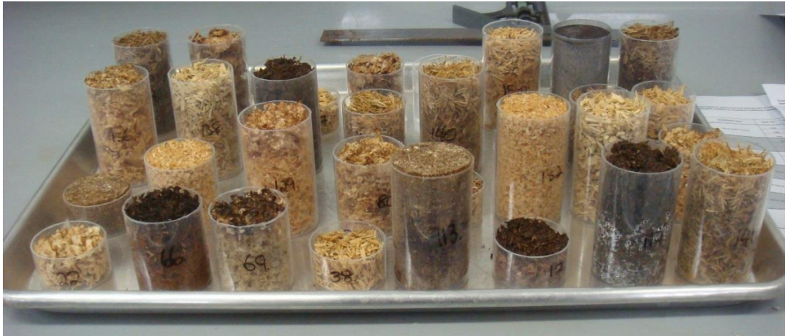
Figure A. 9. Samples in jars prepared on trays for drying rate trial
