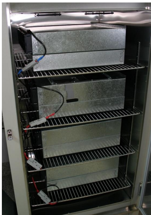
Figure 29. Custom wind tunnels in the temperature and humidity controlled cabinet
