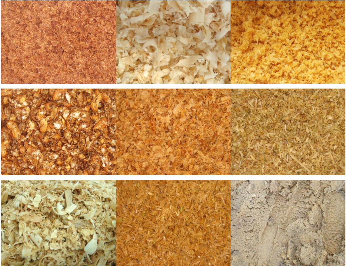
Figure A. 5. Selected bedding materials acquired for testing: Top, L–R: hardwood sawdust, pine shavings, pine sawdust. Middle L–R: peanut shells, mixed softwood shavings, lemongrass straw. Bottom L–R: Cypress sawdust, rice hulls, sand.
