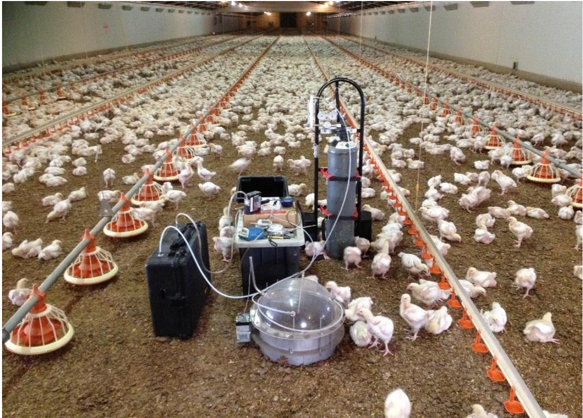
Figure 79. Using a flux hood to collect odorant samples from the litter surface in a meat chicken shed
