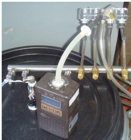
Figure 80. Collection of odorant samples: VOC samples collected into sorbent tubes (left); and VSC and odour (for olfactometry) samples collected into Nalophan bags (right)
