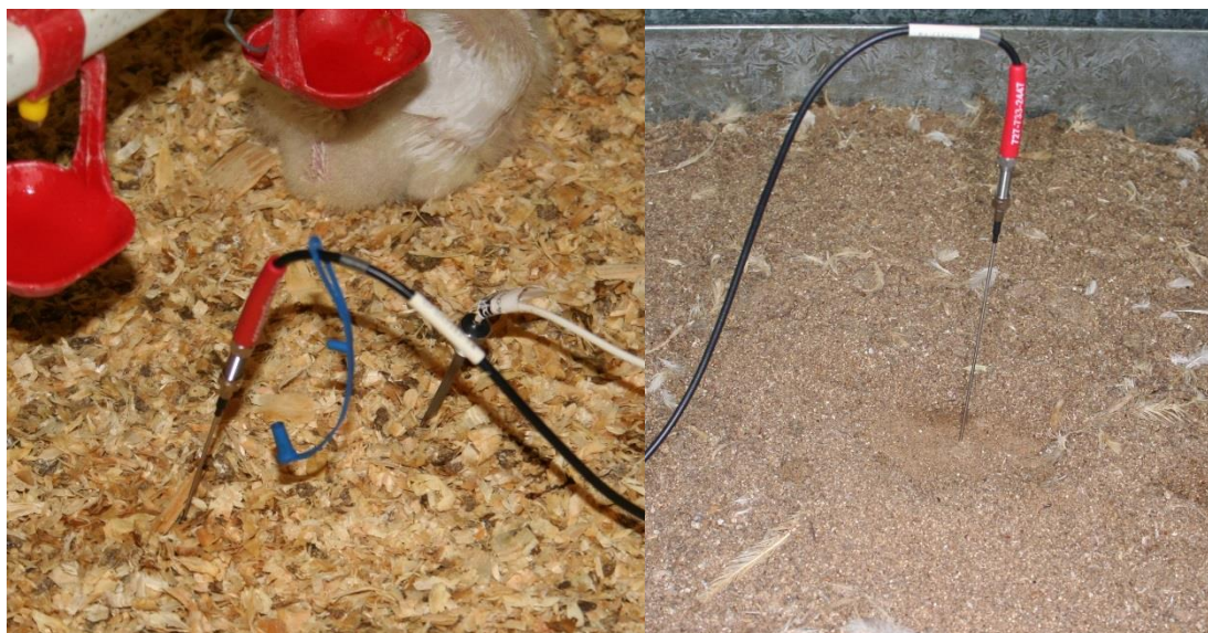
Figure 56. Oxygen concentration measurement using a probe and accompanying temperature sensor in friable litter ( left ) and caked litter ( right )
