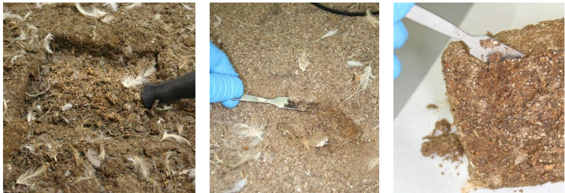
Figure 52. Collecting litter samples from sections of the litter profile: Friable under-cake material ( left ); bottom of the cake ( right ) from the sample in Figure 48; and the surface of the cake ( middle ) from the sample in Figure 49
