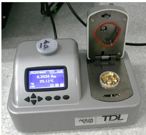
Figure 57. Water activity meter showing the temperature controlled sample chamber (right) and a sample of friable litter)
