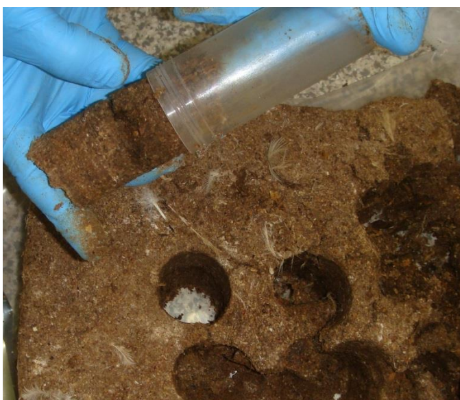
Figure A. 8. Cutting cake to fit the sample jars
