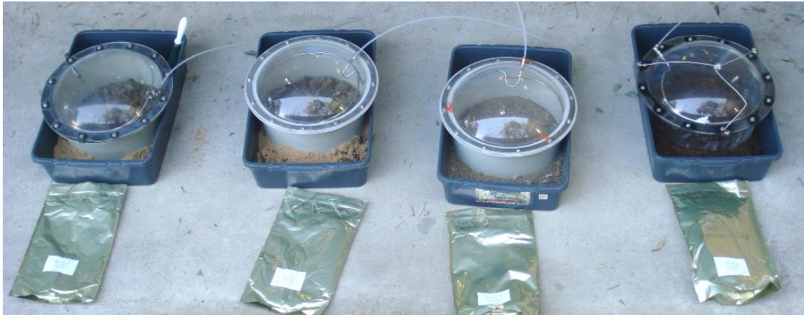
Figure 78. Flux hoods used to measure odorant emissions from litter samples at the laboratory
