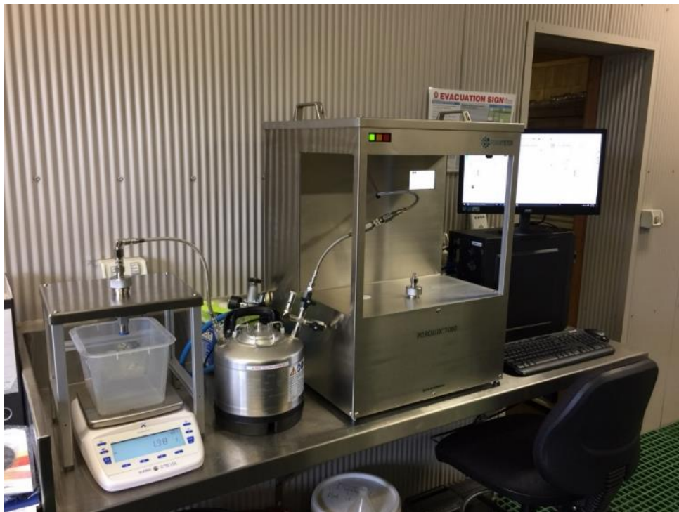
Figure 123. Permeability module in the wood value platform: Porolux 1000 porometer. Permeability was calculated from Booker's equation (Booker, 1977):
