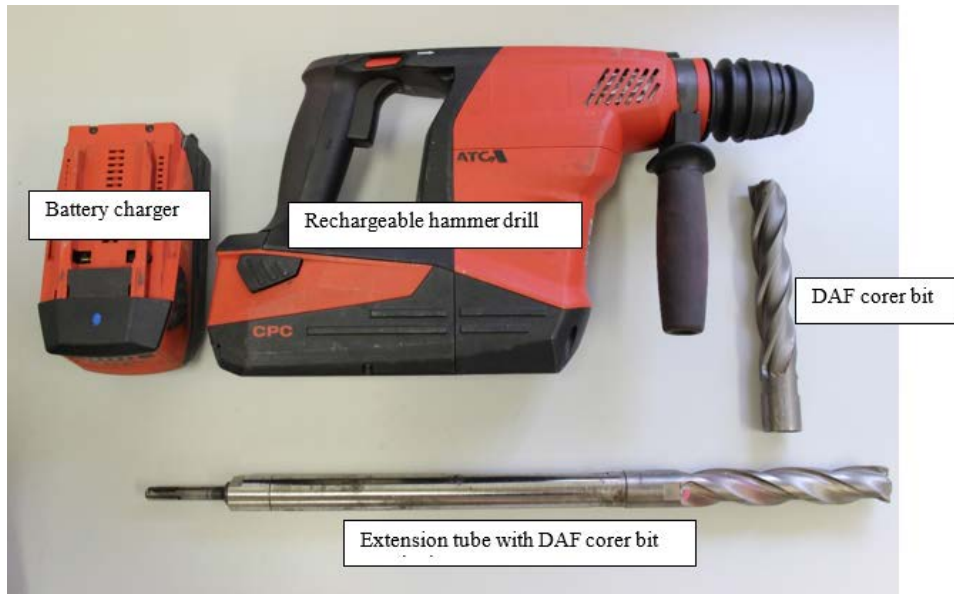
Figure 112. DAF tree corer system comprising a rechargeable hammer drill (top) and extension bar and corer bits (bottom).
