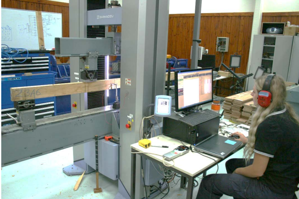
Figure 11. Static bending testing for MOE from a sub-sample cut from a 3.9 m board.
