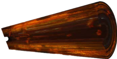
Figure 93. Volume visualisation of reconstructed billet using Drishti. The internal knots are clearly visible.
