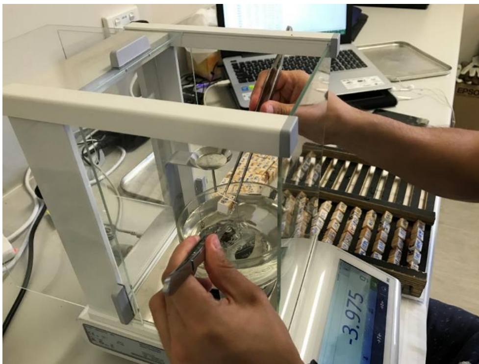
Figure 116. Wood segment density determined in accordance with Australian Standards.
