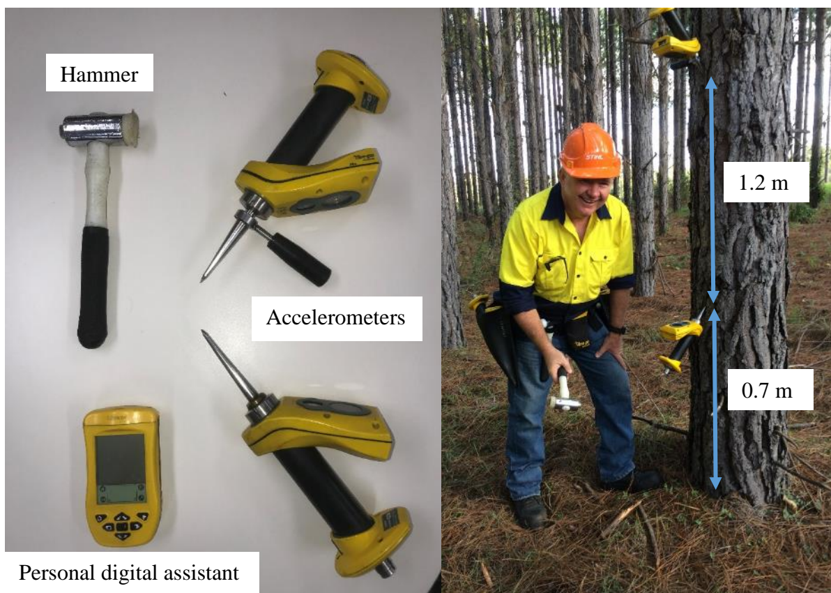
Figure 124. Experimental setup used for testing standing trees (ST300, Fibre-gen, Inc.)
