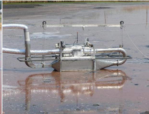
Figure 8: Close-up of wind tunnel suspended from cableway above liquor, control pond, piggery C
