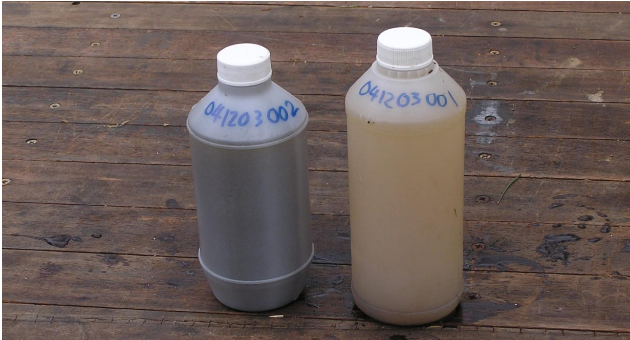
Figure 49: Comparison of liquor from covered pond (clear, with dark green colouration, LEFT), with that from control pond (turbid, RIGHT)
