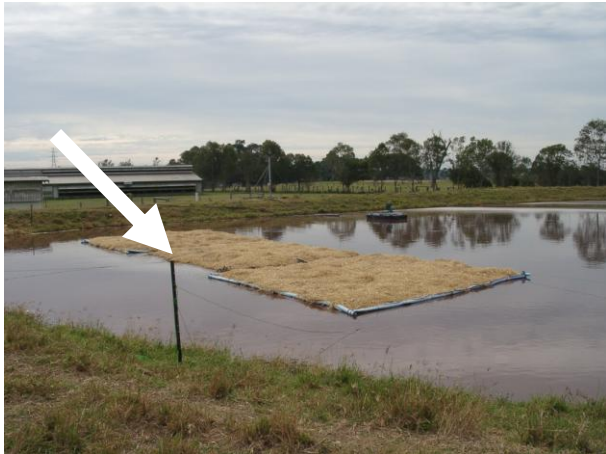
Figure 110: Trial supported straw covers soon after deployment (July 2000)
