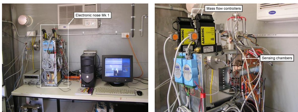
(a) Electronic nose system comprising power supply and electronics, pneumatics control, sensor chamber and PC
