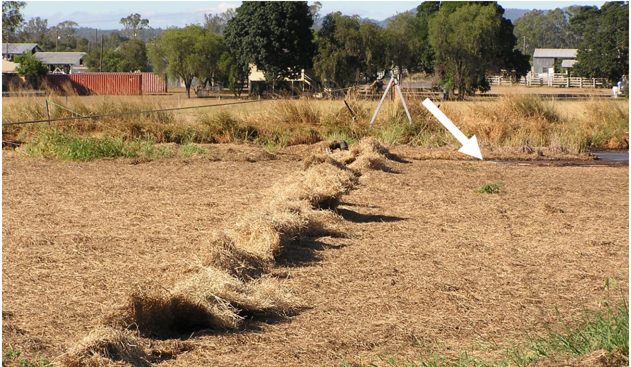
Figure 114: Relocated trial supported straw cover 57 months after deployment (April 2005) – grass cover under stress
