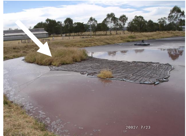
Figure 111: Trial supported straw covers 24 months after deployment (July 2002) – note well established grass cover on left hand cover unit.
