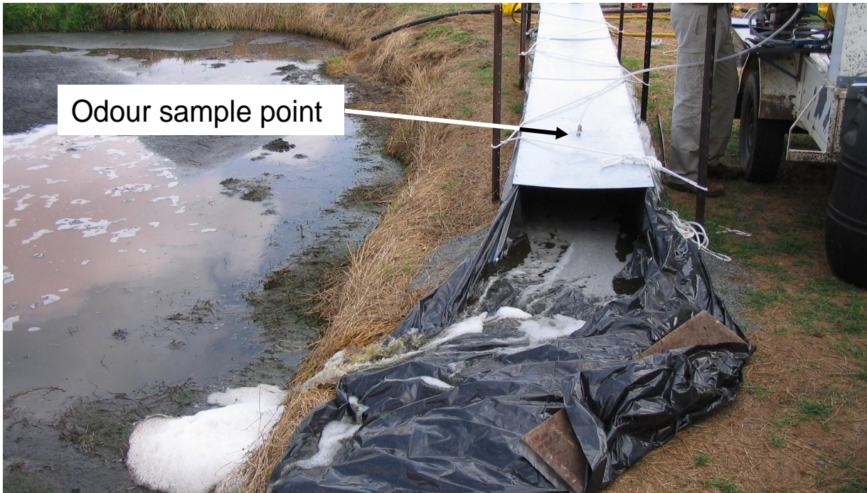
Figure 16: Odour sampling from flume during flushing
