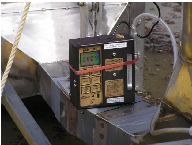
Figure 24: VOC sampling pump
