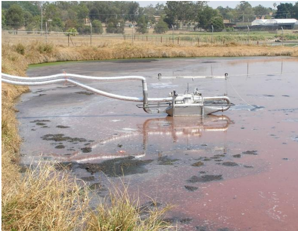
Figure 7: Wind tunnel suspended from cableway above liquor, control pond, piggery C
