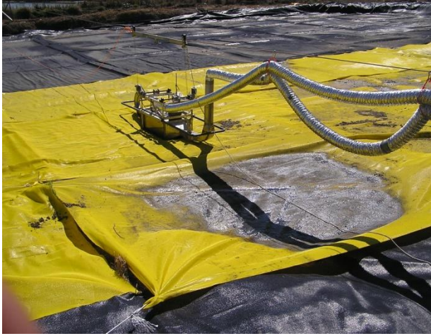
Figure 9: Sampling from cover, adjacent to “window” cut into polypropylene cover
