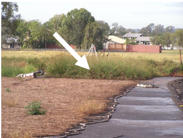
Figure 112: Relocated trial supported straw cover 45 months after deployment (April 2004) – note persistent grass cover
