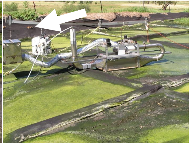
iv) Cover after 13 months (March 2004); Note minor damage (arrow)
