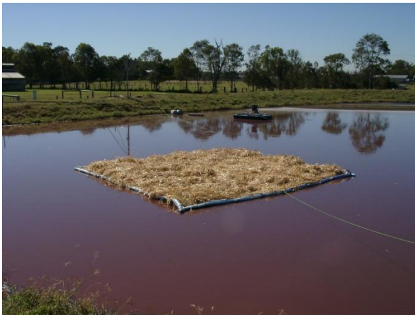
Figure 88: Trial supported straw cover in position
