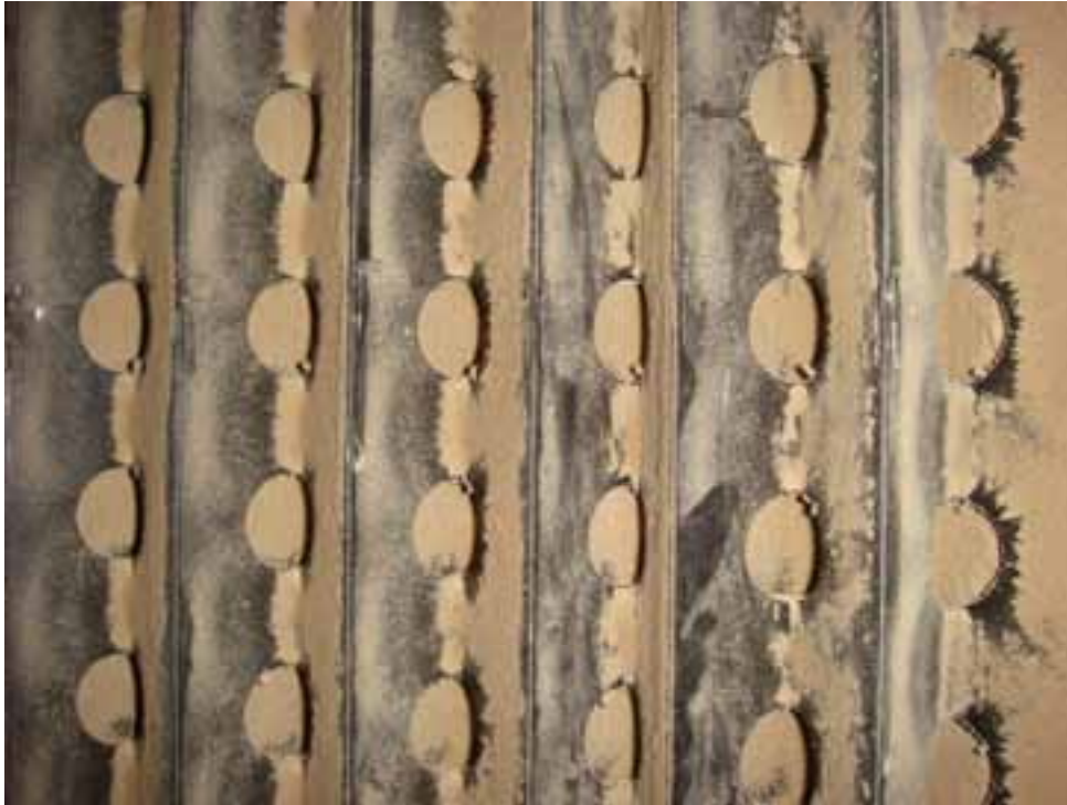
Figure 10 The front face of StuffNix showing accumulation of dust on the inside of the filter ( Note: filter maintenance had been neglected and required de-dusting )
