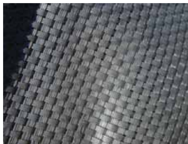
Figure 44 Close up of the woven geotextile material used on the BioCurtain®
