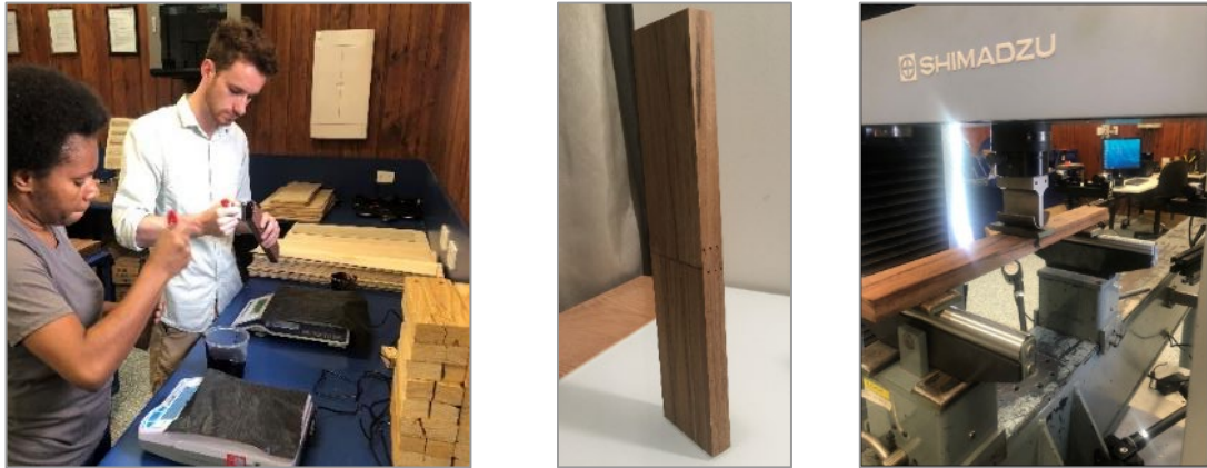
Figure 15: Finger-jointed hardwood sample manufacture (left), finished sample (centre) and testing (right).
