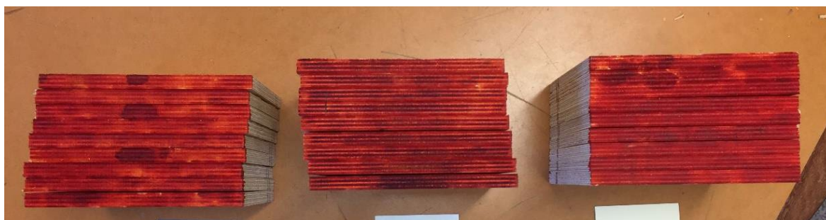
Figure 23: FR treated plywood with chemical test indicating retardant penetration.
