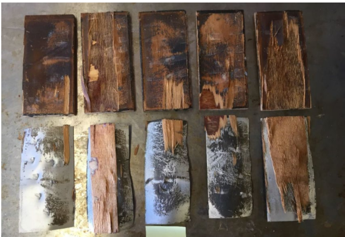
Figure 22: Aluminium overlaid plywood bond quality testing.
