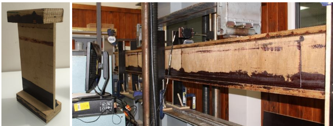
Figure 19: Engineered timber I-beam sample (left), and testing (right).
