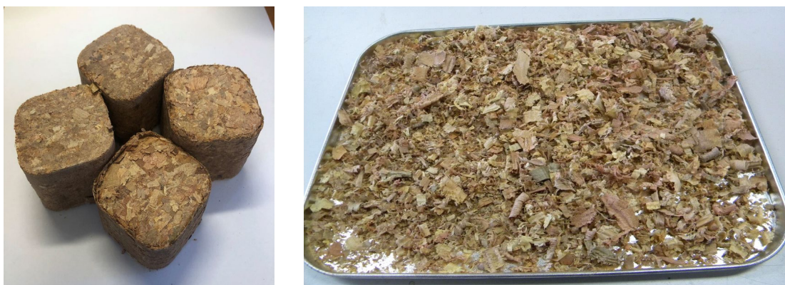
Figure 18: Compacted briquettes (left) made from sawmill residues (right).
