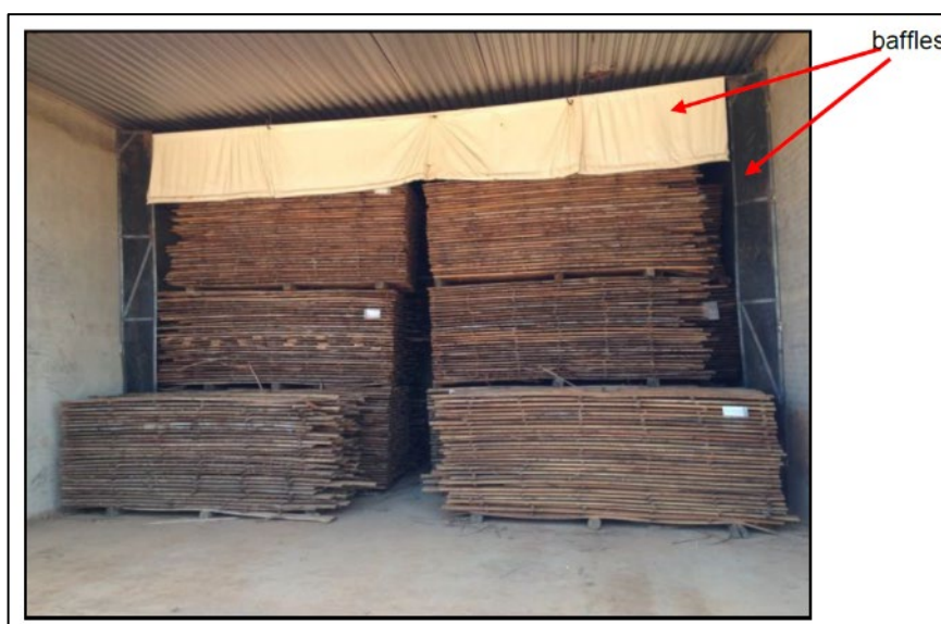
Figure 8: Use of baffles to improve kiln air flow (from Drying in PNG – Survey and recommendations).
