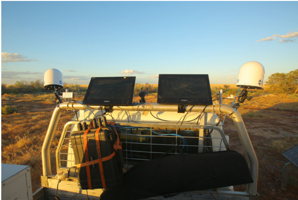
Fig. 3. Photograph of the thermal image cameras mounted to the headboard of a tray-back vehicle.
