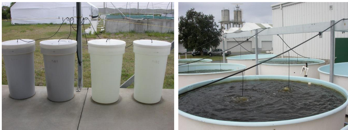
Figure 11 – Intermediate 200 L algal cultures (left) and mass cultures in 5000 L tanks (right)
