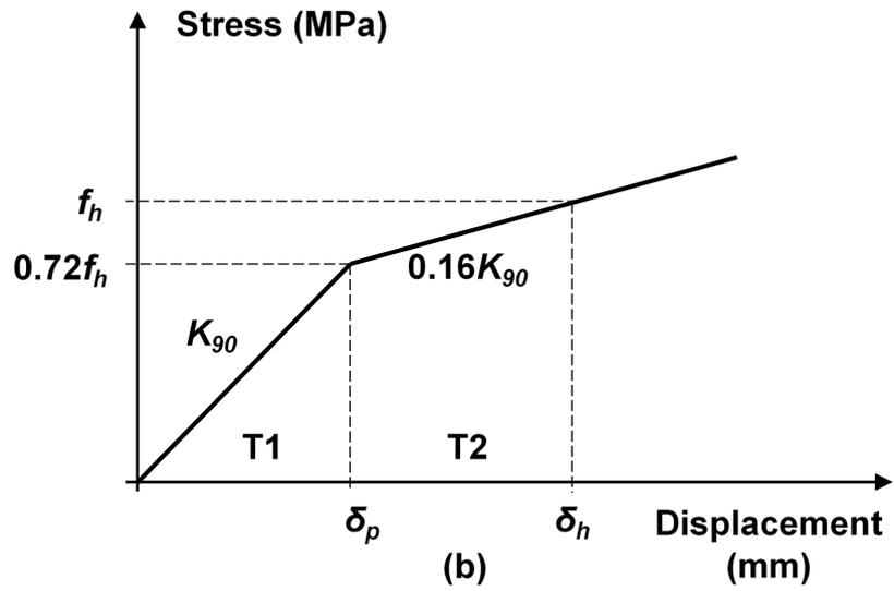
Fig. 3 (a) Tri-linear model when loaded parallel to grain and (b) Bi-linear model when loaded perpendicular to grain
