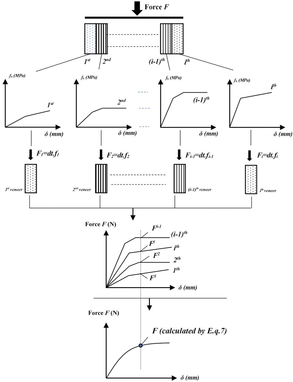
**Fig. 4** The load-displacement curve of a  $i$ -ply LVL
