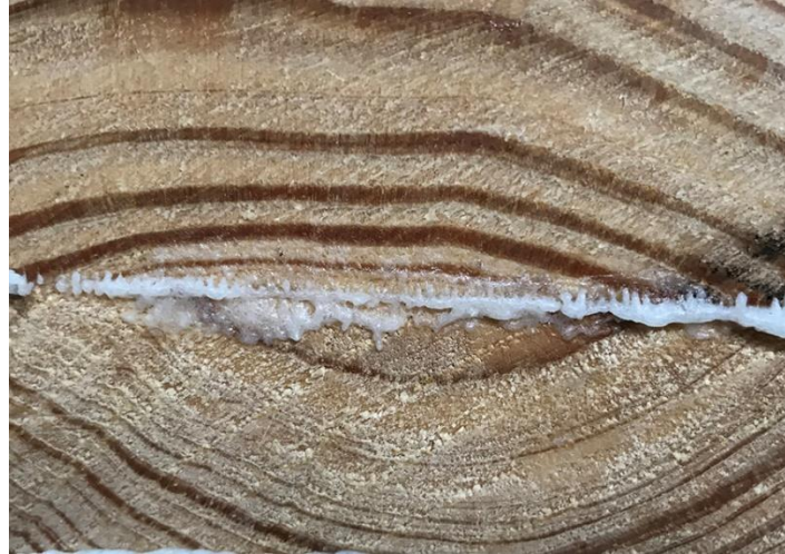
Fig. 5. Higher spread rates and application perpendicular to the incisions were two techniques used on incised samples to ensure adhesive penetration into incisions.
