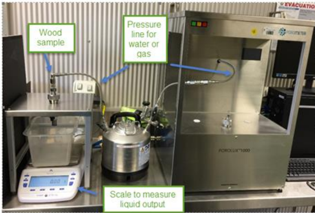
Fig. 2. Permeability test being undertaken using the Porolux 1000
