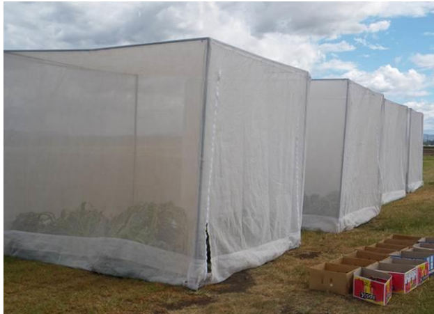
Plate 2 Treated fruit exposed to fruit flies within field cages
