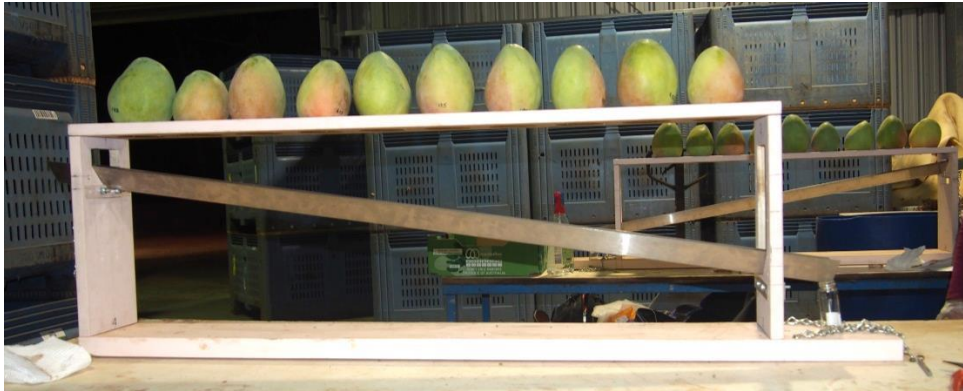
Plate 1 The desapping rack used to collect sap from the 20 fruit per replication. Ten fruit were desapped at one time.
