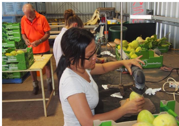
Plate 2 Applying the USB abrasion test with a small orbital finishing sander.
