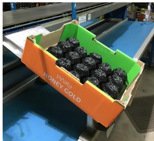
Plate 2 The suspension liner in the tray. Note the 1 cm gap between the liner and the inside of the tray (left), which results in a gap at the top of the tray when inclined for packing (right).
