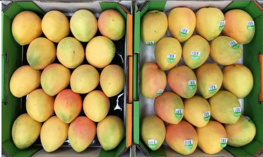
Plate 4 Tray with suspension liner (left) and the currently used expanded polystyrene liner, on arrival at Wamuran. The fruit in the suspension liner showed less re-orientation than those in the standard liner.
