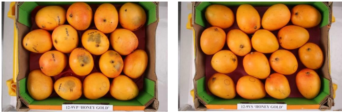
Plate 1 NT farm: 'Honey Gold' mango fruit following nine hours vibration at 15 Hz, with either the standard plastic insert (left) or these softer expanded polystyrene insert (right).
