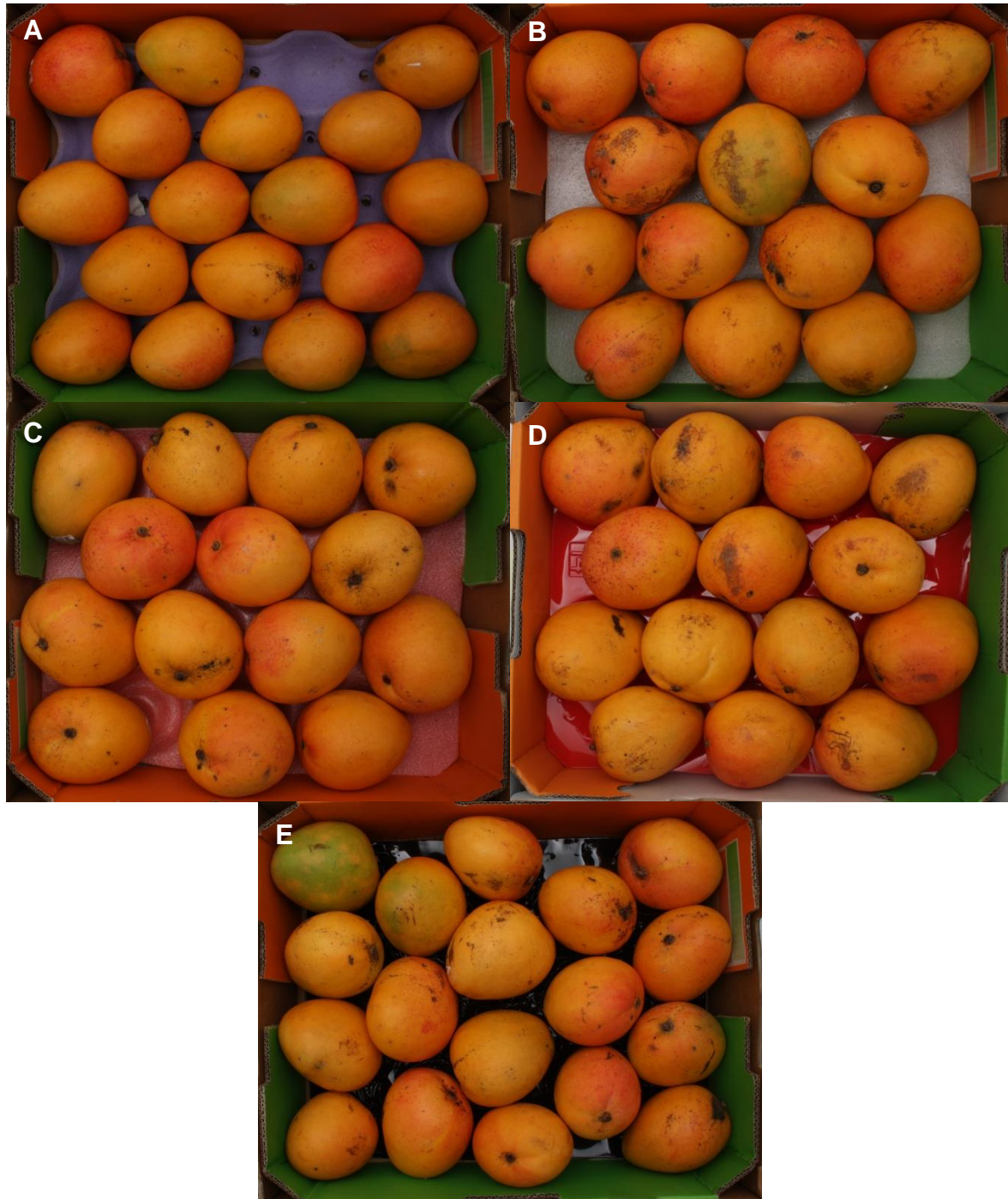
Figure 4. Physical damage resulting from 3 hours of vibration, in various tray liners; paper (A), shallow foam (B), deep foam (C), plastic (D) and the Dutch inverted suspension liner (E).
