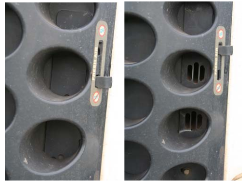
Fresh air exchange lever in the closed (left) and open (right) positions.
