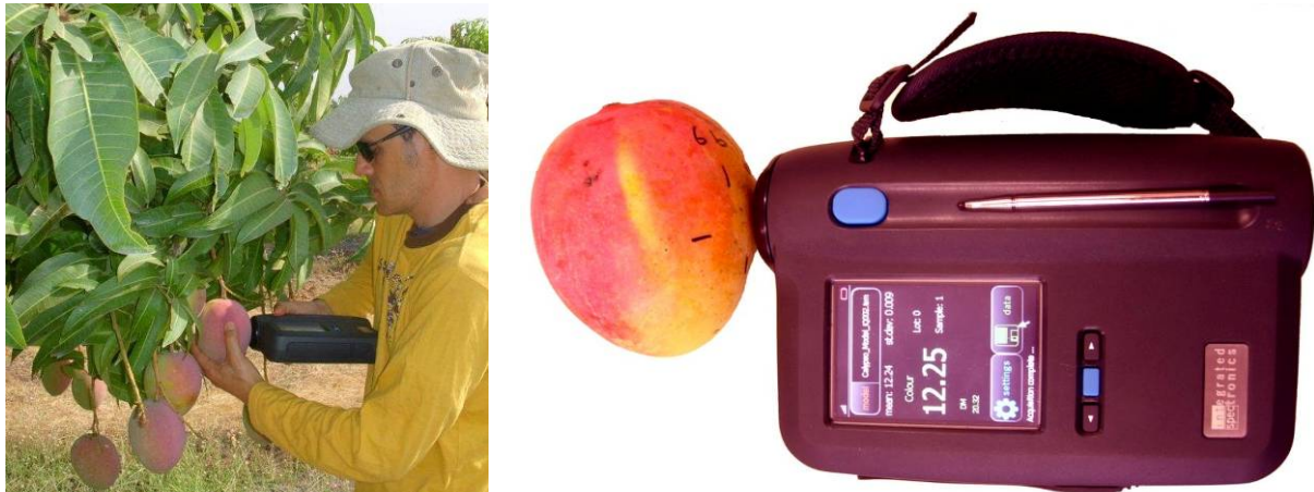
Plate 29 'Nirvana' NIRS handgun in use on a 'B74' mango tree (left) and close up of the unit (right)
