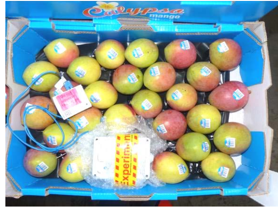
Plate 34 Temperature logger and ethylene logger inserted in the tray on the fifth layer from the top of the pallet
