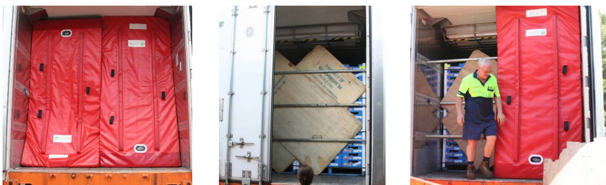
Plate 32 Examples of securing the last row of pallets. Foam batters are placed hard against the last row of pallets (left), the ply sheets placed at an angle to allow flow of air under the pallets (centre), and batters placed against spreader bars leaving about 50 cm gap between the back of the pallet and the batters (right).
