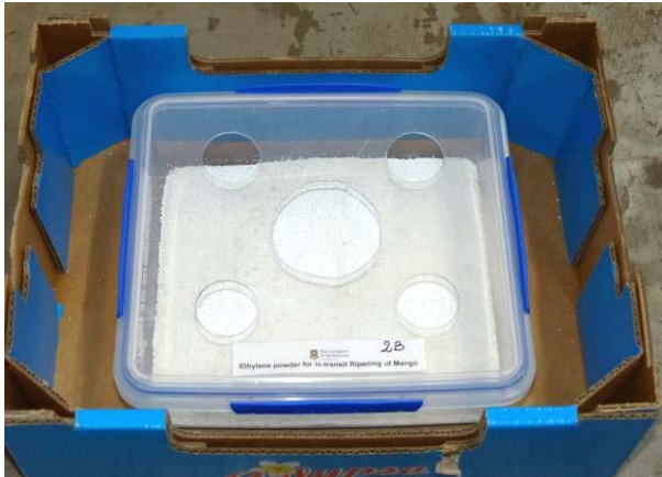
Plate 33 Plastic container with the ethylene powder and deliquescent salt before loading into the container
