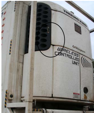
Thermo King refrigeration unit fitted with the fresh air exchange ventilation lever on the top left.
