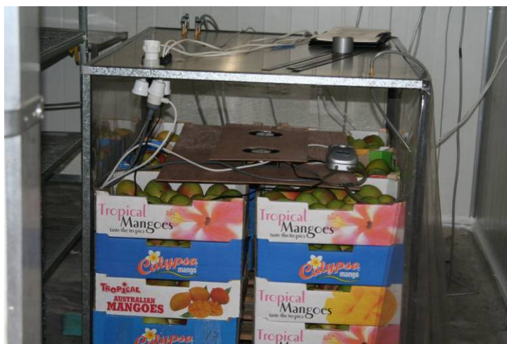
Plate 26 Ethylene treatment chamber used in the trial.
