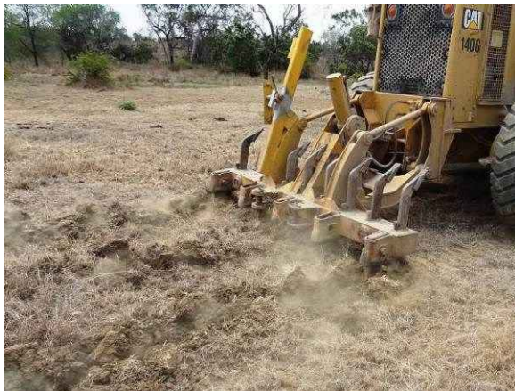
Image 7. L. Three deep ripper tynes on grader tool bar; and R. Typical trailing chisel plough for softer soil types (2011).
