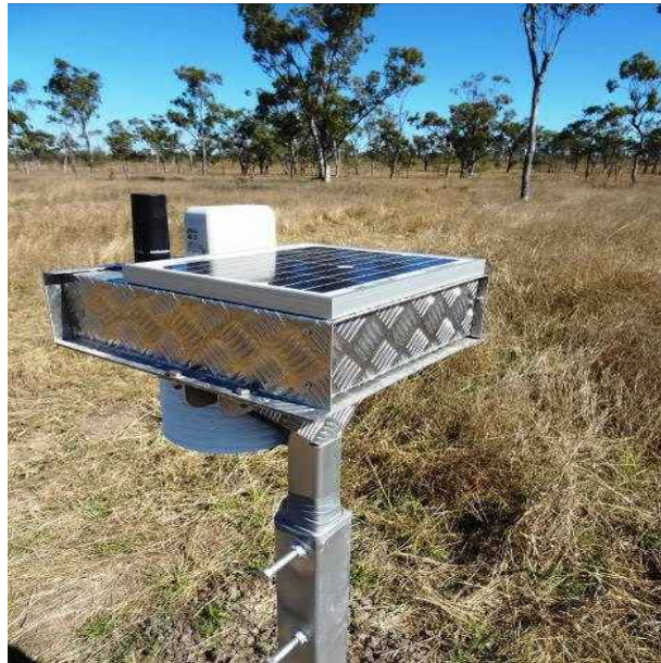
Figure 20. Solar powered weather station with satellite communication capabilities at Spyglass.
