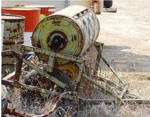
Image 8. L. Roller-drum seeder (trailed behind a vehicle) for sowing pasture seed mixes ; and R. Nine tye toolbar on grader for full surface disturbance.
