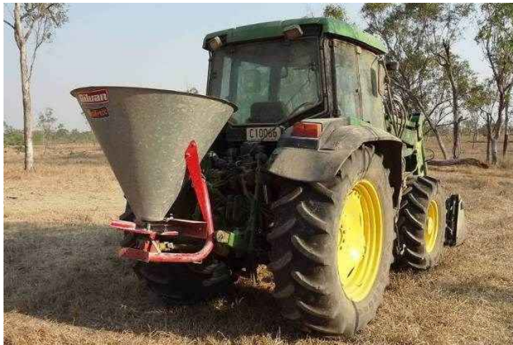
Image 9. 3-point linkage spinner broadcaster for spreading seed and fertilizer on rehabilitation sites.
