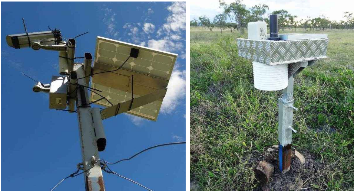
Image 16. L. Satellite transmission camera; and R. Satellite transmission weather station at Spyglass experiment site.
