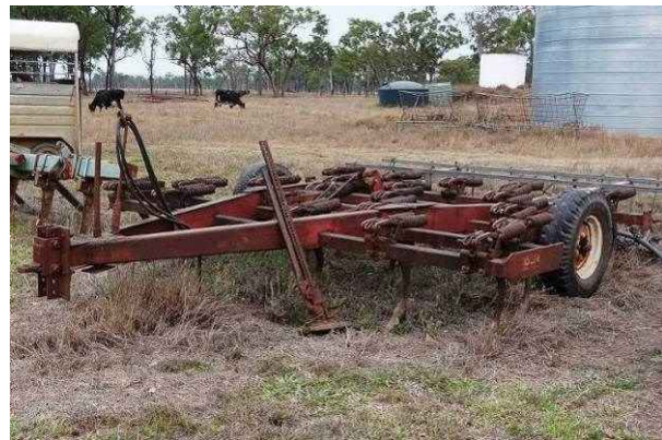
Image 7. L. Three deep ripper tynes on grader tool bar; and R. Typical trailing chisel plough for softer soil types (2011).
