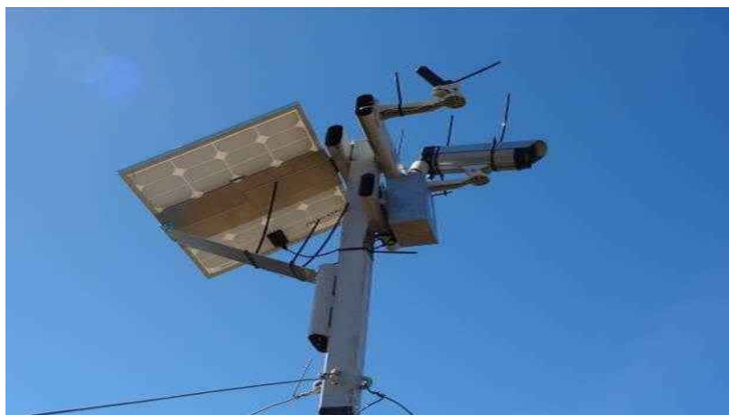
Figure 18. Remote solar powered camera with satellite transmission capabilities at Spyglass.
