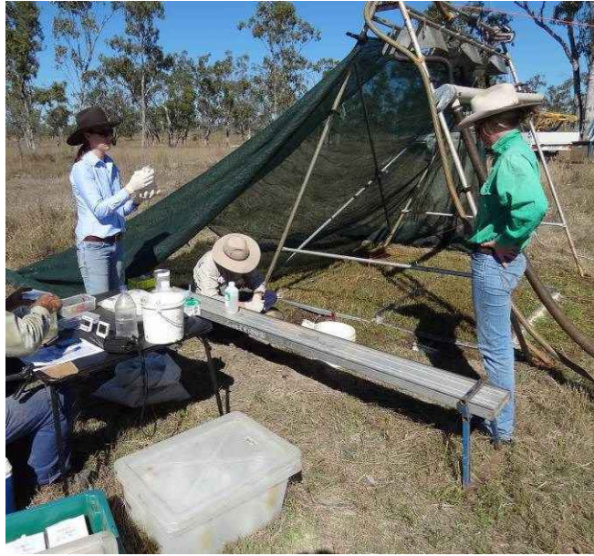
Figure 16. Rainfall simulation A-frame unit in operation at Spyglass (2012).
