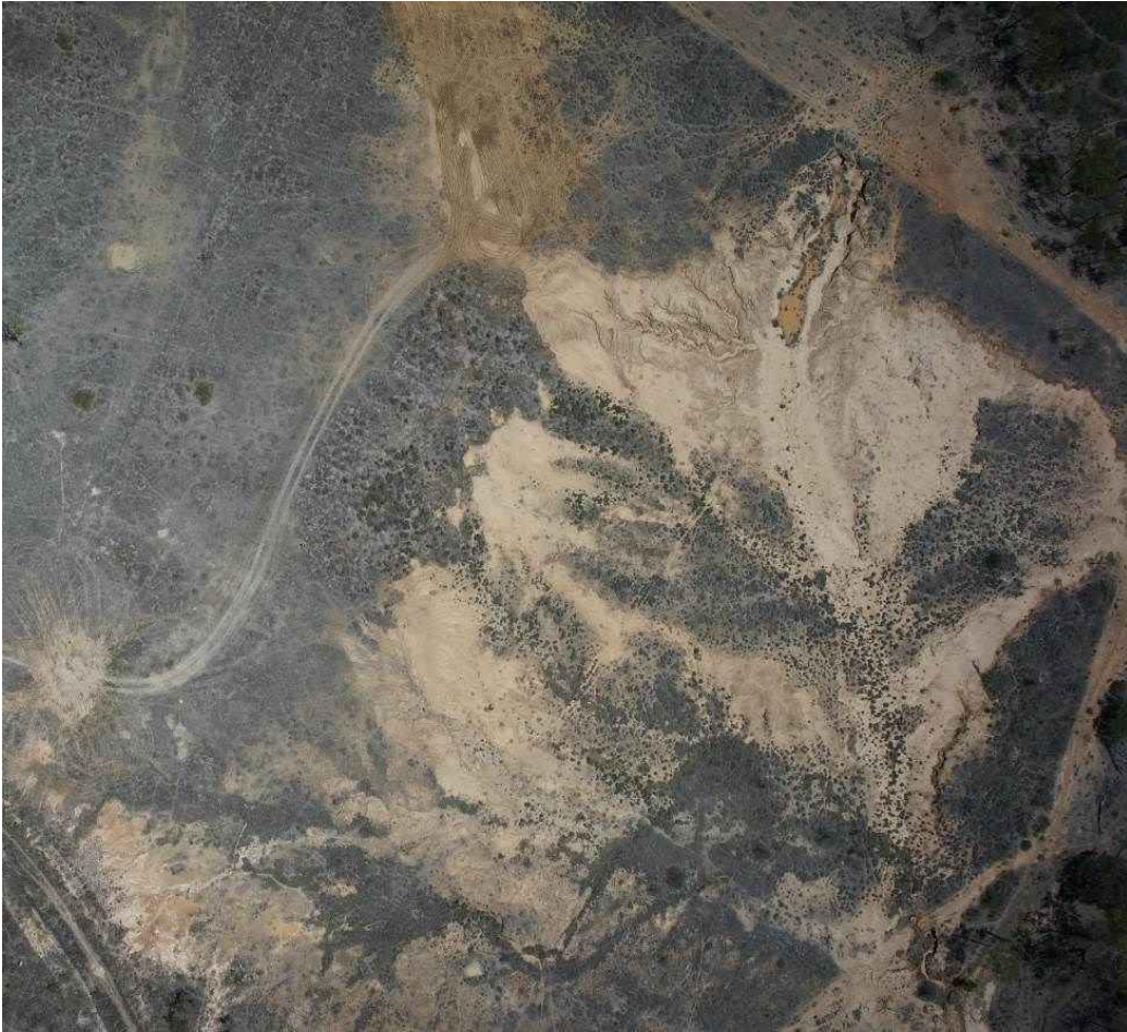
Figure 5. UAV image of hay mulch treatment (to right of road) and untreated bare gully head at Spyglass in December 2013.
