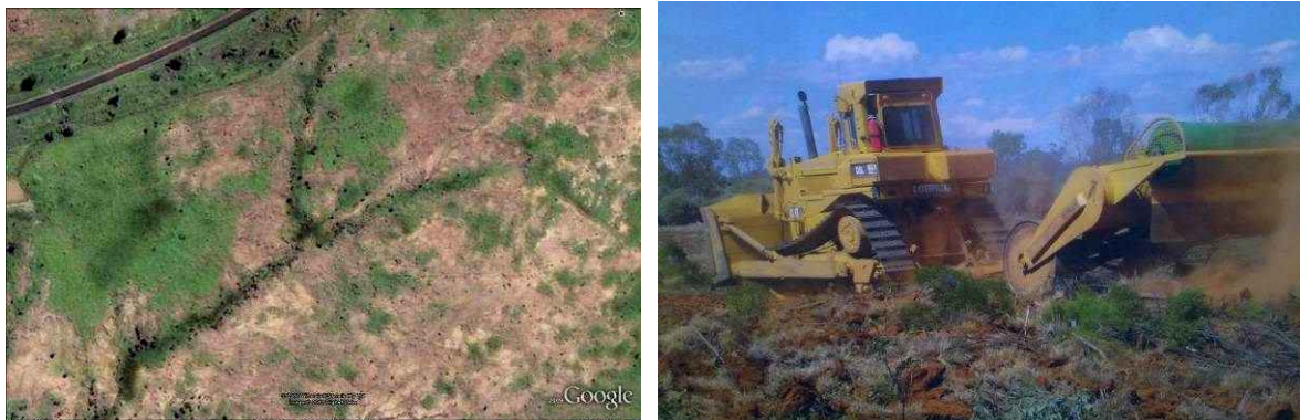
Figure 14. L. Fitzroy experiment site 2 (Banana) paddock before rehabilitation; and R. Typical blade plough with roller seeder in operation.
