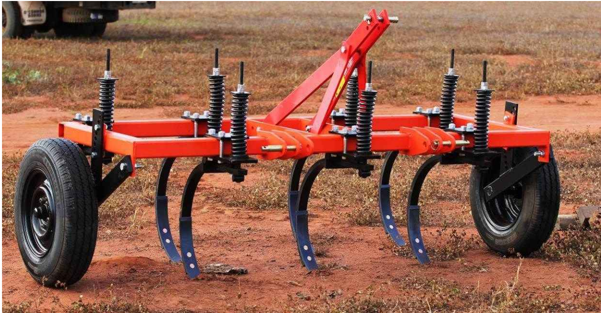
Figure 6. Seven spring tyne, three-point linkage chisel plough suitable for medium level surface disturbance for rehabilitation of clay and loam soil types.
