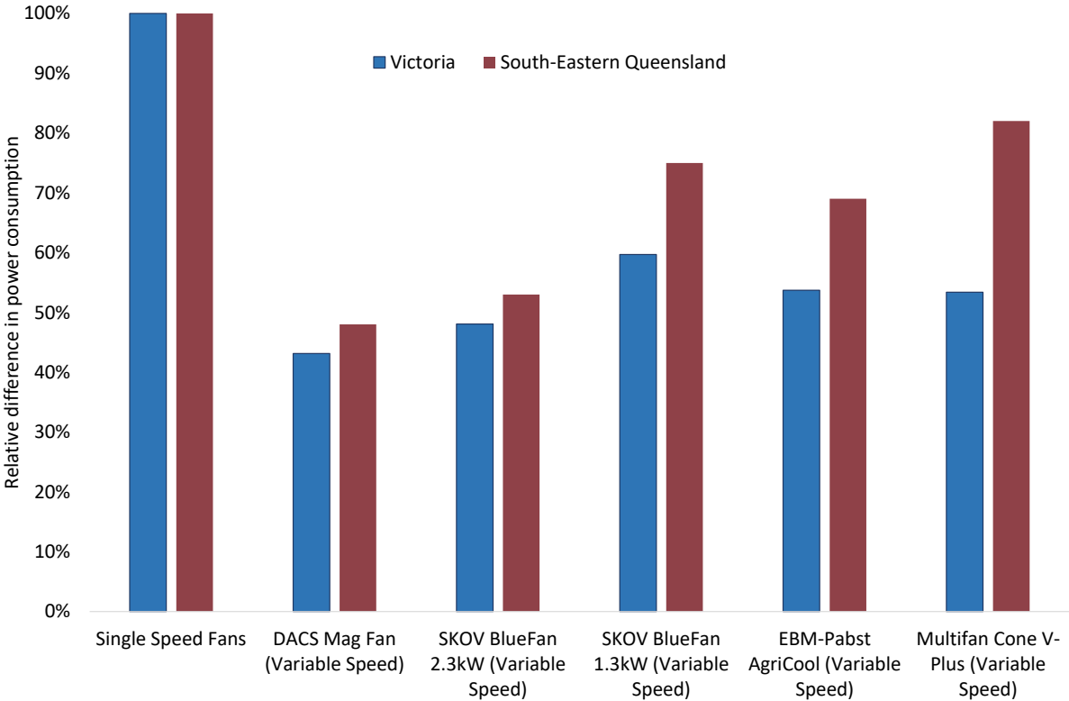
Figure 14: Calculated example showing the difference in power consumption for the variable speed fans relative to the single speed fans in Victoria and south-eastern Queensland.
