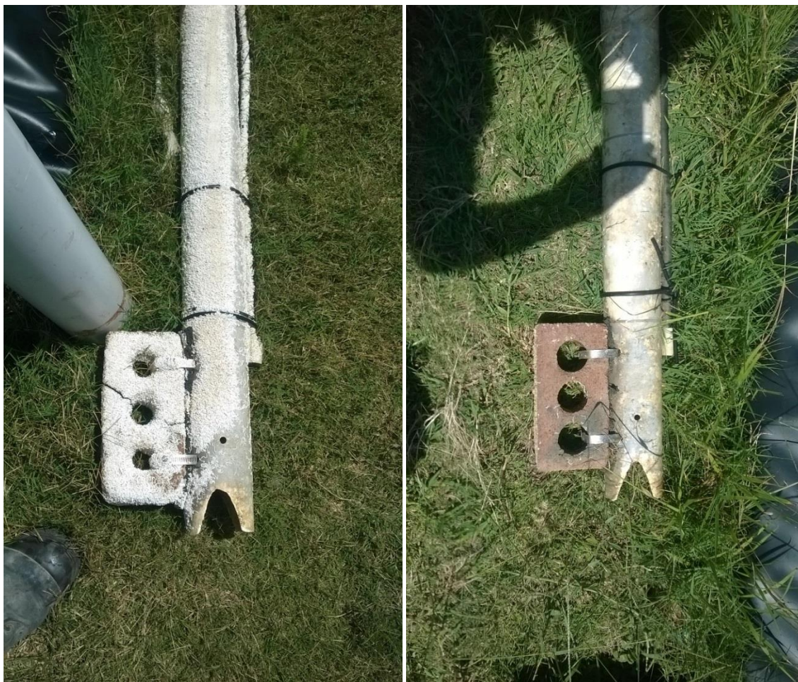
Figure 30 Lower sections of air lifts used to help distribute feed from automatic belt feeders showing higher levels of encrusting tube worms in pond G2 on left compared with pond G1 on right.
