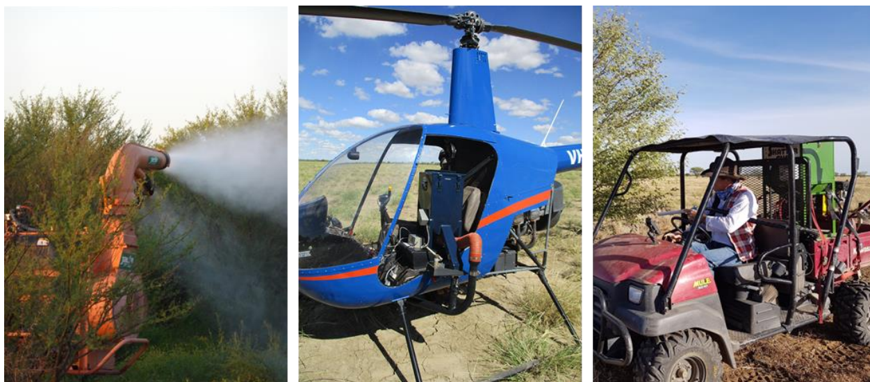
Figure 1. Agricultural mister, weed sniper and skattergun prickly acacia herbicide application equipment.
