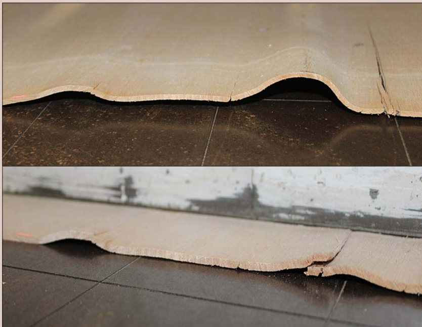
Figure 6.14. Waviness causing an overlapping split when flattened.
