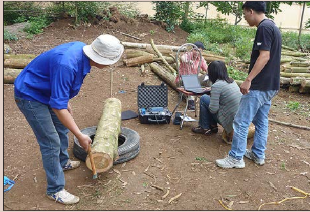
Figure 12.3. Log stiffness assessment using the Bing acoustic method.
