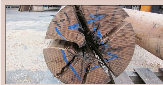
Figure 4.5. End-splitting made worse by the spindles on a spindled lathe.
