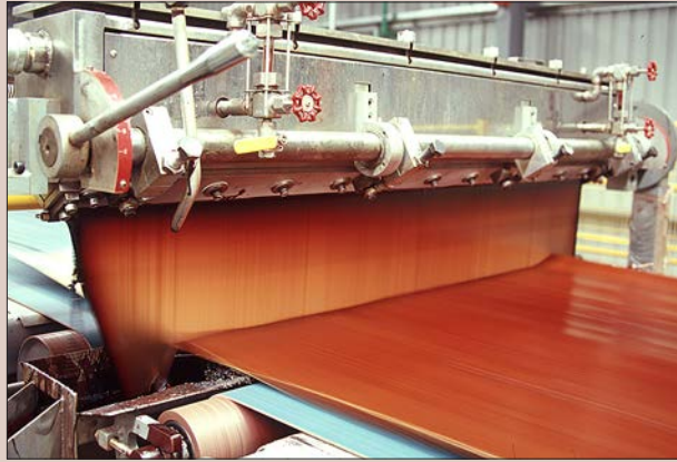
Figure 9.3. A curtain coater. Source: Wesbeam Pty Ltd, Australia.
