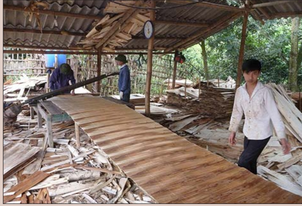
Figure 5.1. Veneer sheets being clipped manually by guillotine in Vietnam.
