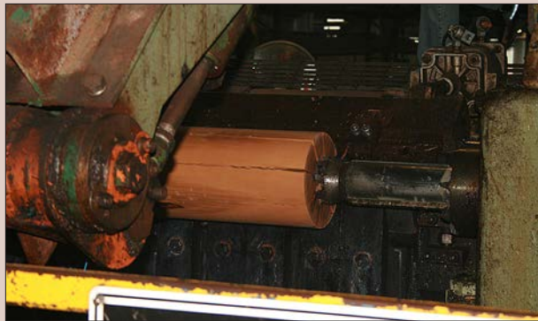
Figure 4.4. End-splitting during peeling with a spindled lathe.
