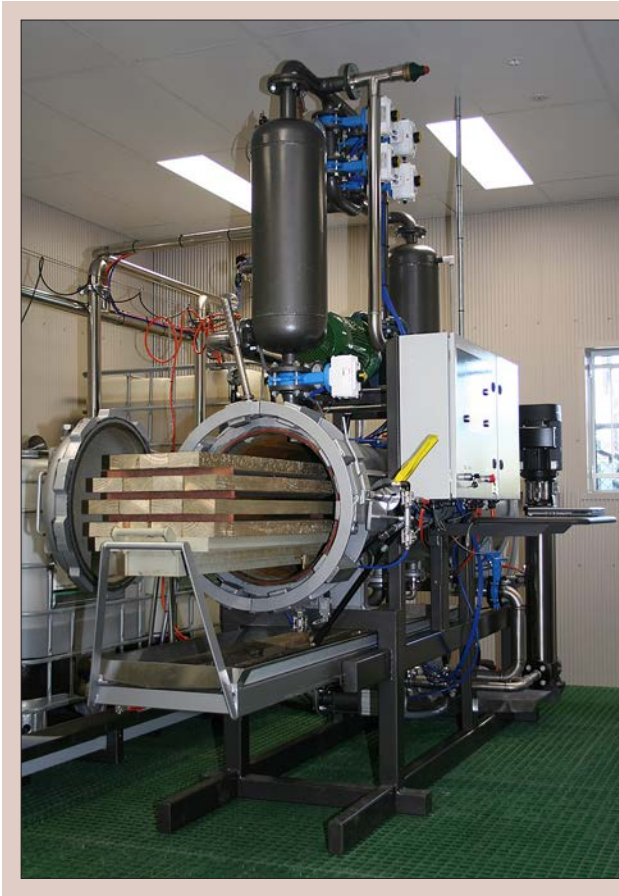
Figure 11.4. A semi-industrial scale vacuum- pressure impregnation plant.
