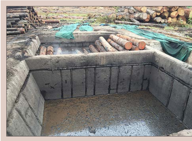
Figure 3.21. Log pre-conditioning using hot water soaking.
