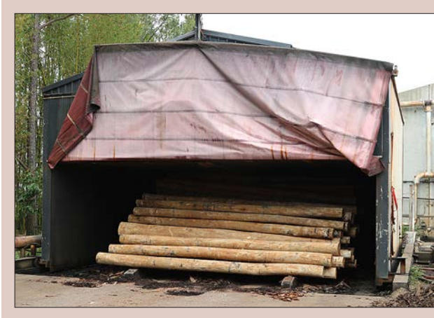
Figure 3.22. Log pre-conditioning using saturated steam.
