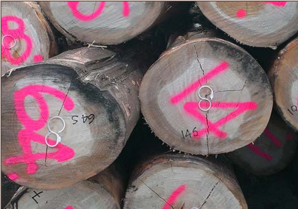
Figure 3.17. S-hooks on log ends can minimise end-splitting.
