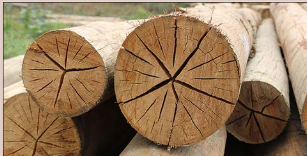
Figure 3.13. Logs can suffer severe end-splitting if they are not either processed quickly or stored correctly.
