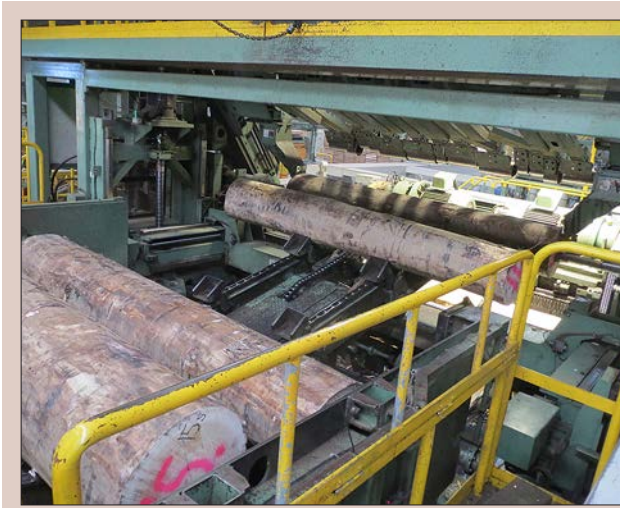
Figure 3.26. Log scanning ensures logs are positioned in the lathe spindles at the optimal location.
