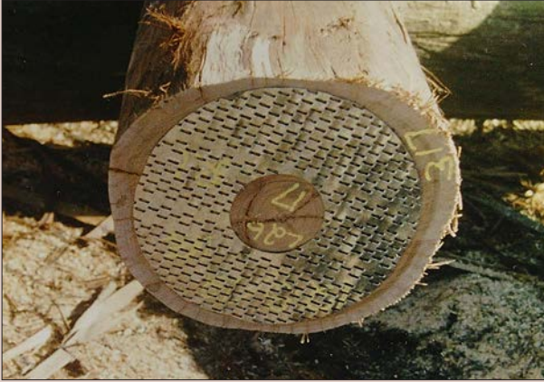
Figure 3.16. Nail-plates on eucalypt log ends can minimise end-splitting. Photo: Edgar Stubbersfield.
