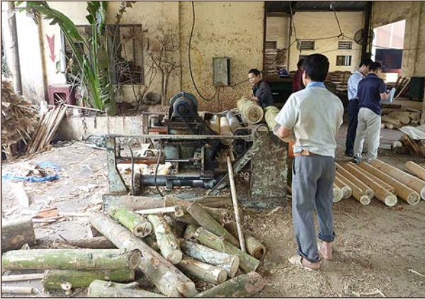
Figure 3.23. Combining debarking and log round-up in one operation in Vietnam.
