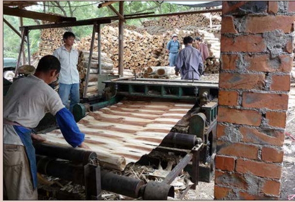
Figure 5.2. Veneer ribbon being coiled in preparation for a separate clipping operation.
