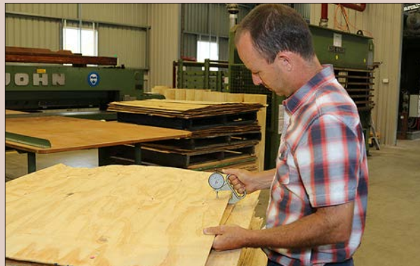
Figure 7.8. Routine checking for veneer thickness variation.
