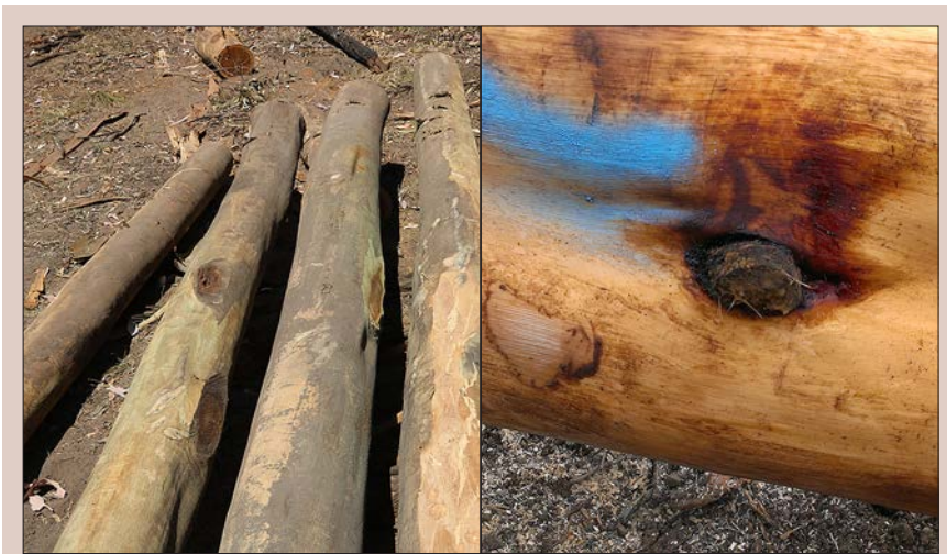
Figure 3.4. Knots (old branch stubs) visible on the surface of eucalypt logs (left), and a branch defect that produces an internal knot and hence a veneer defect (right).
