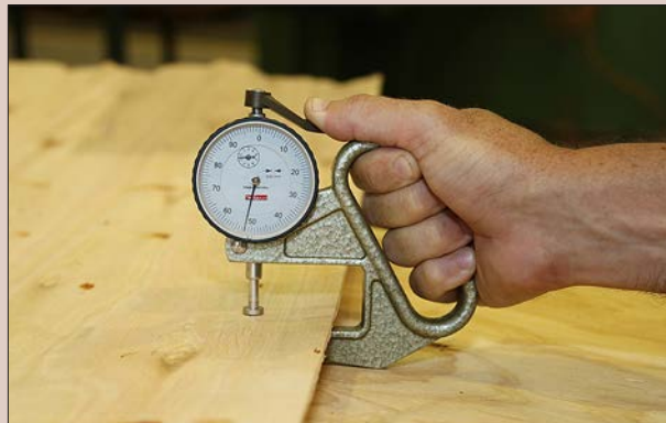
Figure 7.7. A hand-held dial gauge used to measure veneer thickness.
