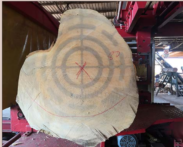
Figure 3.25. Visual aids such as a light stencil can assist the lathe operator in positioning the lathe spindles.
