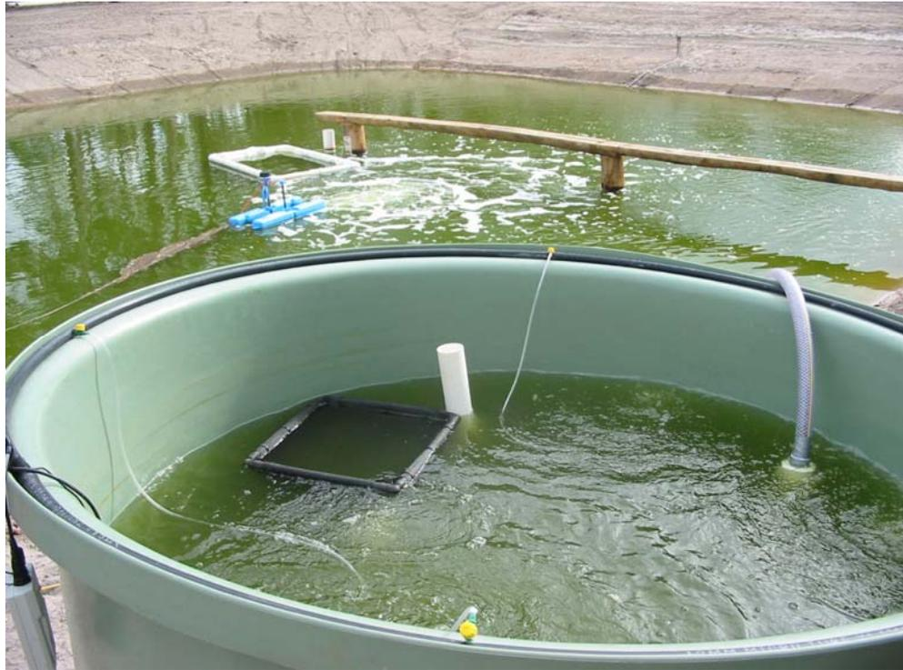
**Figure 8.4.** Acclimation tanks ( $2\text{m}^3$ ) were used on-site to lower the salinity from 10 to 2.9ppt at a rate of  $0.19\text{ppt hr}^{-1}$ . A hapas net used to monitor survival and vigour post-stocking can be seen adjacent to the pond walkway.
