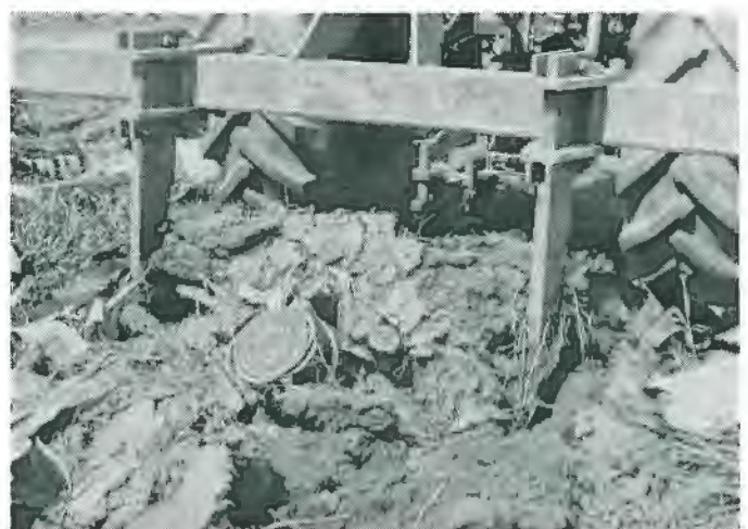
Plate 2. Digging a nursery: a cutter bar cuts roots and assists lifting of butts.
