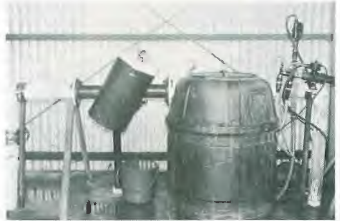
Plate 6. Fertigation essential components: from left to right, a filter, a fertiliser tank and an injector.
