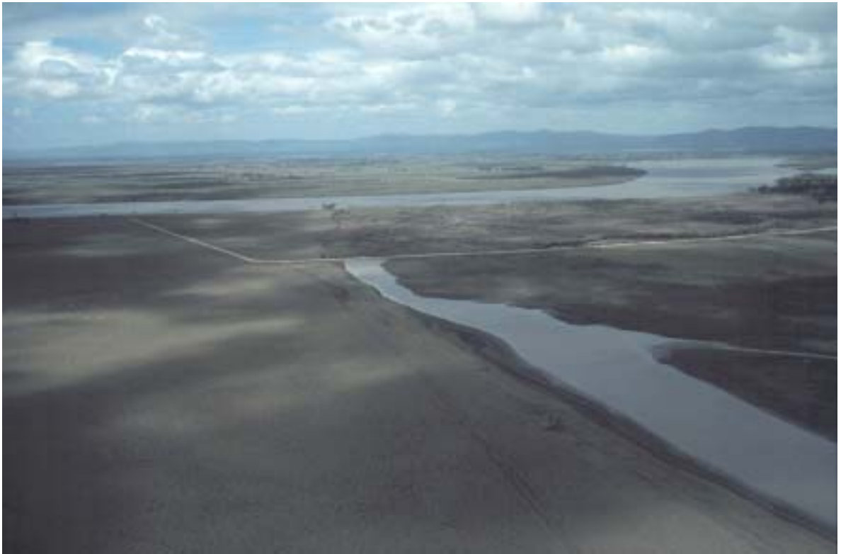
Section of pondage system adjacent to Fitzroy River showing remnant tidal channel isolated from estuary.
