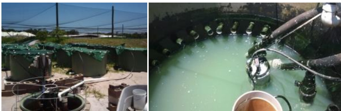
Figure 69 The experimental system showing tanks (left) and water supply from recirculation sump (right).
