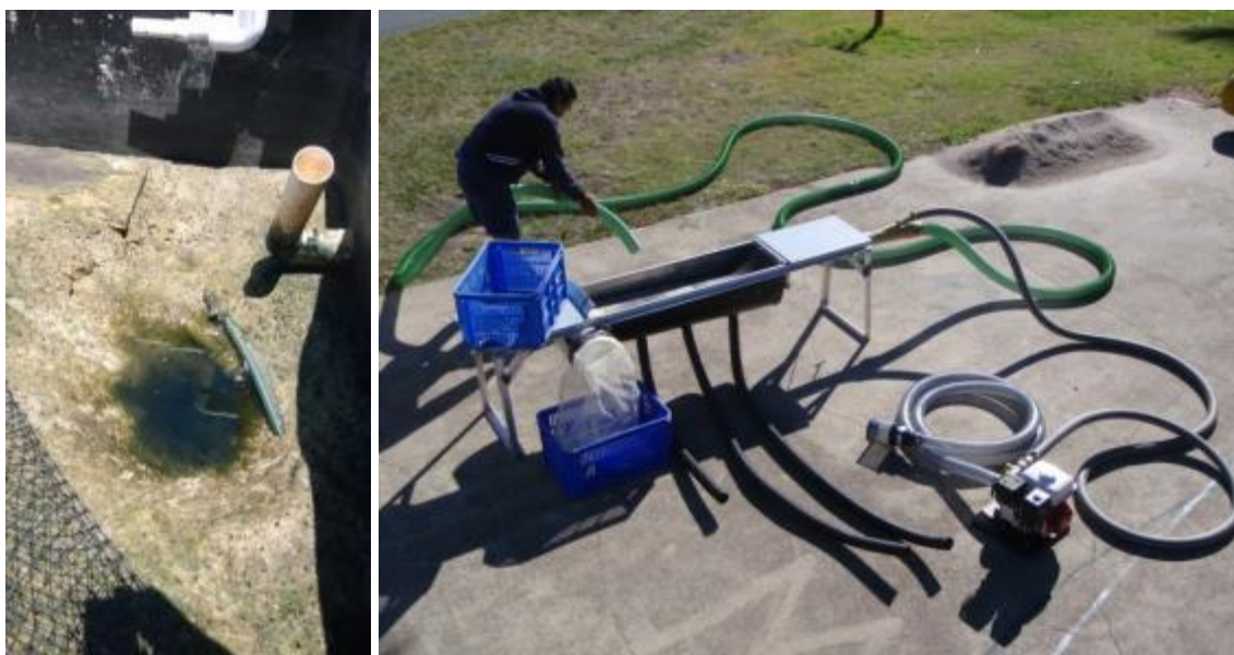
Figure 7 PASF bed showing short-circuit where water could routinely be released from the bed to allow sun drying (left) and the worm harvester (right).
