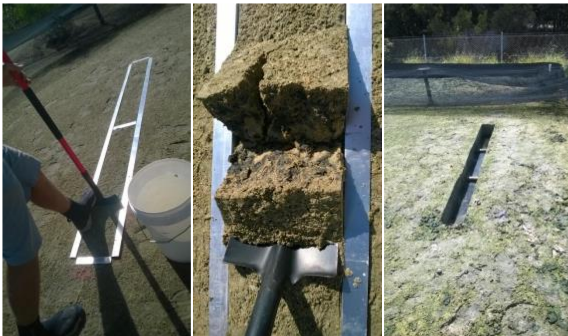
Figure 8 Quadrat sampling from PASF beds showing worm holes/burrows and substrate structure with mottling of aerobic and anaerobic sediments.
