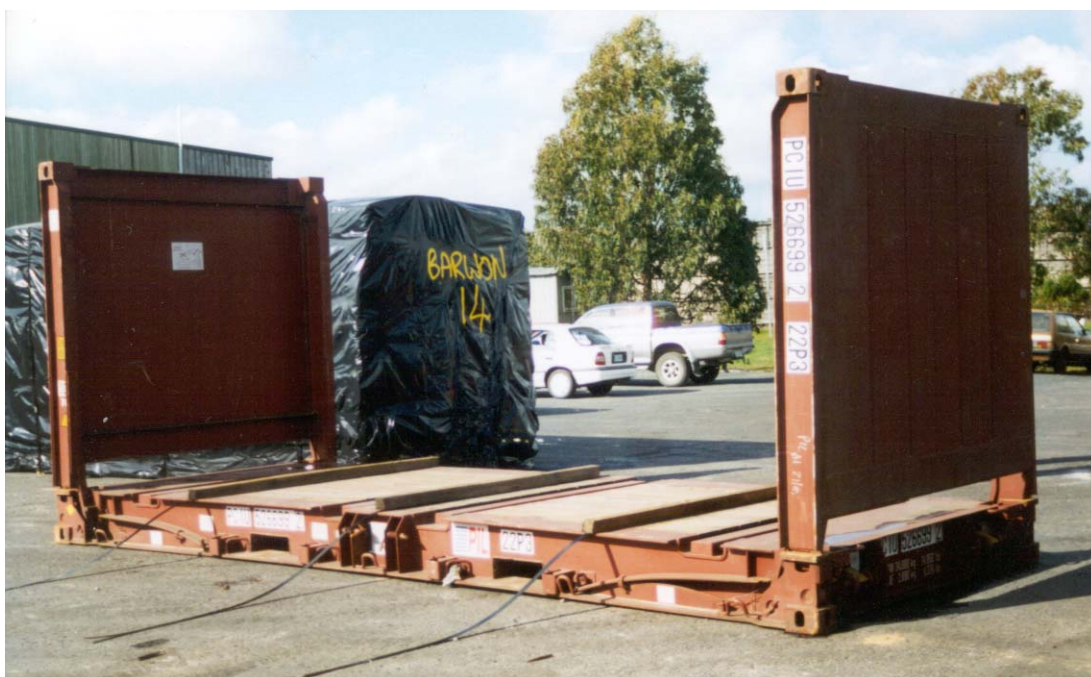
Plate 2. Flat-rack used for shipping timber boards and flooring.
