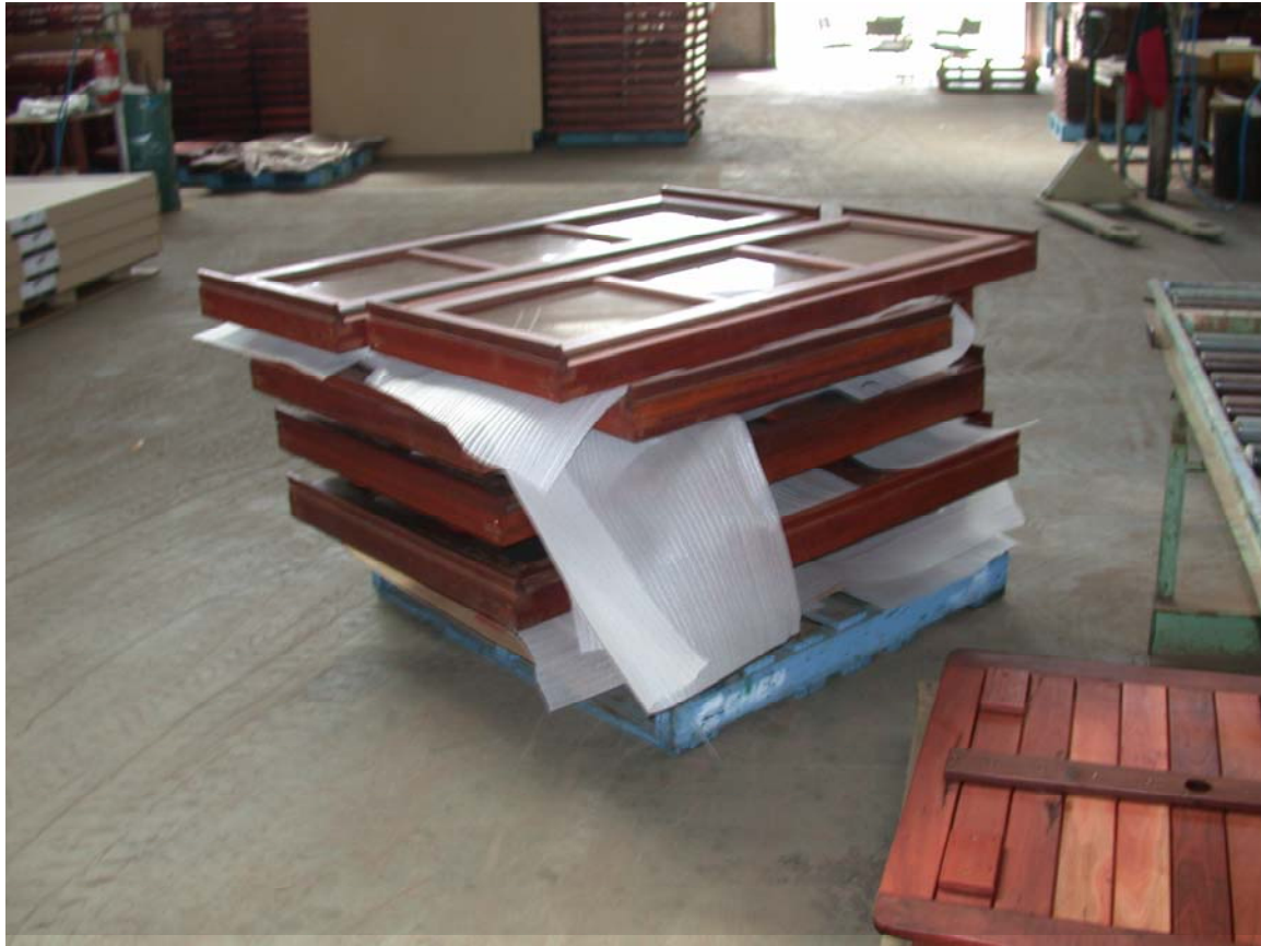
Plate 11. Celair foam between window joinery items.
