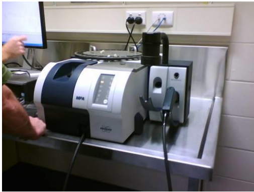
Figure 1. Bruker Fourier-Transform NIR Multi-Purpose Analyser (MPA), with a carousel
