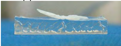
Appendix D Figure 1 Sagittal otolith from a Spanish mackerel placed in a mould half-filled with resin.
