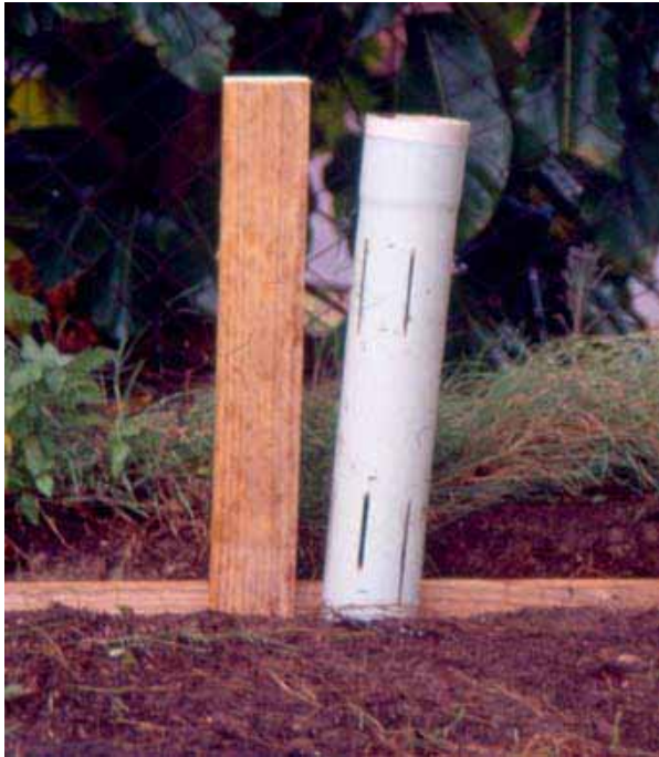
Figure 4: Termite aggregation station showing the timber and the slotted, PVC pipe before installation.
