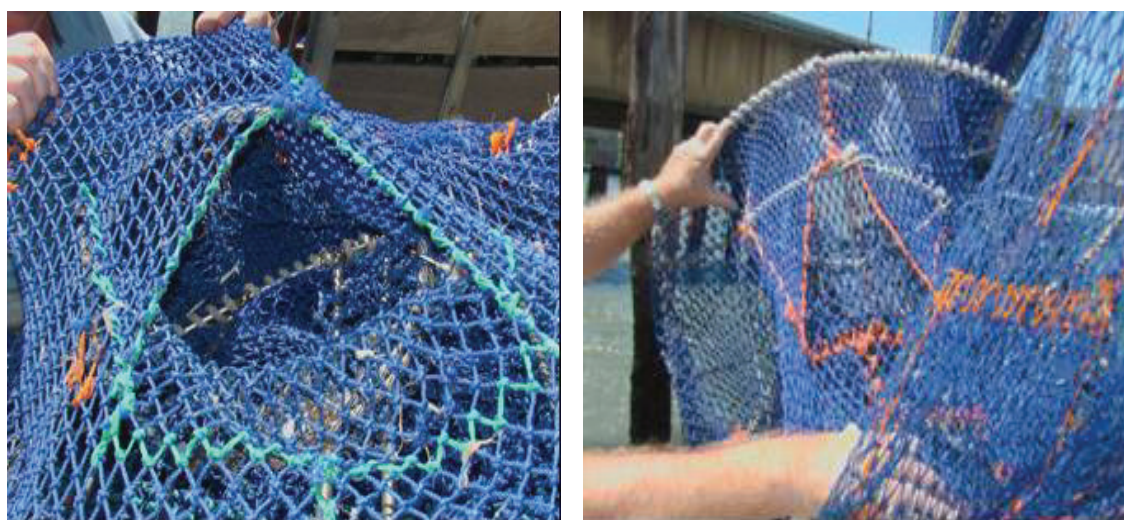
Figure 7.4.1. The BRDs installed on fisher A's vessel that were evaluated as part of the commercial fisher trials. The device on the left was constructed from steel cable, while the device on the right was constructed from stainless steel. Both devices had an escape opening sewn into the net with a flap of loose netting partly covering the opening. The flaps probably reduce or inhibit bycatch escapement. Note the close position of the BRDs to the TED frame, particularly in the right photograph, showing that the devices were positioned relatively far forward in the codend (i.e. around 90 meshes in front of the drawstring), which reduces their effectiveness at excluding bycatch. It is debatable whether these devices conform to the technical specifications required of BRDs listed in the Queensland Trawl Fishery Management Plan, but it is our experience that similar such BRD designs, and the positions that they are installed at, are common throughout the fishery.
