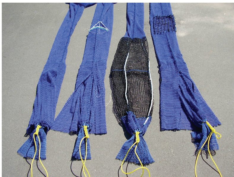
Figure 7.3.2. The four BRD ‘treatments’ compared during the charter. From left to right the devices were the standard codend with no BRD (i.e. control net), fisheye BRD, square mesh codend BRD and square mesh panel BRD. The most forward edge of each device was 50 meshes from the drawstring.
