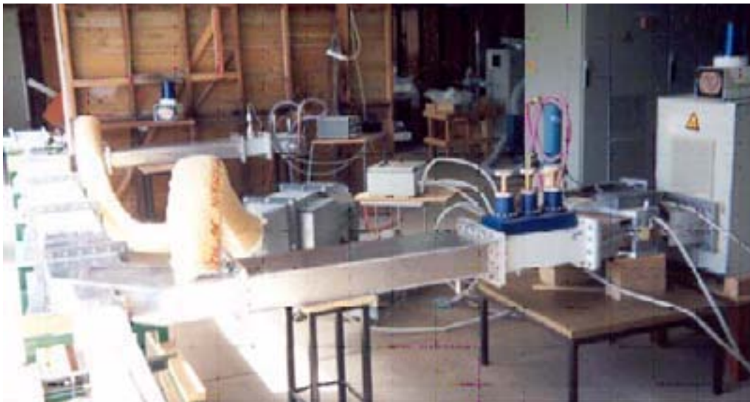
Figure 28: 60 kW microwave with conveyor applicator
