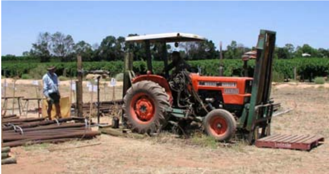
Figure 34: Posts being strength tested using the cantilever method
