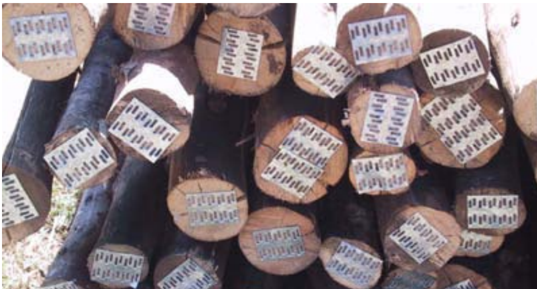
Figure 23: Gang-nailed E. globulus posts
