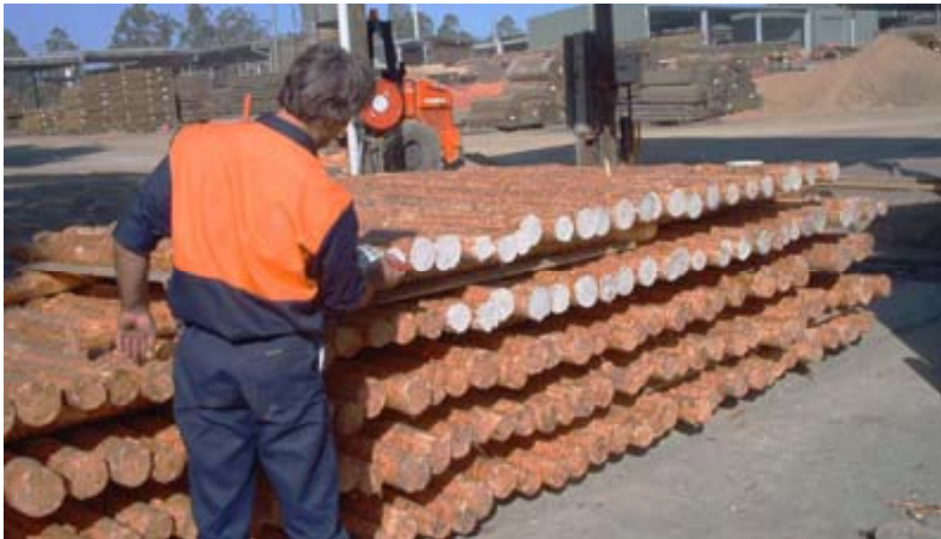
Figure 25: End-sealing P. elliotii posts
