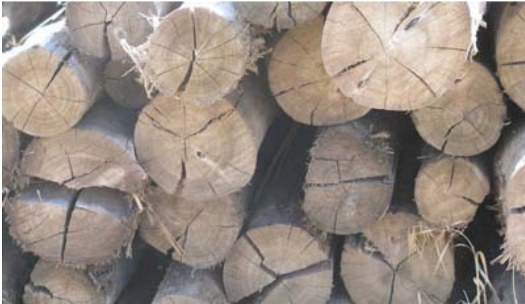
Figure 33: End splits in some posts
