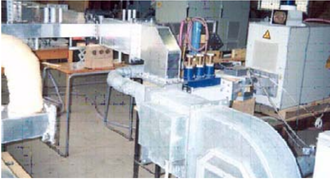
Figure 27: 60 kW microwave with box applicator
