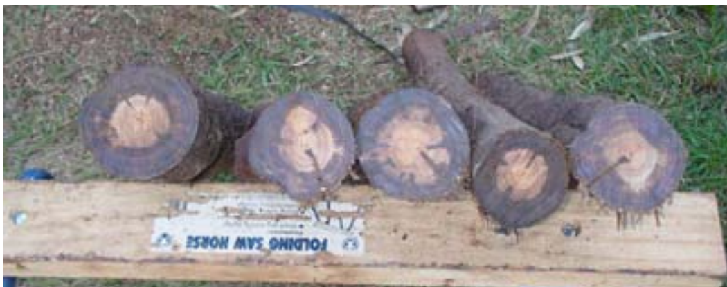
Figure 11: Full sapwood penetration of PEC in debarked only A. mearnsii posts
