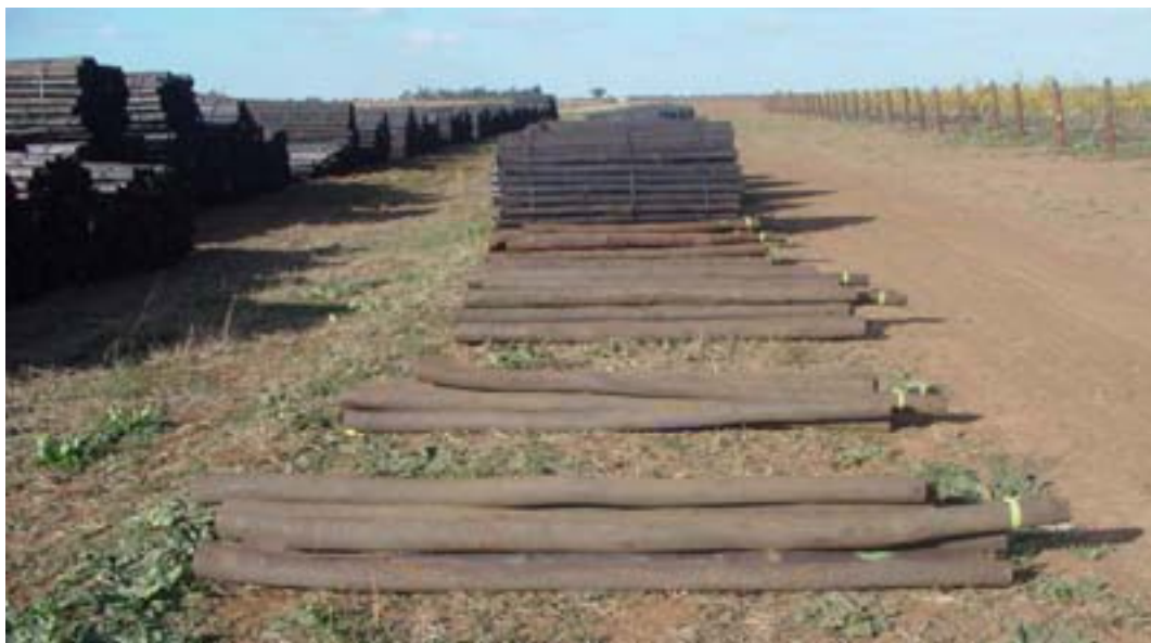
Figure 19: PEC-treated test posts alongside commercial bundles of HTC-treated P. radiata posts
