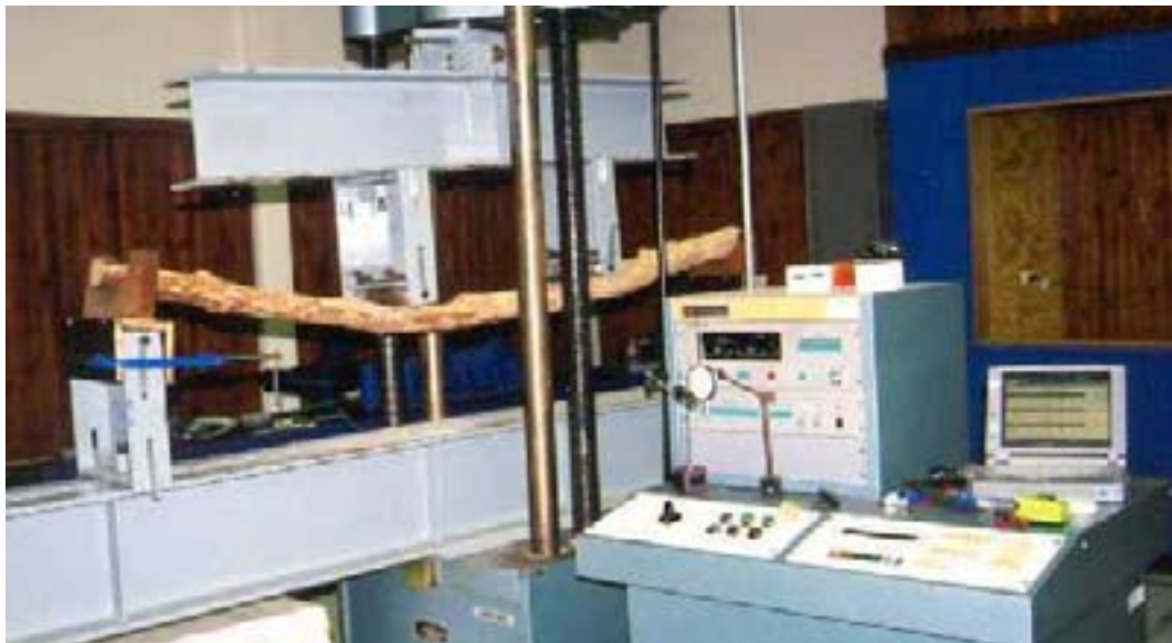
Figure 36: Strength testing an A. mearnsii post using the 4-point bending test method
