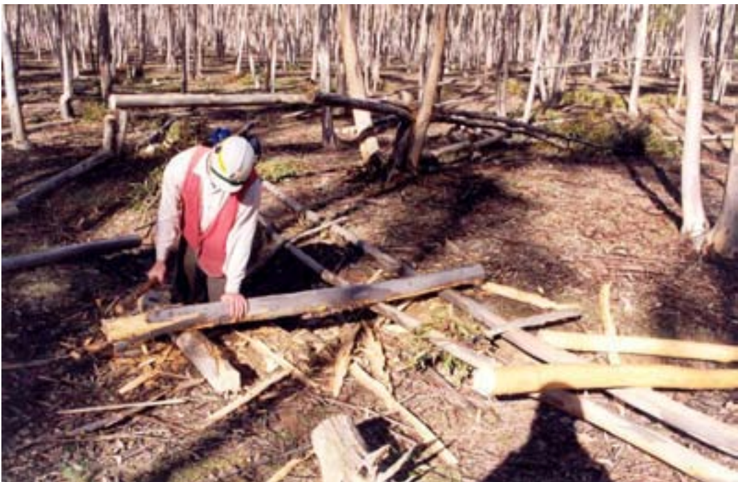
Figure 21: Debarking E. cladocalyx posts at Horsham
