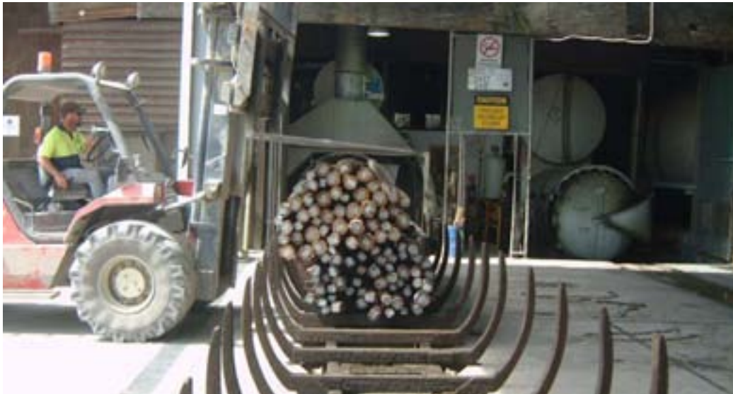
Figure 31: Untreated posts being loaded into the ACQ treatment cylinder at Perma Log Products
