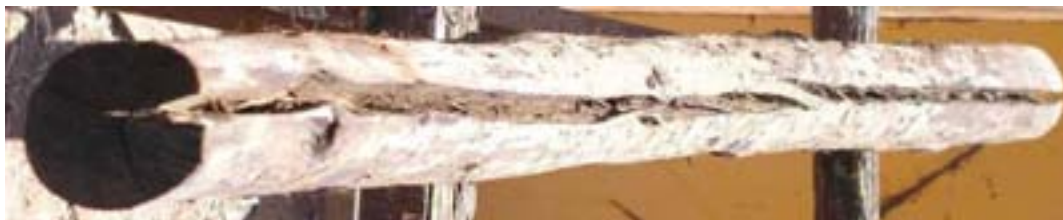
Figure 14: Full length split in A. mearnsii dried with the bark-on
