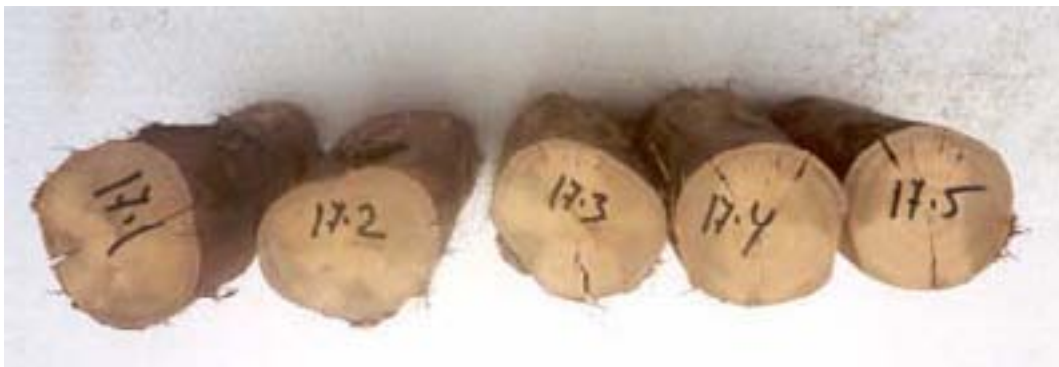
Figure 6: E. globulus post after modification using the conveyor applicator, showing uniformity of small checks. A few larger perimeter splits also developed in some posts.
