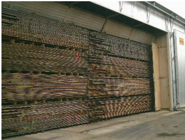
Figure 2.7 - Full kiln charge
