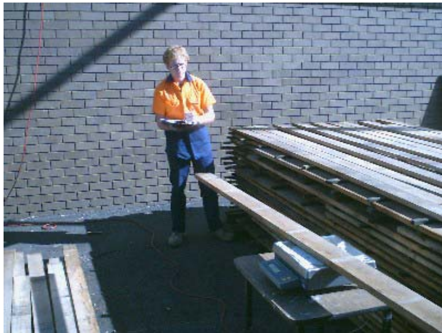
Figure 2.4 - Weighing boards during racking
