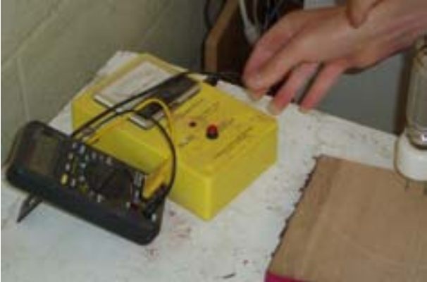
Figure 4.1.10. Deltron DCR22 resistance moisture meter connected to voltmeter & computer.
