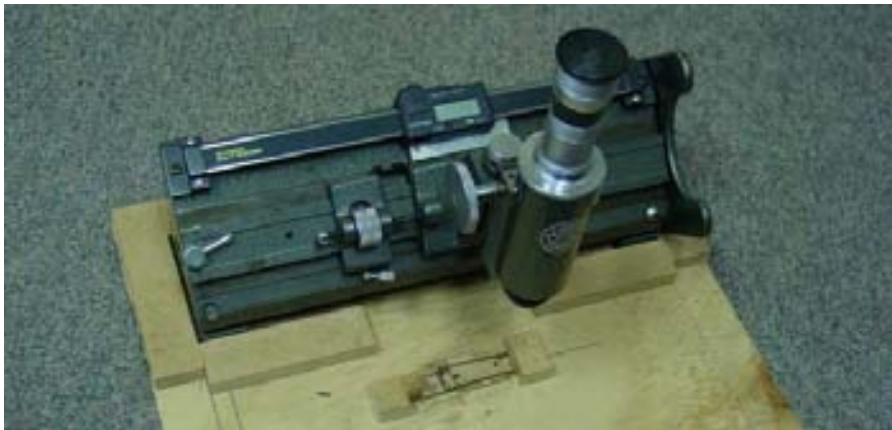
Figure 2.1.2. Apparatus for monitoring shrinkage of slices.
