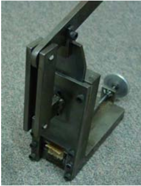
Figure 2.1.1. Apparatus for slicing timber for shrinkage and moisture content profile measurement.
