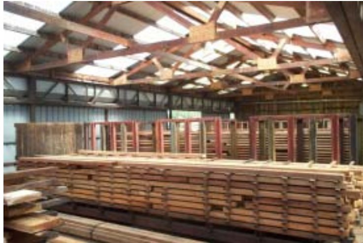
Figure 7.12. A fully enclosed racking building
