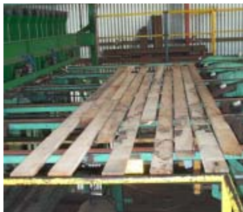
Figure7.38. Top & tailing on a racking machine
