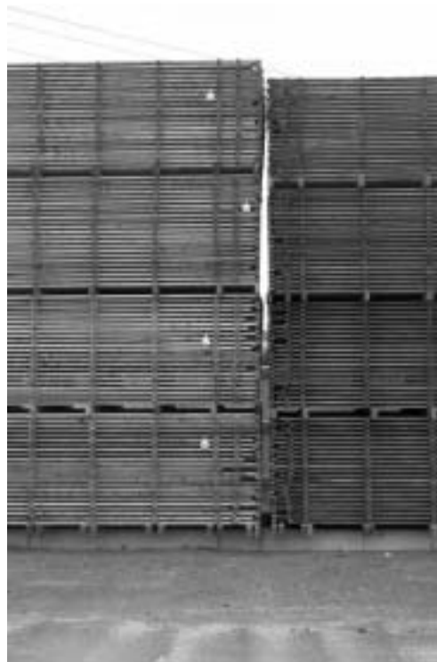
Figure 1.06. Shrinkage in 'identical' drying stacks. The stack on the right has been drying three months longer than the one on the left.
