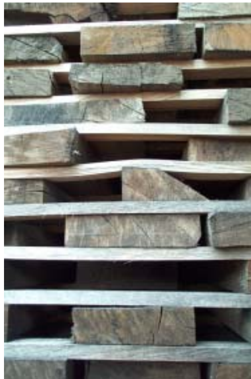
Figure 4.16. Effect of poor sawing accuracy on a rack
