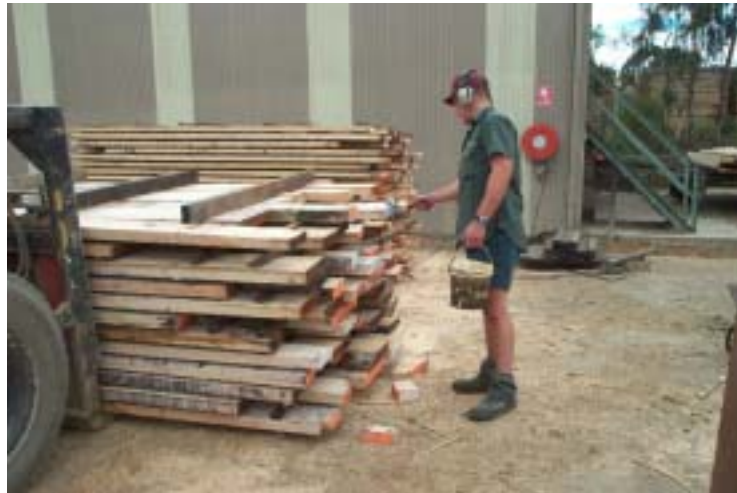
Figure7.37. Docked ends being resealed
