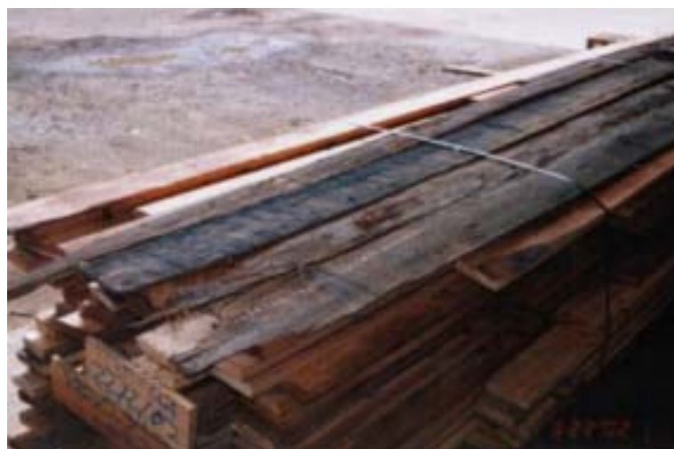
Figure 5.05. Waning boards as a pack cover. Any pack protection is better than no protection
