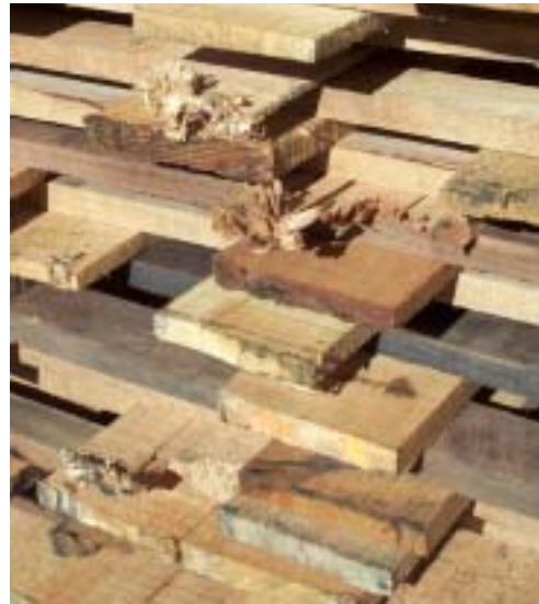
Figure 7.47. The end of poorly racked boards broken in a push through predryer
