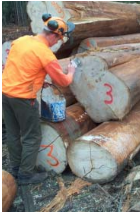
Figure 2.03 End sealing logs as they are graded
