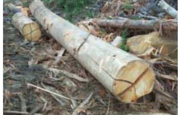
Figure 2.10. Undesirable: logs left exposed
