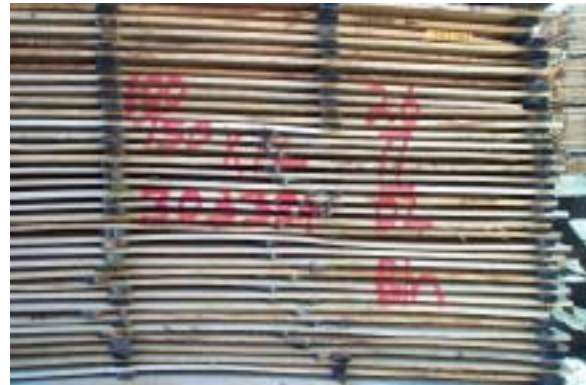
Figure7.28. Undesirable: Poorly aligned rack sticks
