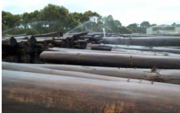
Figure 3.15. Sprinklers covering the logs well
