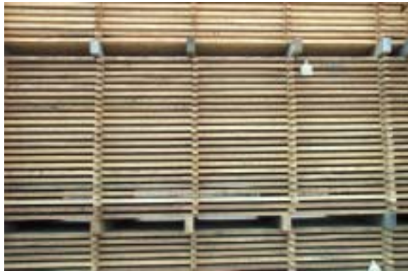
Figure7.27. Desirable: Neatly aligned rack sticks
