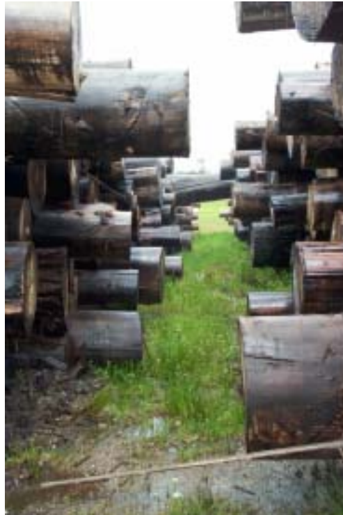
Figure 3.02. The combination of closely spaced log stacks and water from sprinklers reduces airflow, increases humidity and lowers temperature
