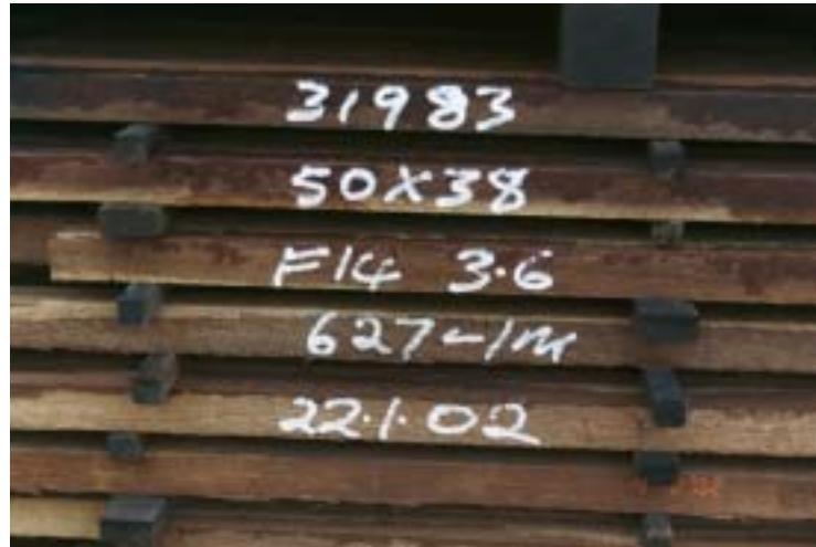
Figure7.20. Rack identification details; rack number, board size, timber grade, length, tally and assembly date
