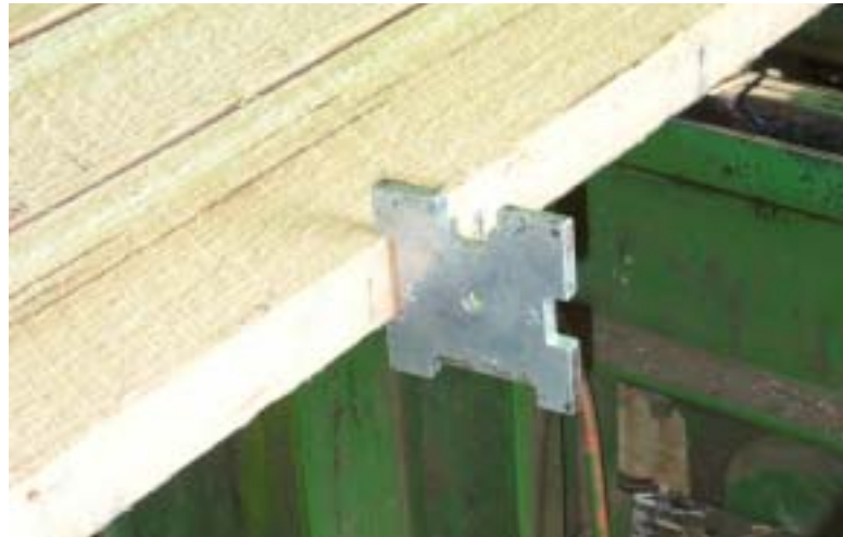
Figure 4.14. The thickness of boards must be checked regularly
