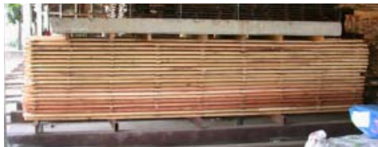
Figure7.10. A well constructed rack
