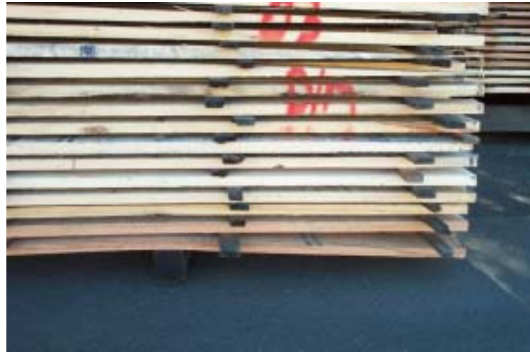
Figure 7.39. Bearer poorly placed
