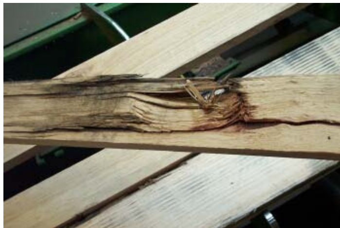
Figure 3.18. Mechanical damage to the log from a coupe or log yard visible in boards
