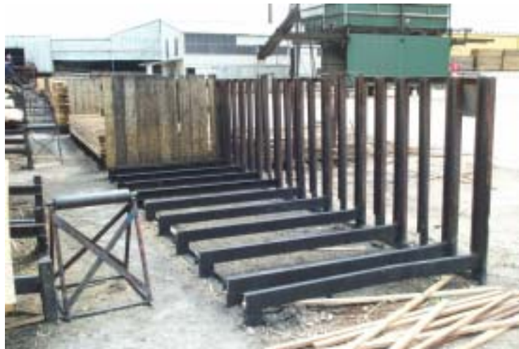
Figure 7.14. Fixed racking frame with stick guides on one side. The central section lifts out so forklifts can remove the completed racks
