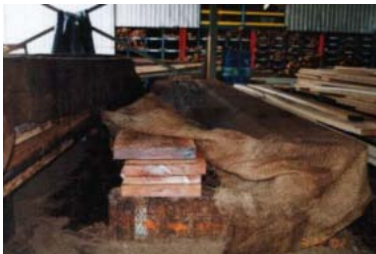
Figure 4.15. Protected Boards stacked under shelter
