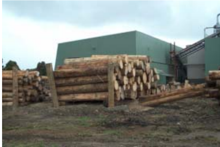
Figure 3.07. Log storage stacks on log bearers and against piled restraints
