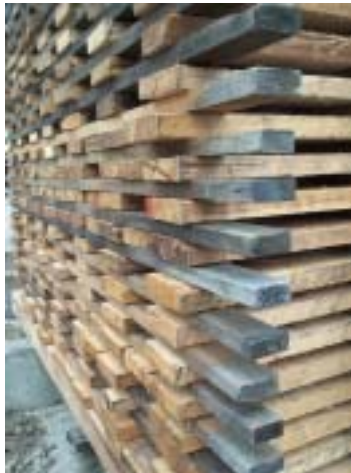
Figure7.29. Desirable: Neat rack end
