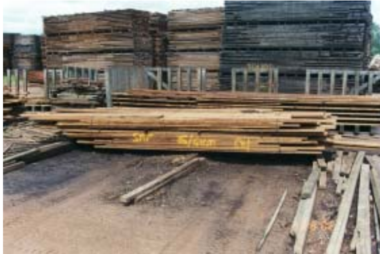
Figure 6.04 Packs in the sun can be damaged
