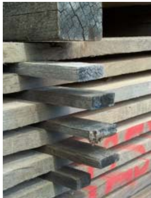
Figure7.44. Uneven rack stick thickness leads to board wave and uneven drying
