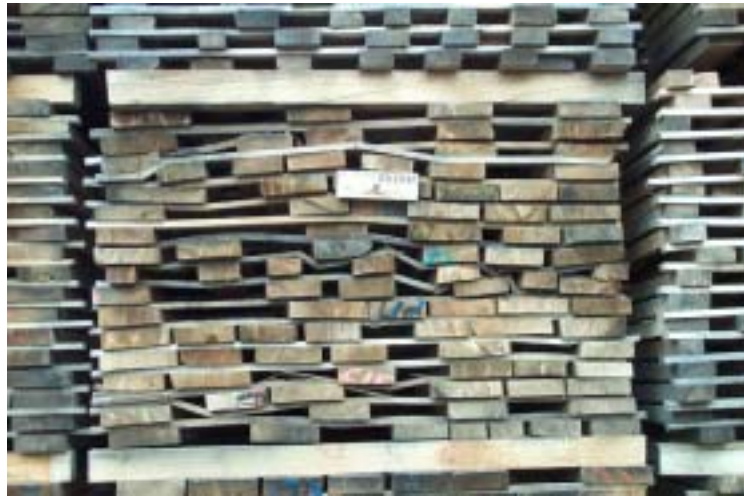
Figure 7.23. The results of poor racking practice
