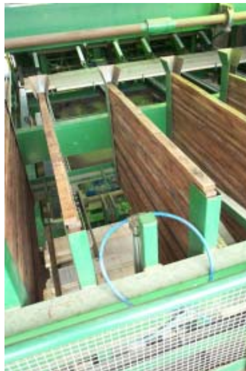
Figure 7.19. Rack sticks in a racking machine cartridge
