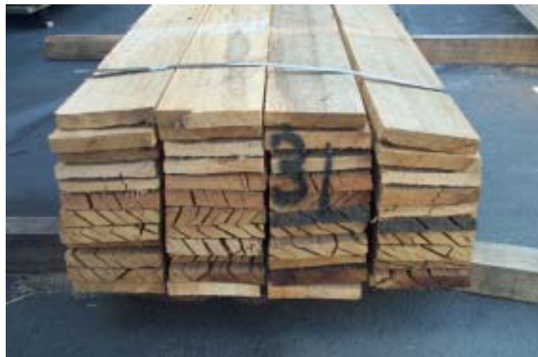
Figure 5.09. End checking from exposure during transport
