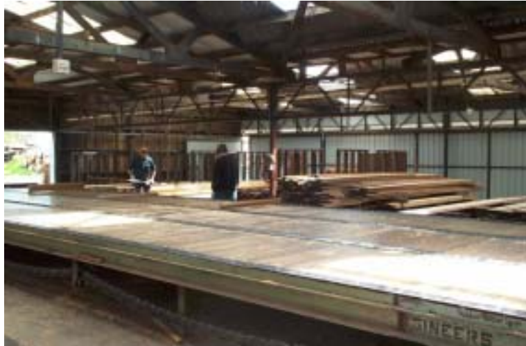
Figure 4.05. A fully enclosed linear green chain grading table. The racking and stacking positions are protected from the weather
