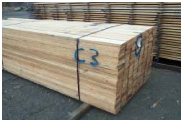
Figure 5.11. Desirable: Neat sides and ends
