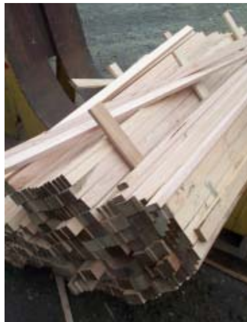
Figure 7.03 New dry and thickened rack sticks
