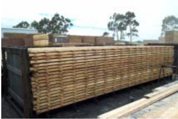
Figure 7.34. Desirable: Neat edges to the rack
