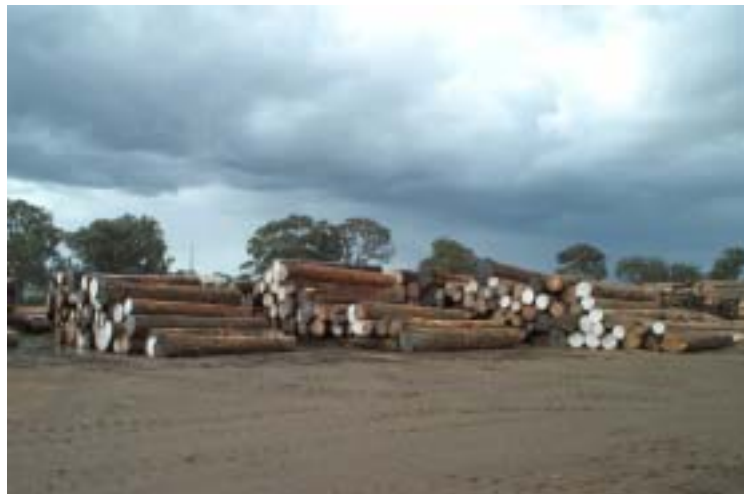
Figure 3.03. Logs batched by species, size and length into temporary stacks before milling. All new exposed log ends are sealed
