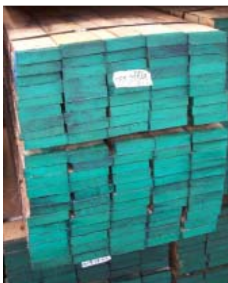
Figure 5.10. Pack number on end coated packs
