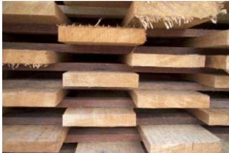
Figure7.09. The checkerboard pattern of top and tail boards
