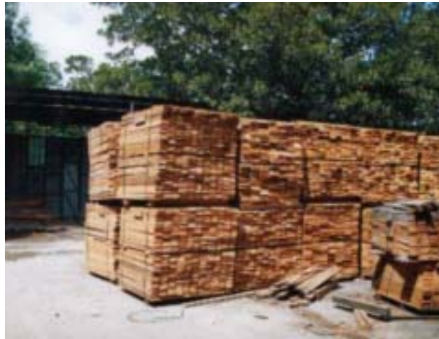
Figure 5.16. Packs exposed to the sun can be damaged
