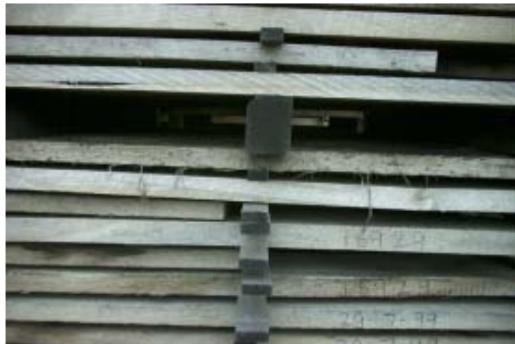
Figure7.46. Uneven support of boards during racking leads to twisted and deformed boards, and unstable stacks
