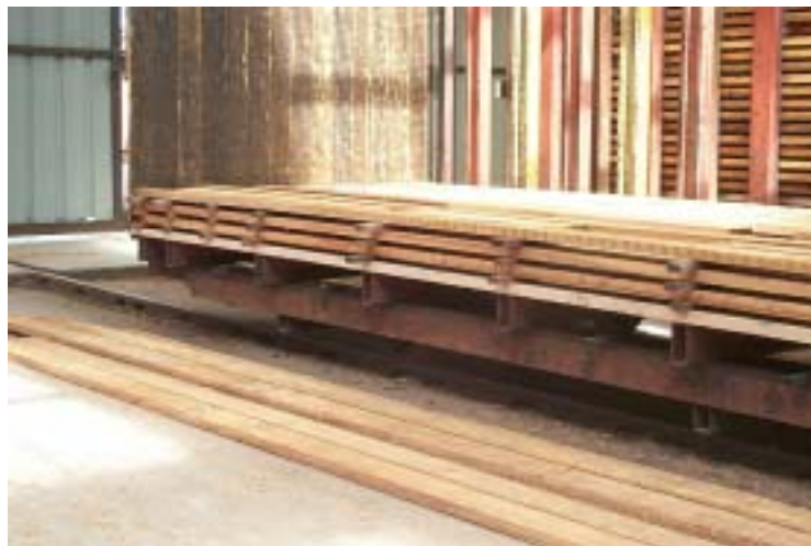
Figure7.33. Long boards are saved for the sides and base of a hand assembled rack
