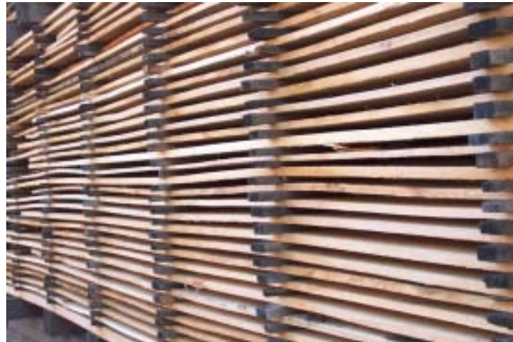
Figure 7.02 Inadequate rack stick spacing
