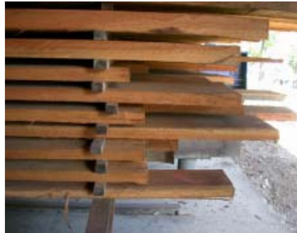
Figure7.30. Undesirable: Uneven rack end
