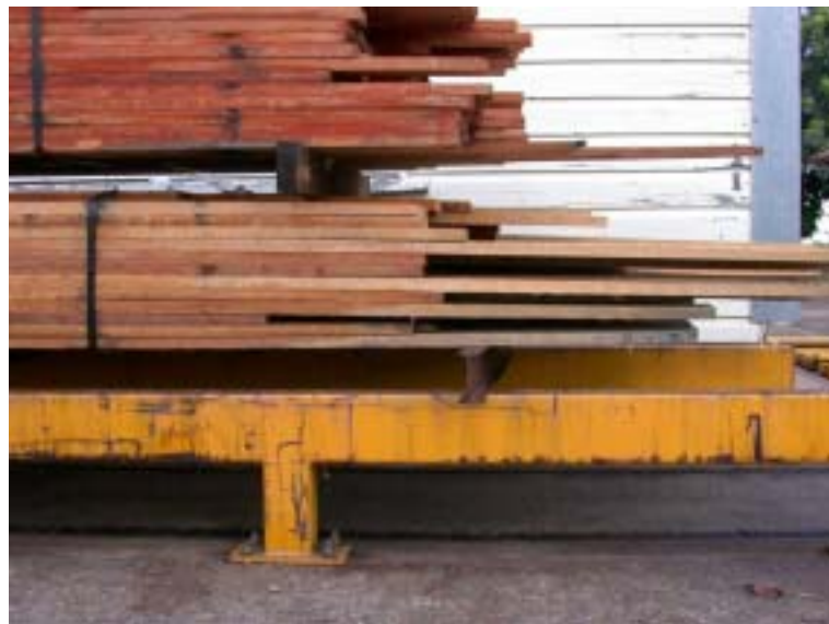
Figure 5.15. Unevenly built packs with unsupported board ends
