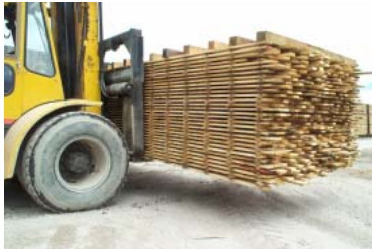
Figure 7.42. Racks have to be transported carefully to minimise loss and movement of rack sticks
