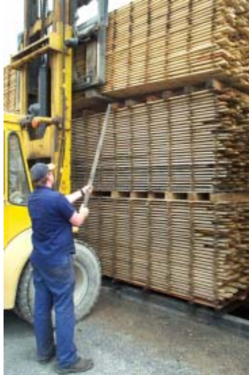
Figure7.13. Even when stacked for temporary storage, bearers and gluts should be aligned with rack sticks
