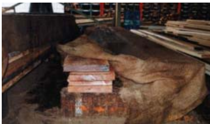
Figure 4.04. High value boards in an aggressive climate stacked under local environmental protection
