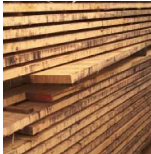
Figure7.49. Boards displaced during transportation dry irregularly and are often discarded
