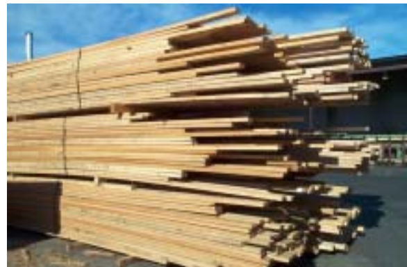
Figure 5.12. Undesirable: Uneven sides and ends
