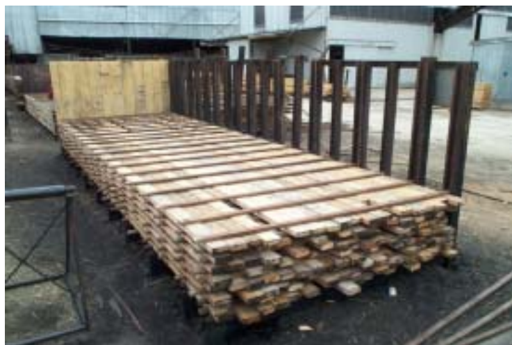
Figure7.26 Racking frame with neat rack stick placement
