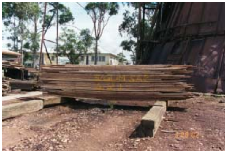
Figure 5.18. Boards in packs of different lengths, supported unevenly and stacked in the sun dry unevenly and deform
