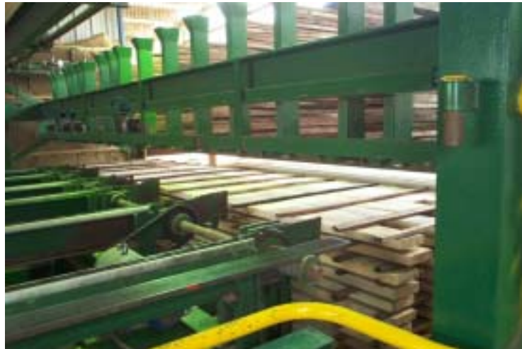
Figure 7.18. Timber being placed by a racking machine
