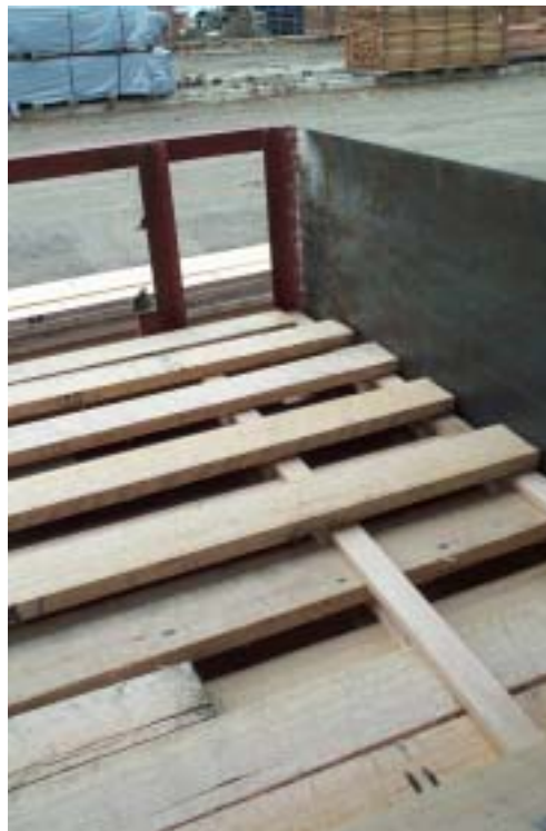
Figure 7.36. Boards in a rack topped and tailed
