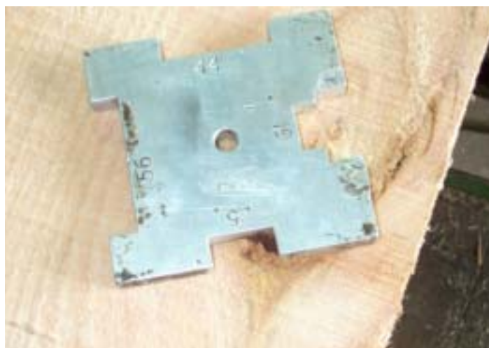
Figure 4.10. A thickness gauge used to check sawing accuracy
