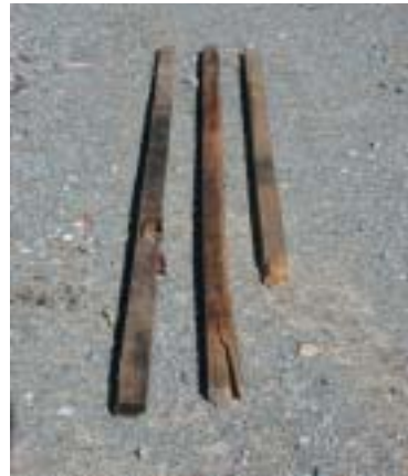
Figure7.32. Rack sticks in poor condition discarded
