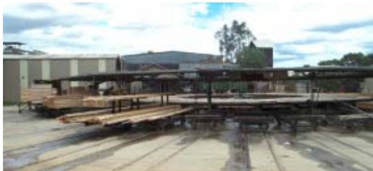
Figure 4.07. A covered circular green grading chain. The racking and stacking positions are exposed to the weather
