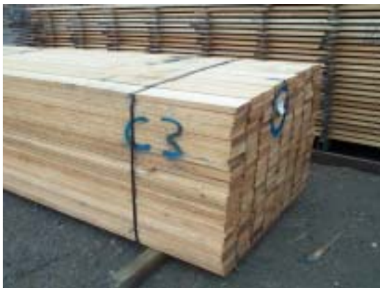
Figure 5.02. Desirable: Pack with even ends
