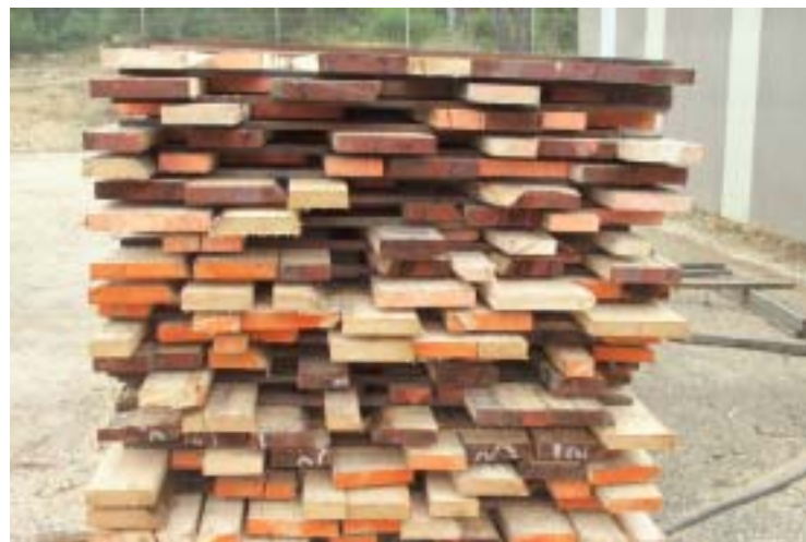
Figure 7.48. Uneven sides and board spacing leads to irregular airflow and uneven drying
