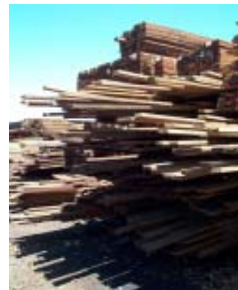
Figure 5.03. Undesirable: Pack with uneven ends
