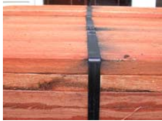
Figure 5.07. Undesirable: Corners crushed by pack straps
