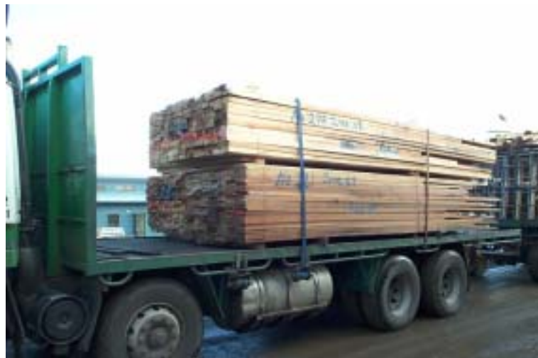
Figure 5.17. Packs on open trucks can be damaged
