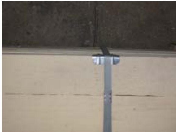
Figure 5.13. Desirable: Corner protectors
