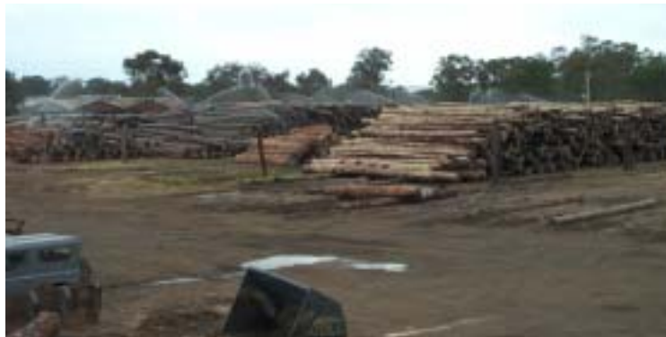
Figure 3.06. A large log storage yard with storage stacks, gravel roading, water sprays and drainage systems
