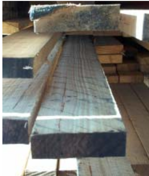
Figure 5.04. Collapse in exposed ends in packs
