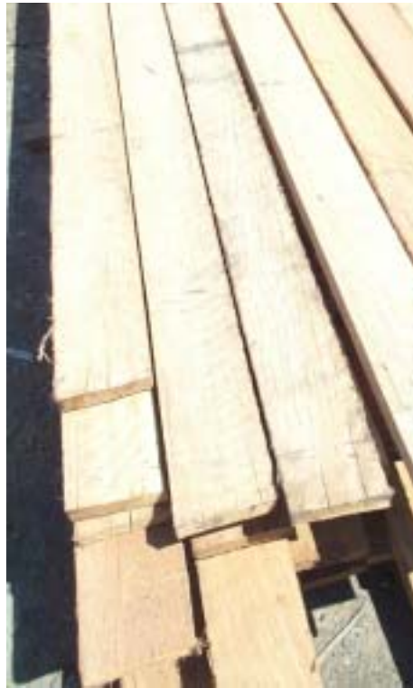
Figure 5.19. Drying checks in the exposed ends and surfaces of boards left in the sun
