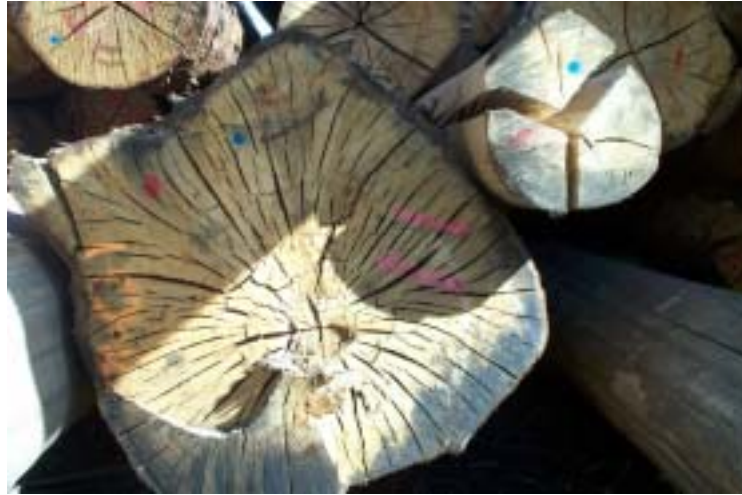
Figure 3.17. Exposing logs to wind and sun for an unnecessarily long period of time can cause severe end and barrel checking
