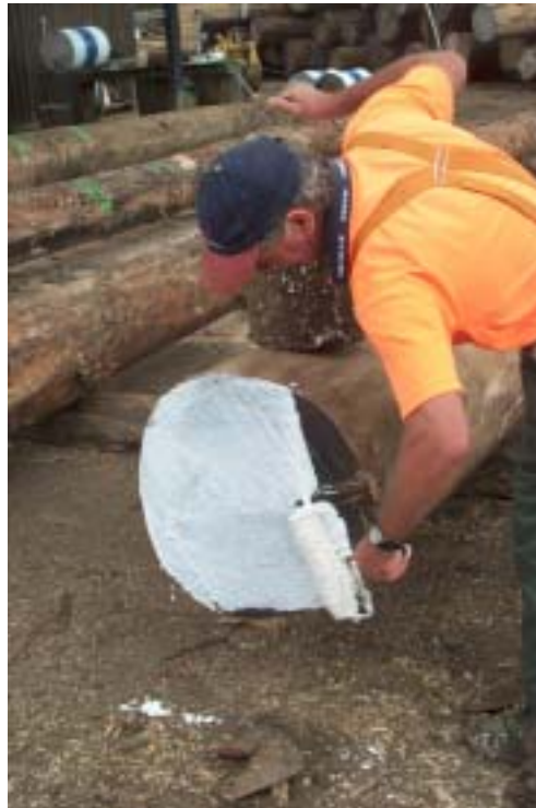
Figure 3.14. All cut ends of logs are resealed immediately
