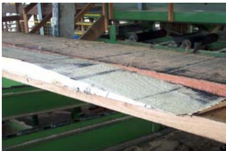
Figure 4.03. Uneven board run off
