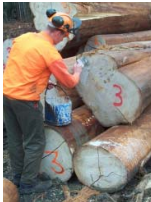
Figure 2.08. All cut ends of logs are resealed immediately
