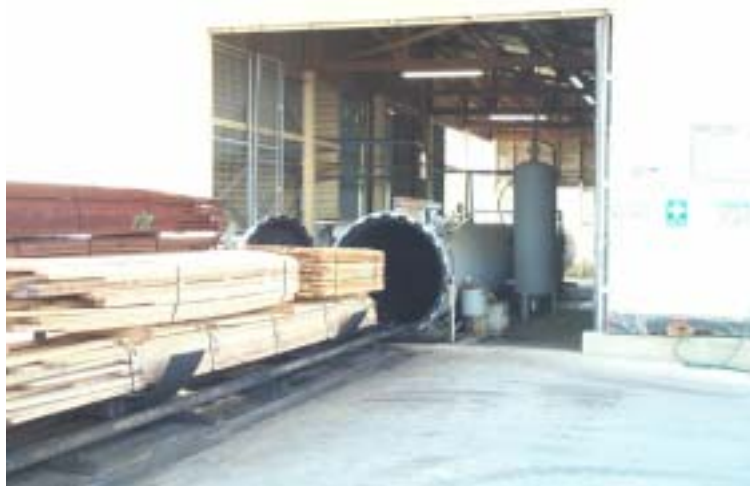
Figure 6.02 Chemical treatment pressure cylinder
