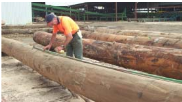
Figure 3.16. Measure the logs with a gauge
