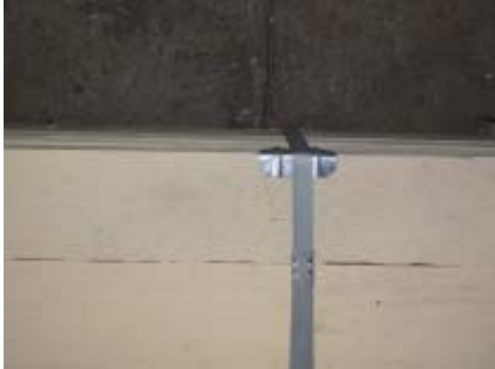
Figure 5.06. Desirable: Corners protected from pack straps
