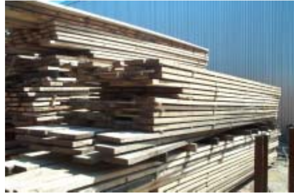
Figure 7.35. Undesirable: Uneven edges to a rack
