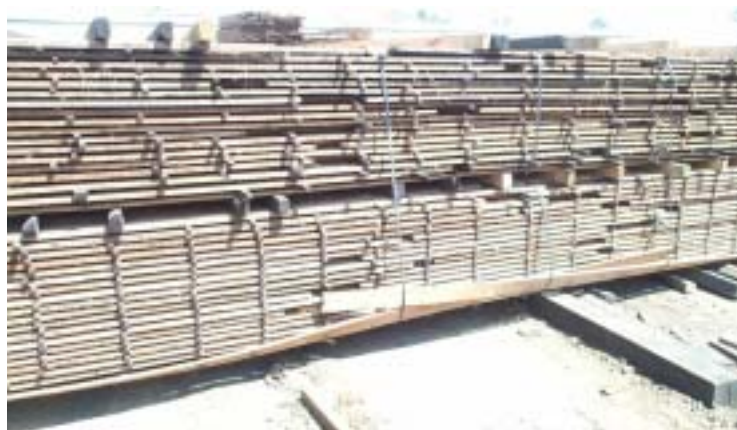
Figure7.50. Boards displaced during transportation are often damaged
