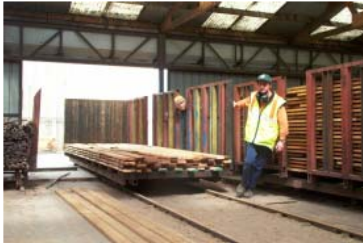
Figure 7.15. Mobile racking frame. Mounted on wheels and rails, the frame is moved outside the building for unloading
