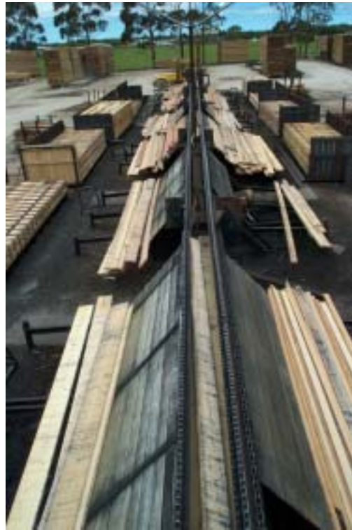
Figure 4.08. A mechanical line sorter. Boards of the same grade and dimension are distributed to racking or stacking positions along sets of chains. The racking staff and boards are exposed to the weather
