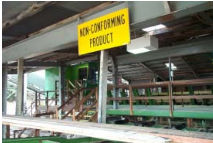
Figure 7 25 Segregate non-conforming product
