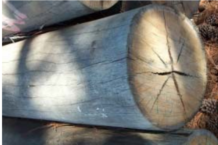
Figure 2.02. End and barrel checking of unprotected logs
