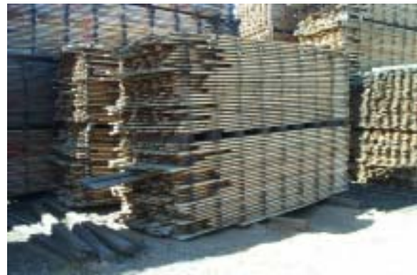
Figure 7.41. Undesirable: Bearers out of line
