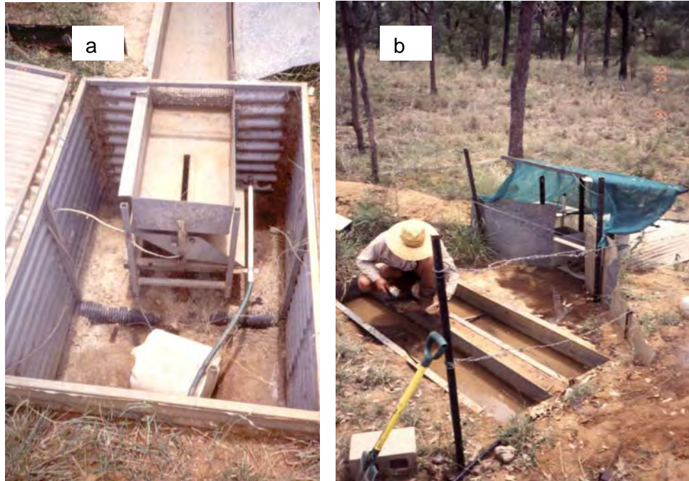
Figure 9.3 (a) Gerlach trough, tipping bucket and suspended sediment sampling equipment for plots, and (b) bed load sediment sampling trough upslope of a flume for a mini-catchment.
