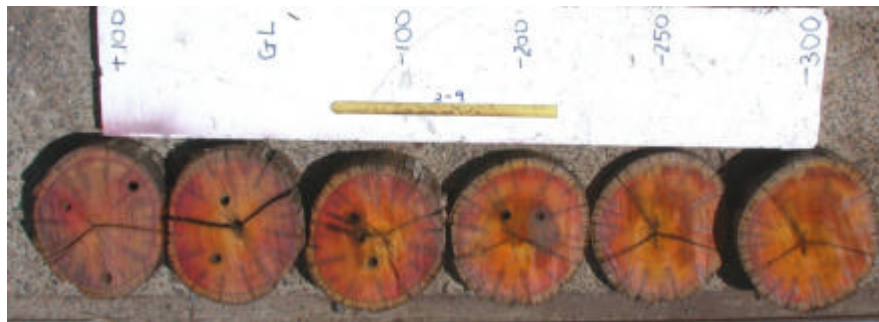
Figure 44 Boron penetration in a DC 1 pole
