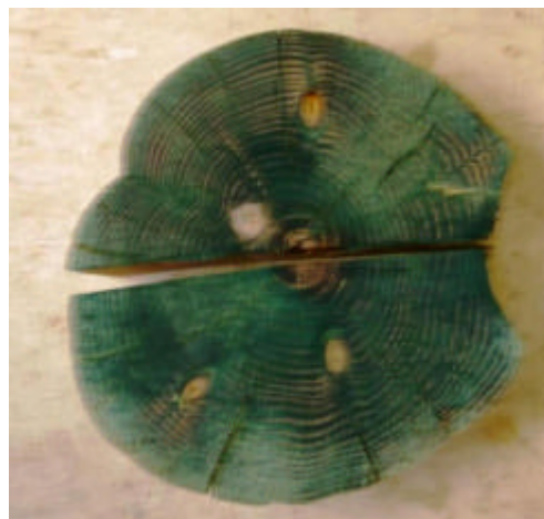
Figure 14 Penetration of CCA preservative near ground-line in a P. radiata pole
