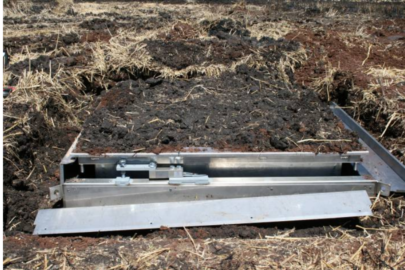
Figure 44. Lysimeter during field installation showing removed load cell covers.
