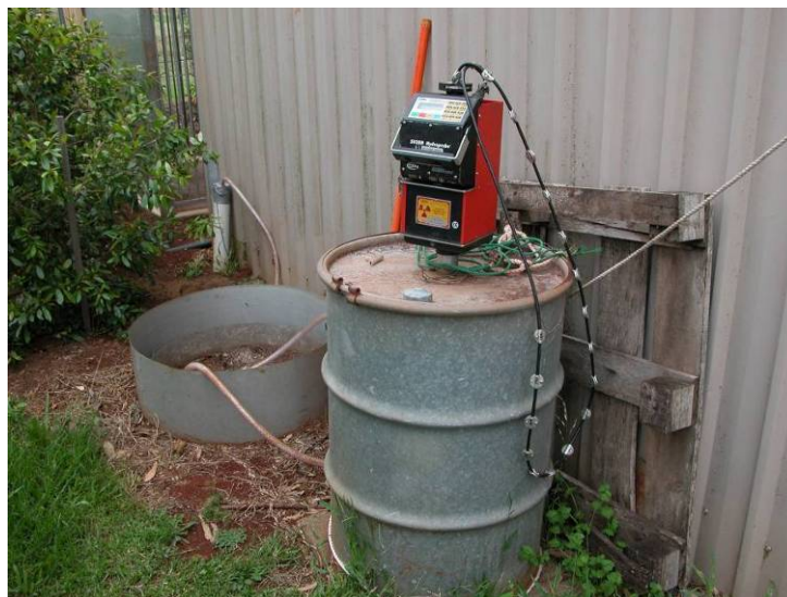
Figure 6. Taking neutron probe water standard count reading.
