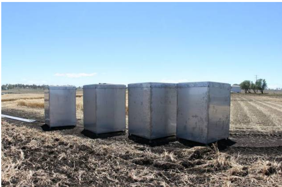
Figure 46. Lysimeters at Kingsthorpe prior to installation (12 Nov 2008).
