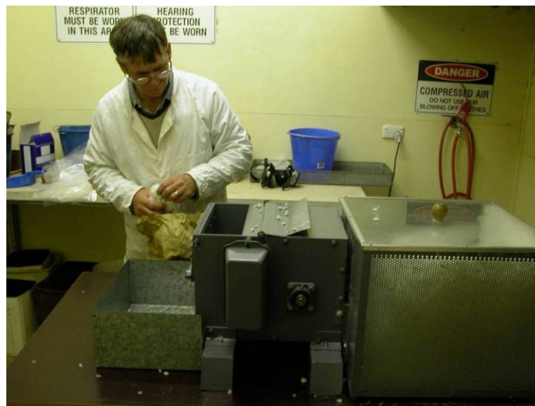
Figure 10. Ginning cotton using a laboratory ginning machine.
