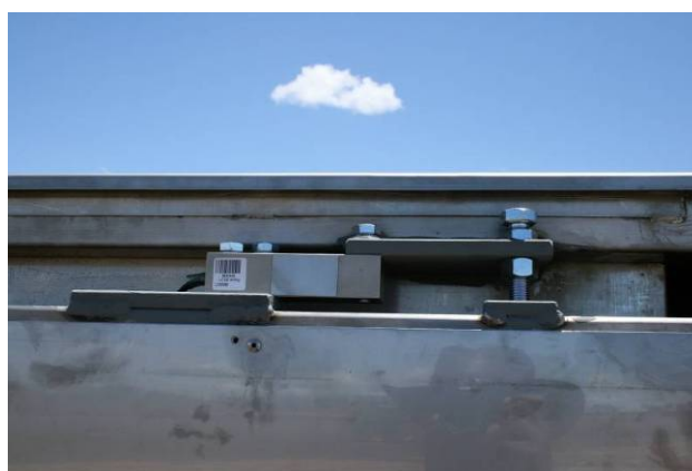
Figure 43. Detail of load cell mount.
