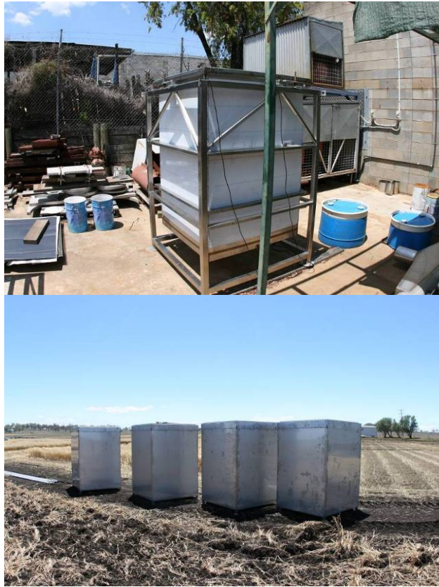
Figure 2. Lysimeter design 2 , constructed of stainless steel and the total mass of the inner lysimeter box rests directly on the load cells.
